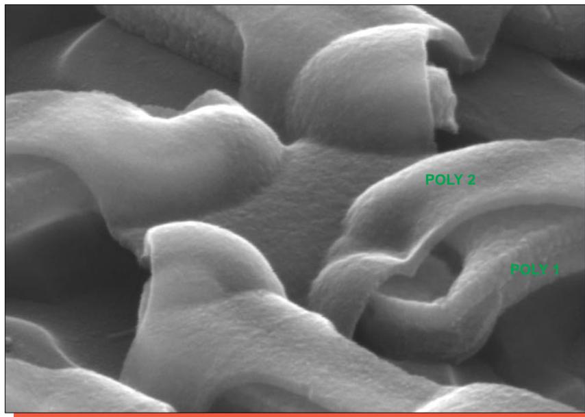
Figure 29. Detailed SEM views of the SRAM cell structures (delayed).
