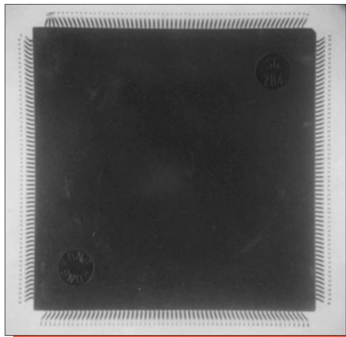
Figure 1. Package photographs of the Analog Devices ADSP-21062-KS-160 SHARC Digital Signal Processor. Mag. 2.5x.
