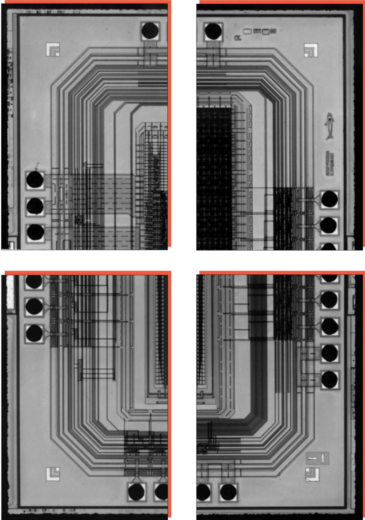
Figure 5. Optical views of die corners. Mag. 80x.
