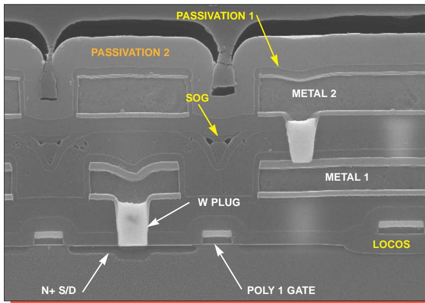
Figure 8. SEM section views illustrating general structure. Mag. 13,000x.
