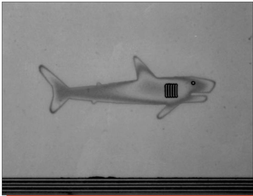
Figure 4. Optical views of die markings. Mag. 500x.
