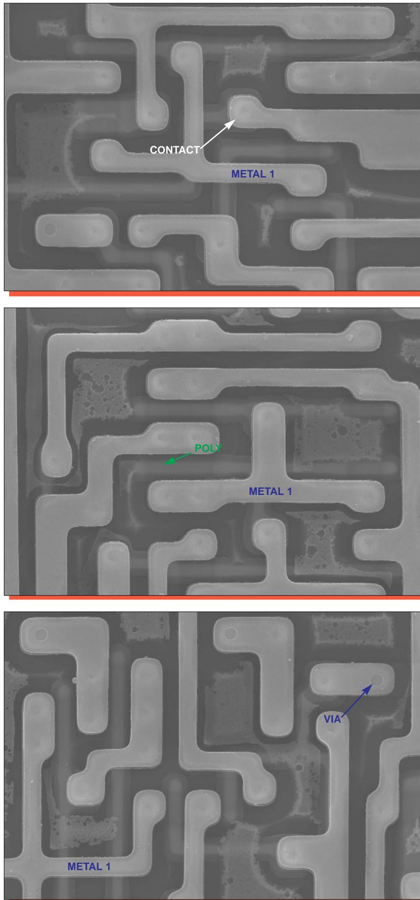
Figure 15. Topological SEM views of metal 1 patterning. Mag. 6500x, 0°.
