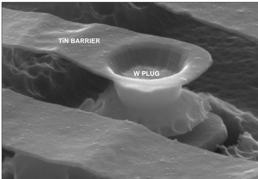
Figure 12. Perspective SEM views of metal 2 step coverage, barrier, and plug. 60°.
