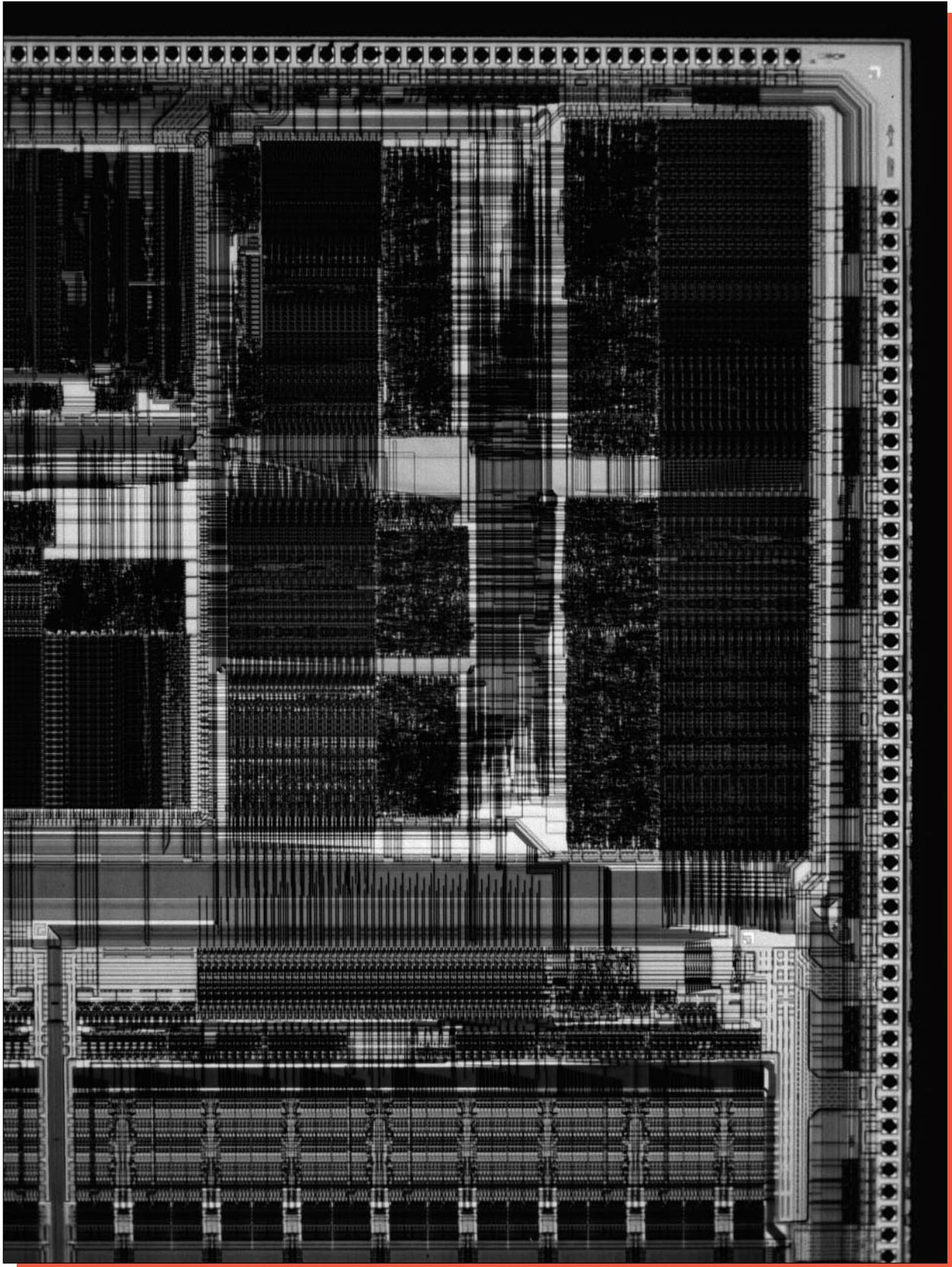
Figure 3a. Portion of the Analog Devices ADSP-21062-KS-160 die. Mag. 26x.
