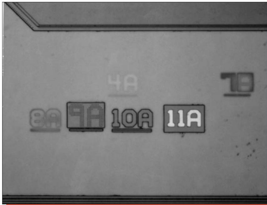
Figure 6. Optical views illustrating a slotted bus line and mask revision numbers.
