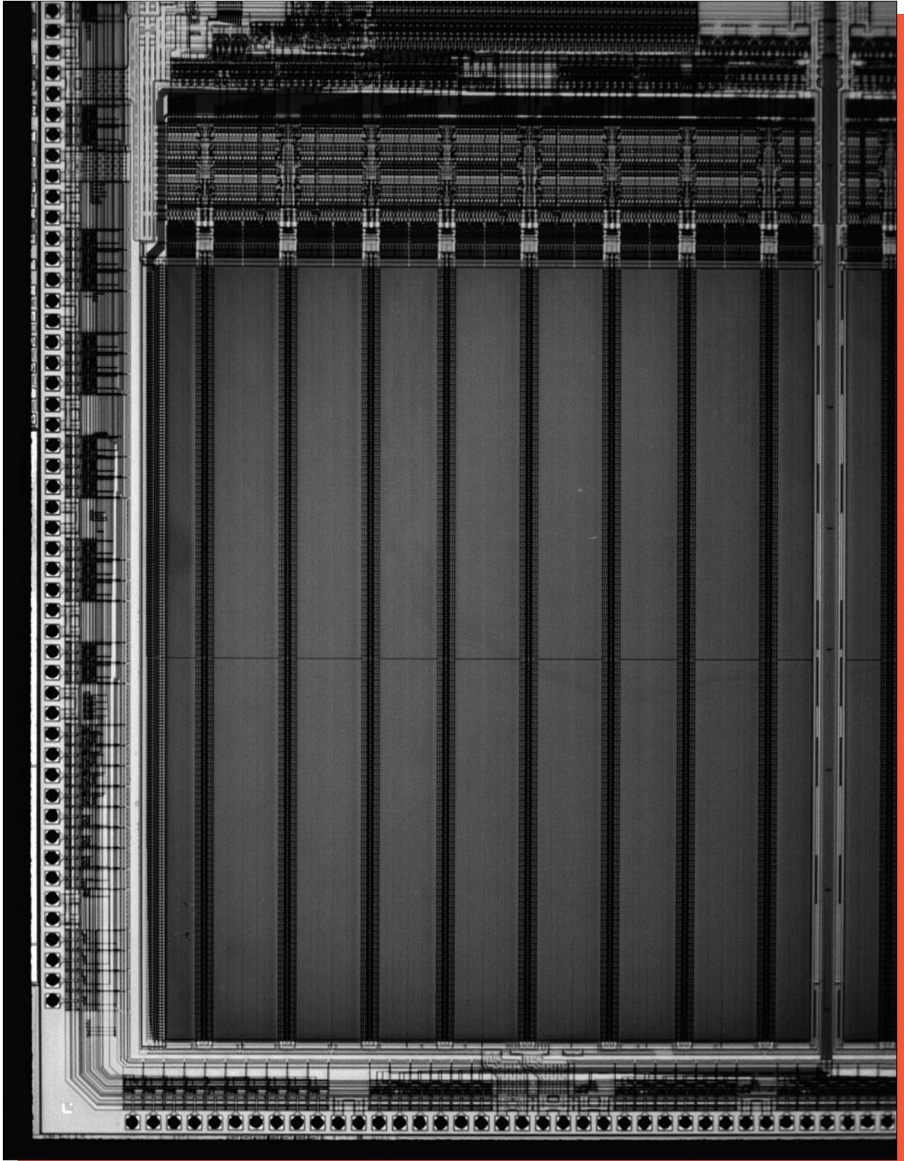
Figure 3b. Portion of the Analog Devices ADSP-21062-KS-160 die. Mag. 26x.
