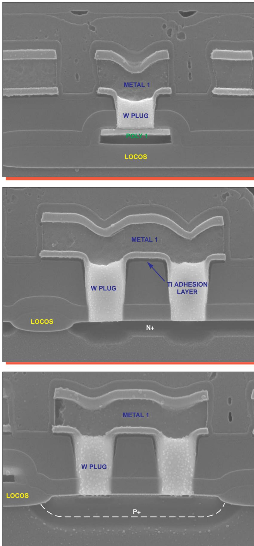
Figure 18. SEM section views illustrating typical metal 1 contacts. Mag. 26,000x.
