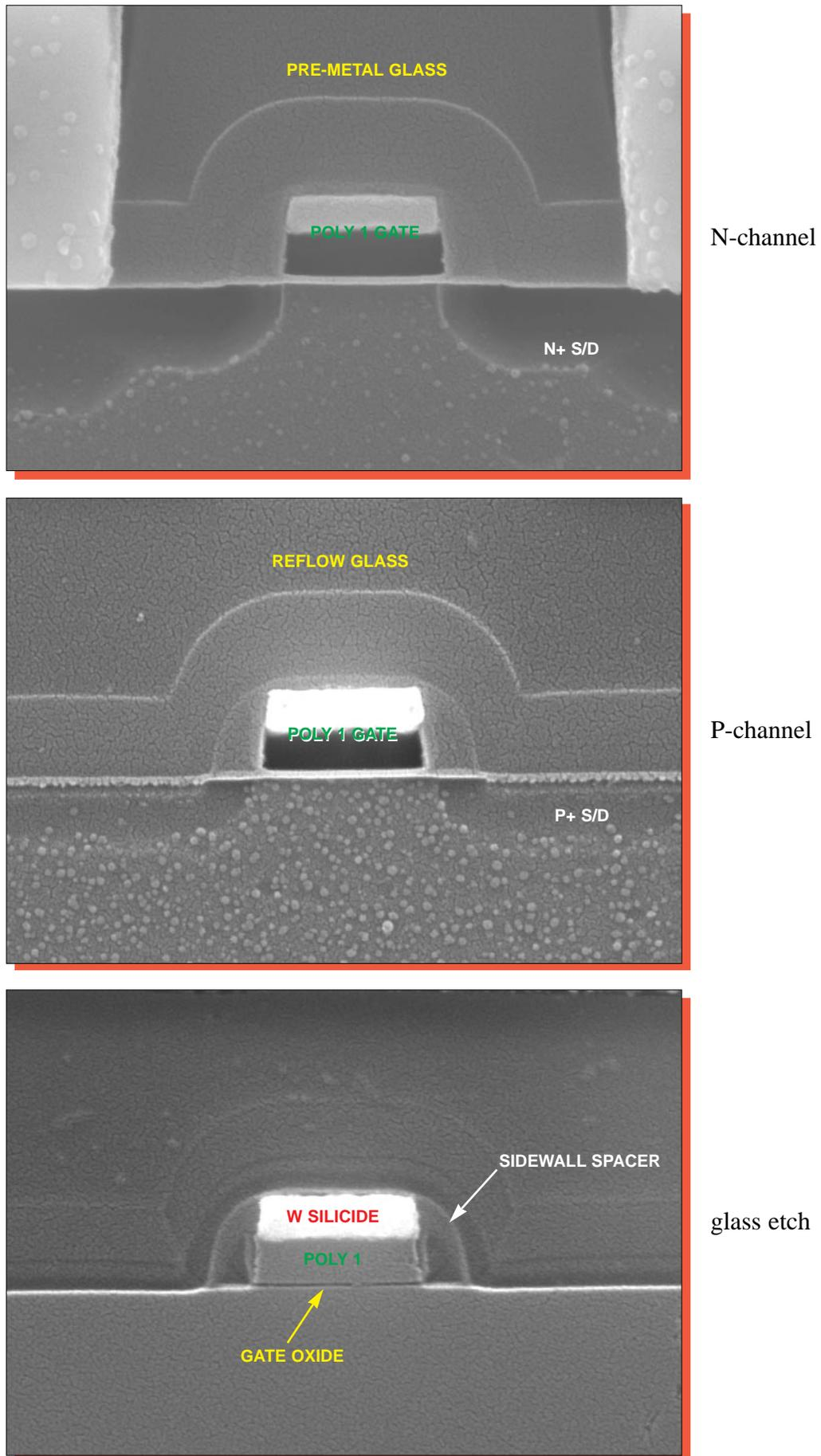
Figure 21. SEM section views of typical transistors. Mag. 52,000x.
