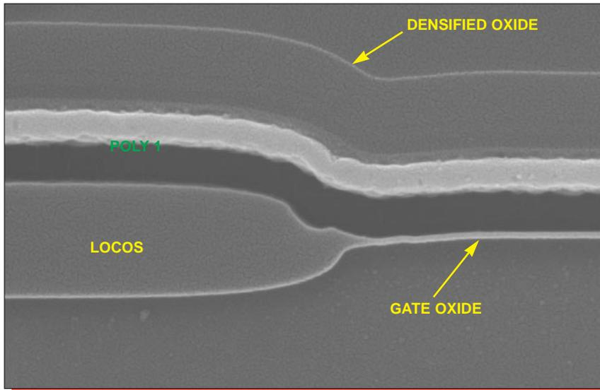
Figure 22. SEM section view of typical birdsbeak. Mag. 52,000x.
