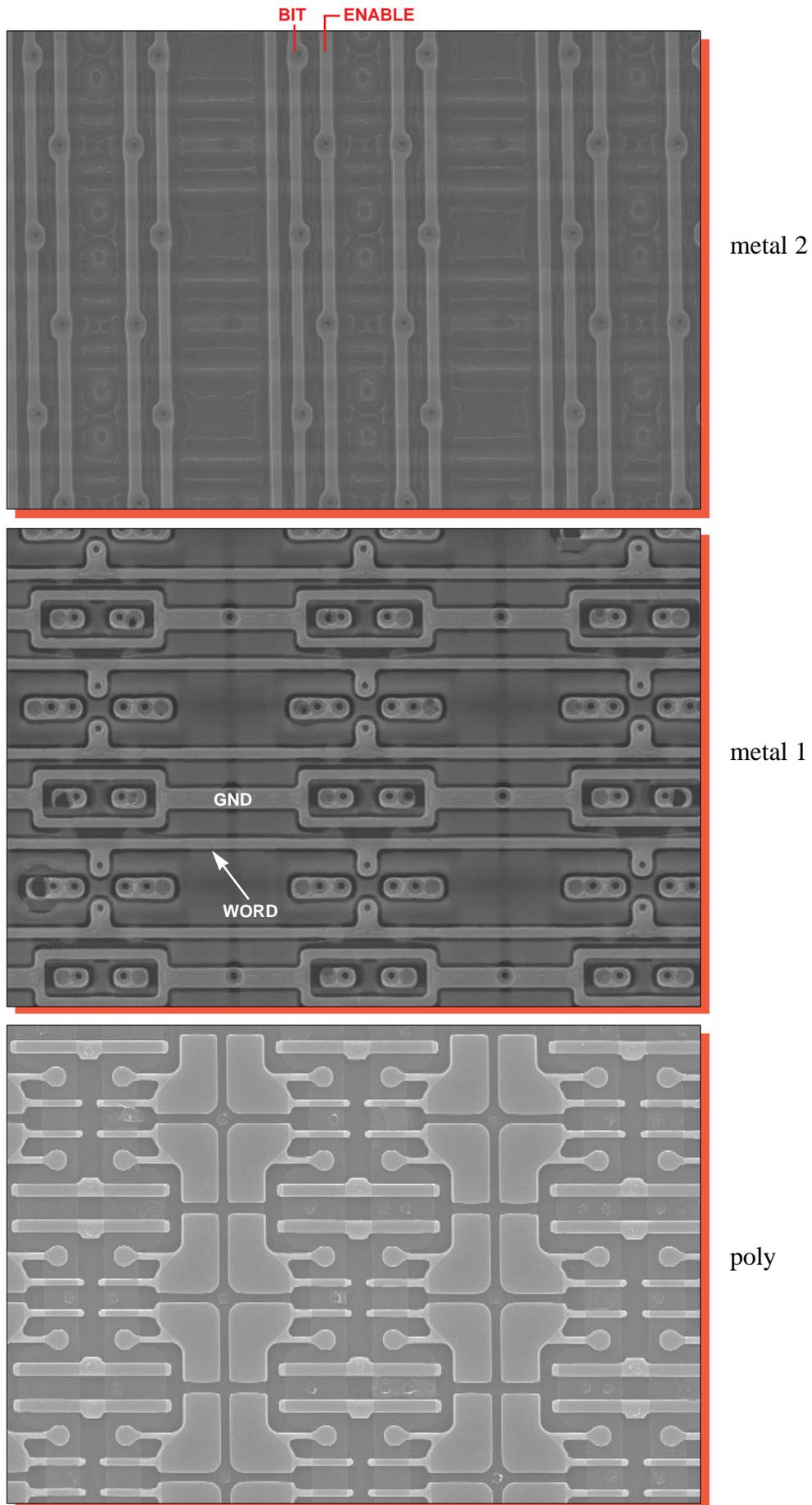
Figure 15. Topological SEM views of the EEPROM cell. Mag. 1625x, 0°.
