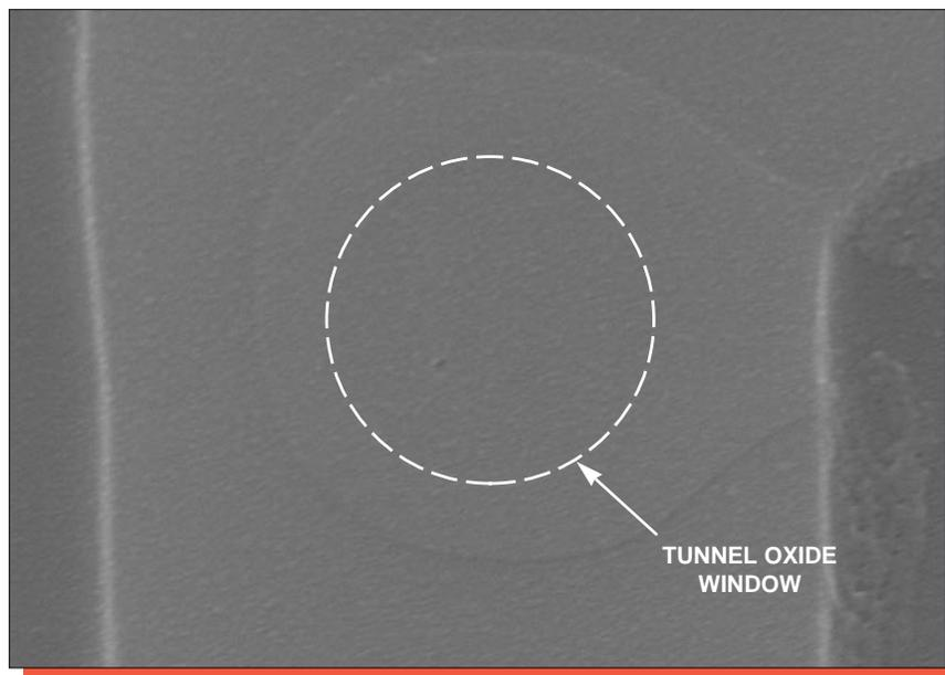
Figure 18. Topological SEM view of the tunnel oxide window. Mag. 26,000x, 0°.
