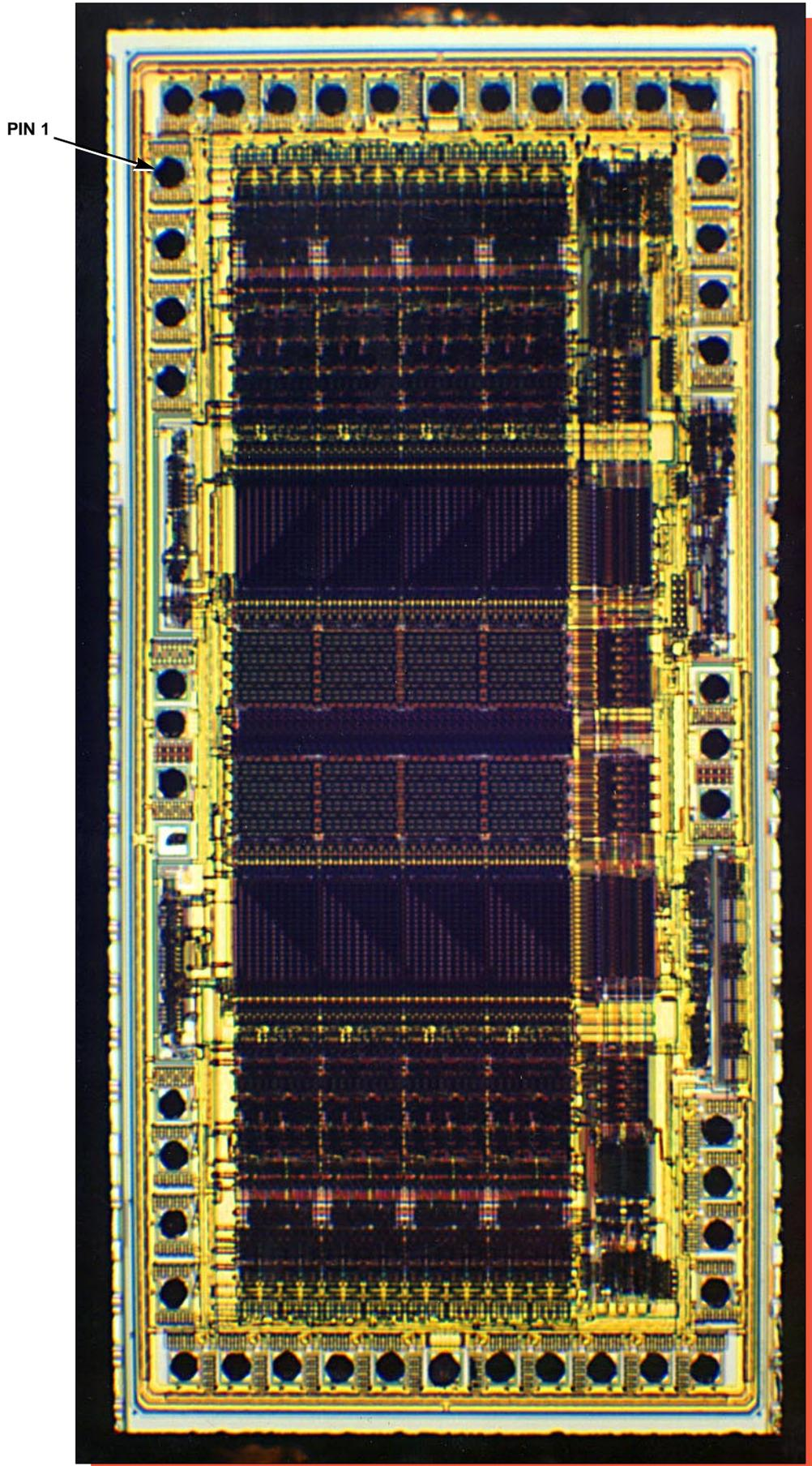
Figure 1. Whole die photograph of the Lattice ispLSI 2032-180L CPLD. Mag. 50x.
