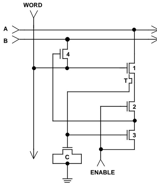
Figure 25. Topological view and schematic of an additional EEPROM cell.
