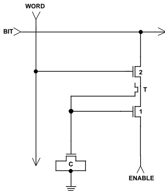
Figure 17. Topological view and schematic of the EEPROM cell. Mag. 3250x, 0°.
