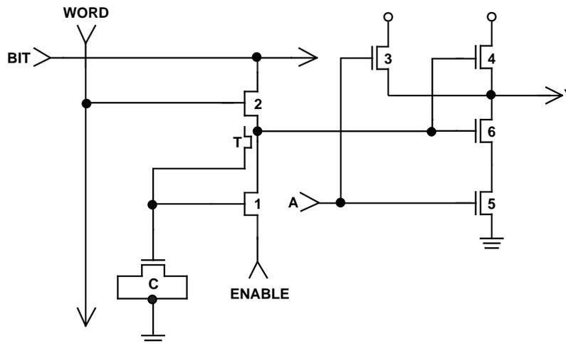
Figure 28. Topological view and schematic of an additional EEPROM cell.
