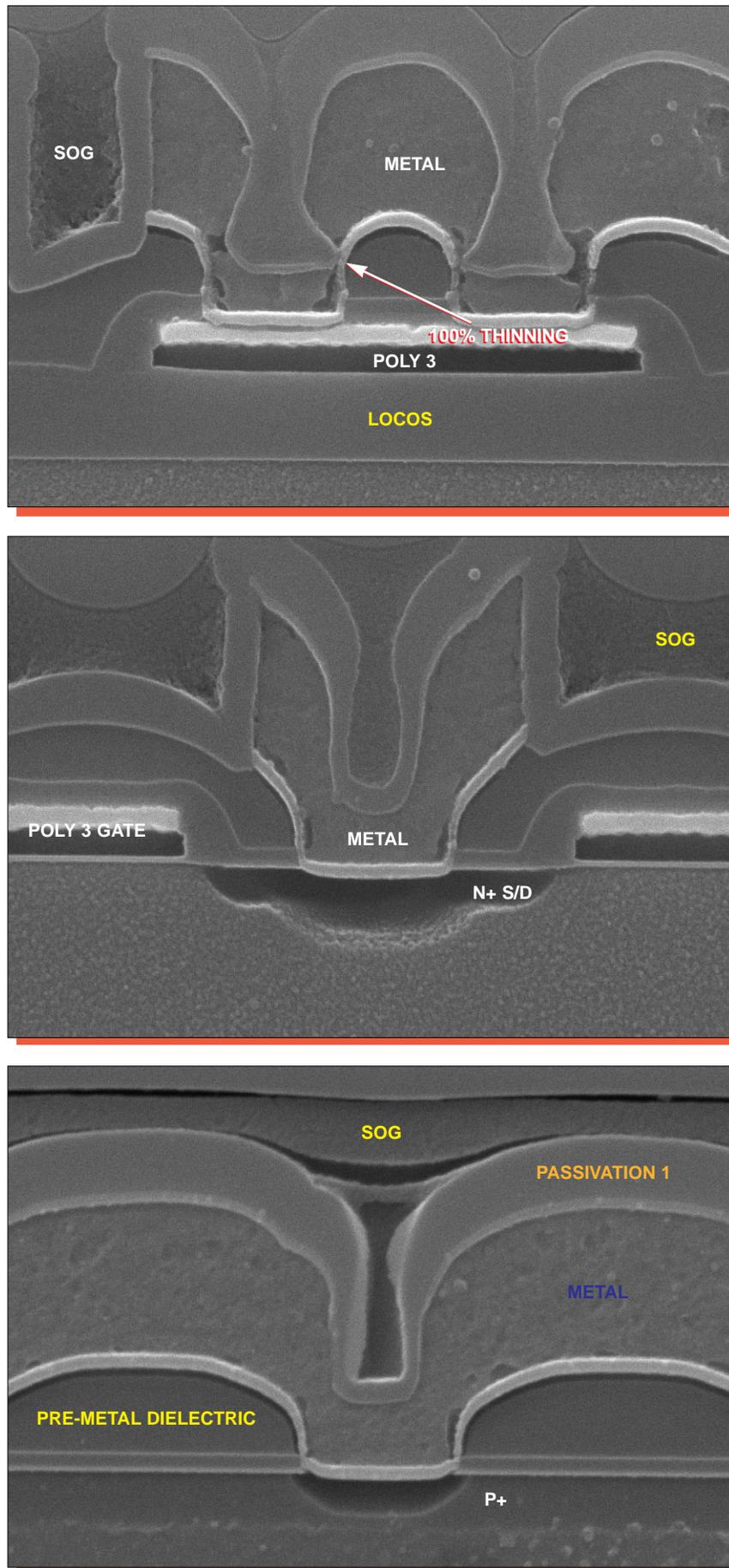
Figure 13. SEM section views of typical metal contacts. Mag. 26,000x.
