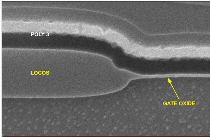
Figure 17. SEM section view of a typical birdsbeak. Mag. 52,000x.
