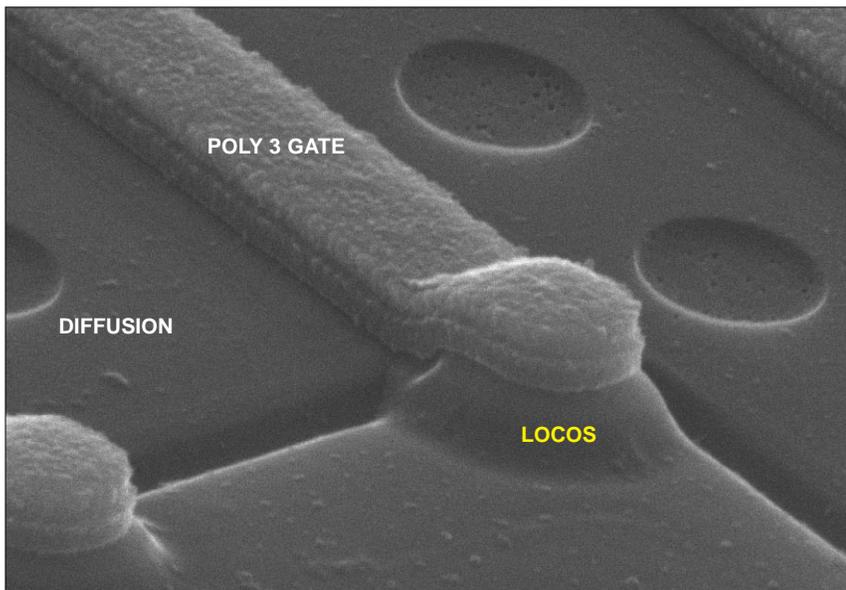
Figure 15. Perspective SEM views of poly 3 coverage. 60°.
