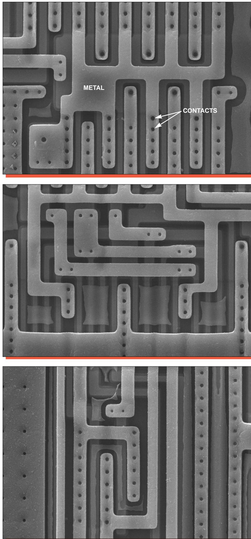
Figure 11. Topological SEM views of metal patterning. Mag. 3200x, 0°.
