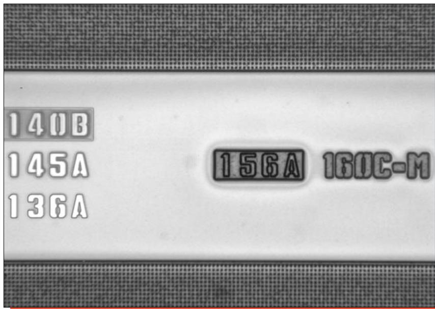
Figure 6. Optical views of die markings. Mag. 350x.
