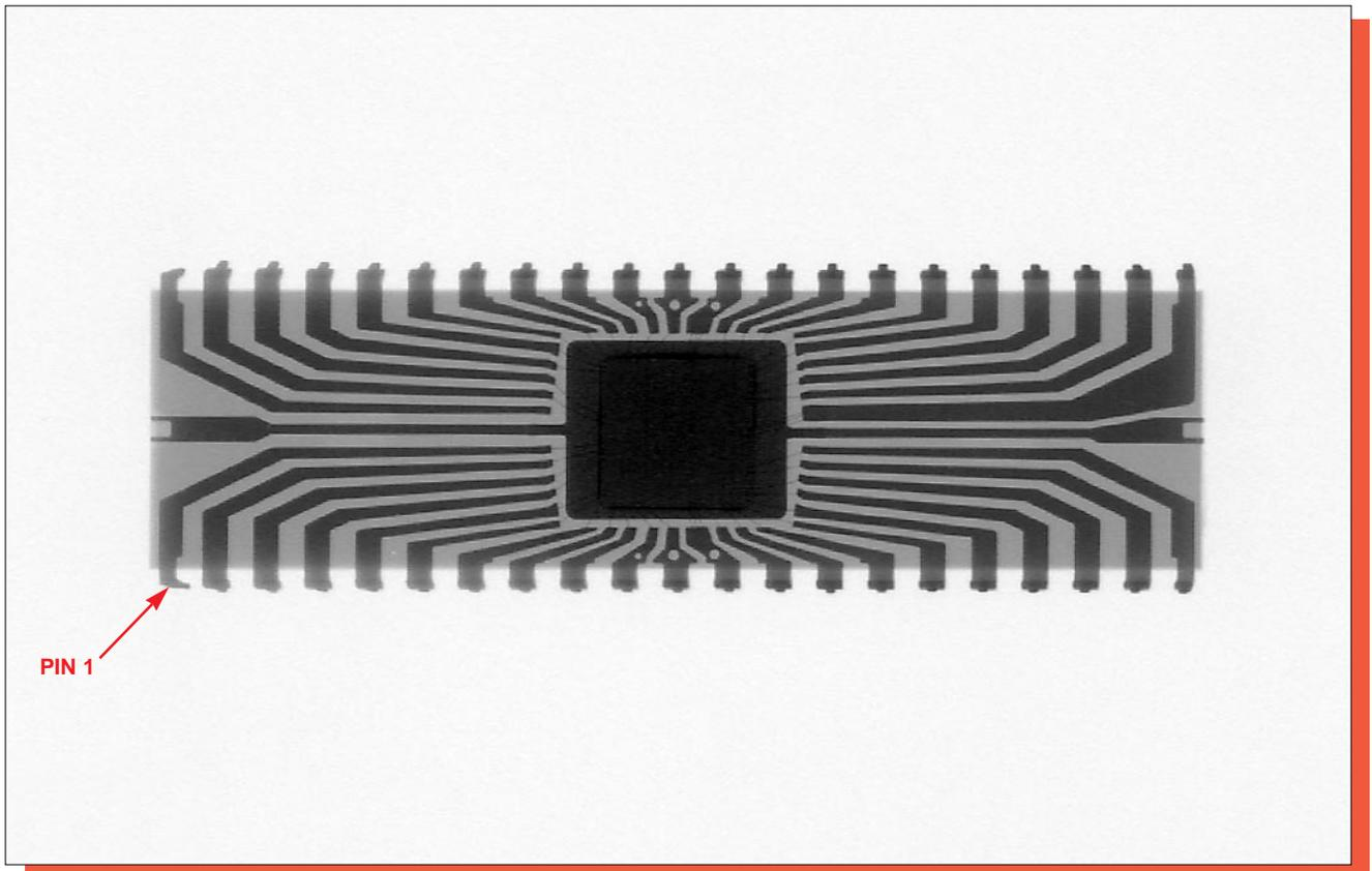
Figure 2. X-ray view of the package. Mag. 2.5x.
