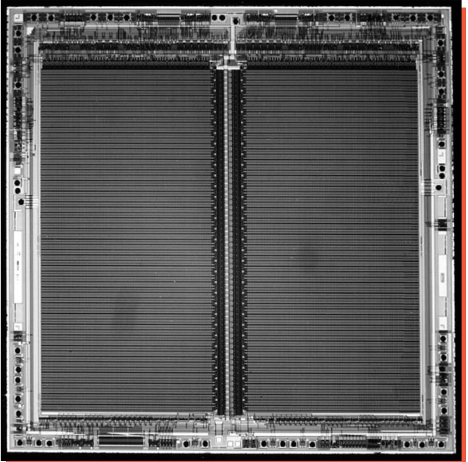
Figure 5. Whole die photograph of the Macronix 27C8100PC-10, 8Mb EPROM.
