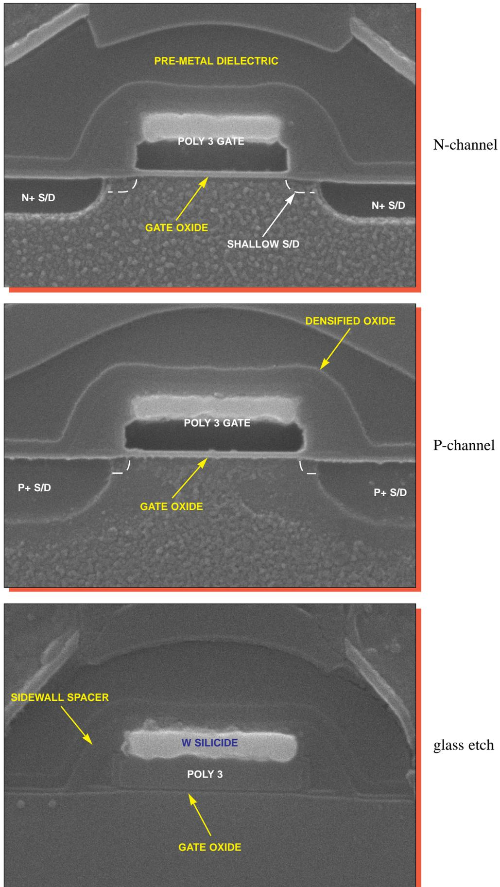
Figure 16. SEM section views of typical transistors. Mag. 52,000x.
