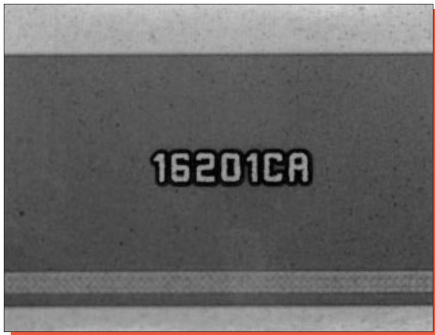
Figure 10. Identification marking from the die surface. Mag. 100x.
