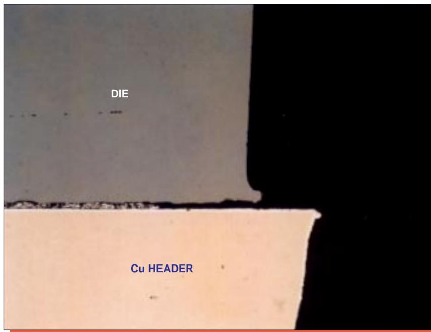
Figure 5a. Package section views illustrating die placement on header. Mag. 200x.
