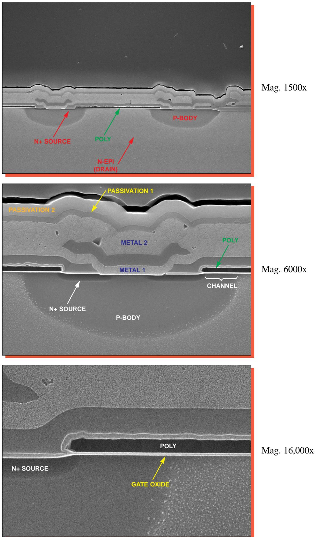
Figure 23. SEM section views of the DMOS Power HEXFET structure.
