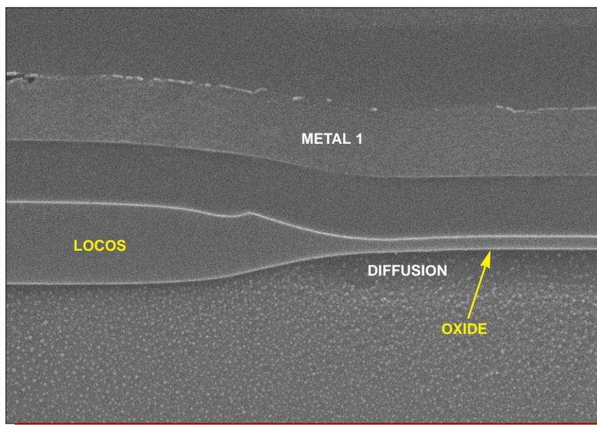
Figure 21. SEM section views of local oxide birdbeak profiles. Mag. 16,000x.
