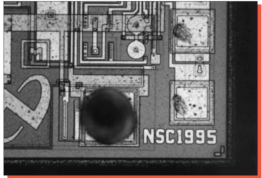
Figure 7. Optical views of the die corners on the National LM2672 device. Mag. 200x.
