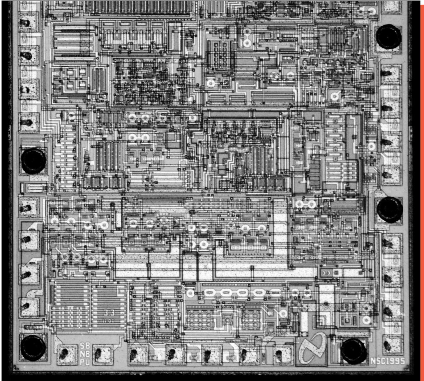
Figure 5b. Detailed optical view of the linear device area. Mag. 100x.
