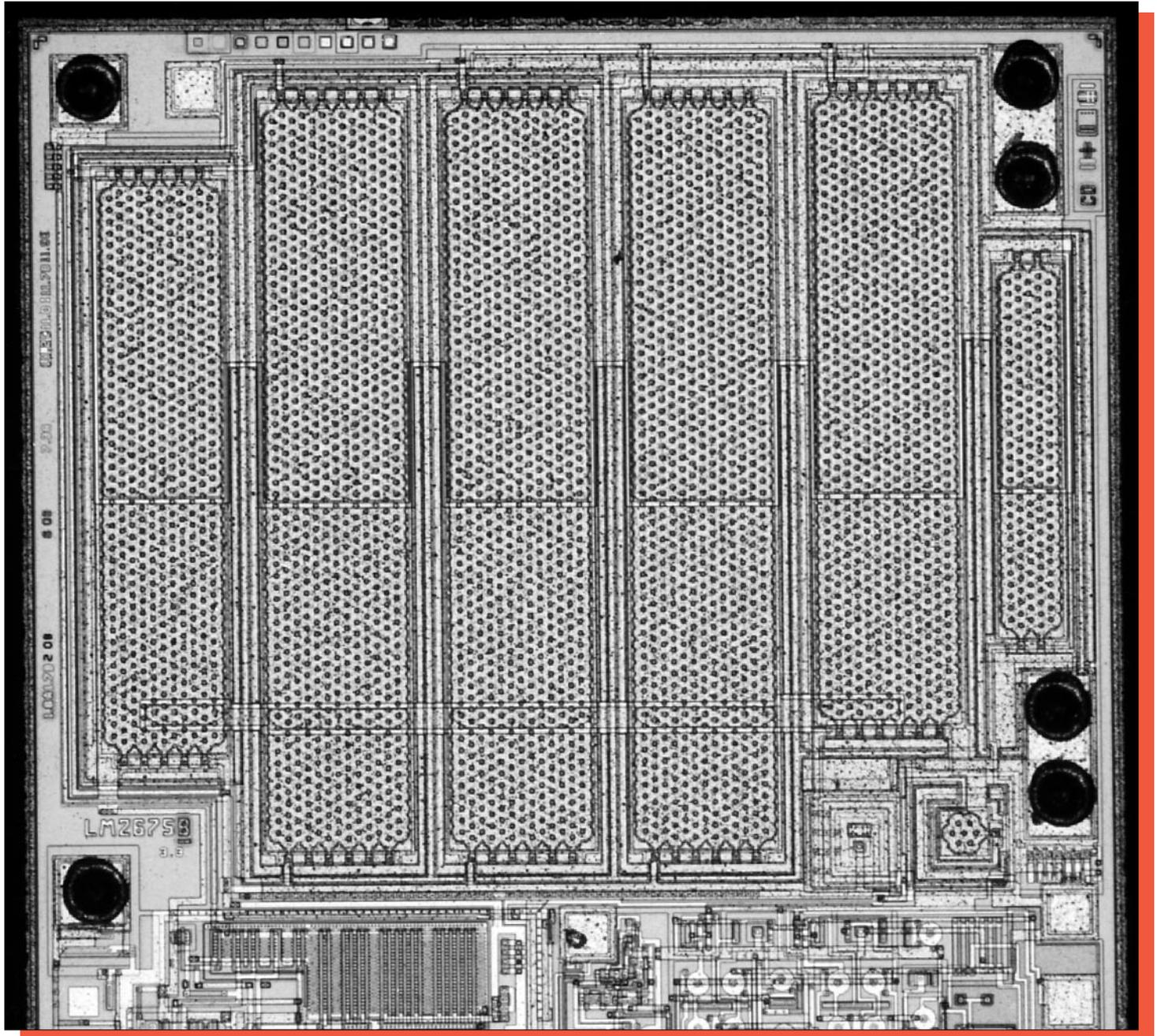
Figure 5a. Detailed optical view of the DMOS area. Mag. 100x.
