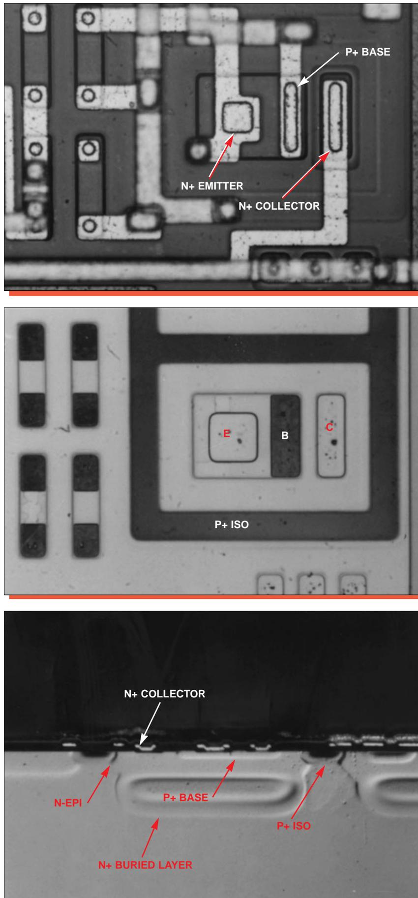
Figure 25. Optical views of an NPN transistor. Mag. 800x.
