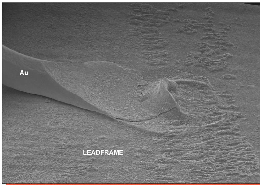
Figure 4. SEM views of typical wirebonds. Mag. 500x, 60°.
