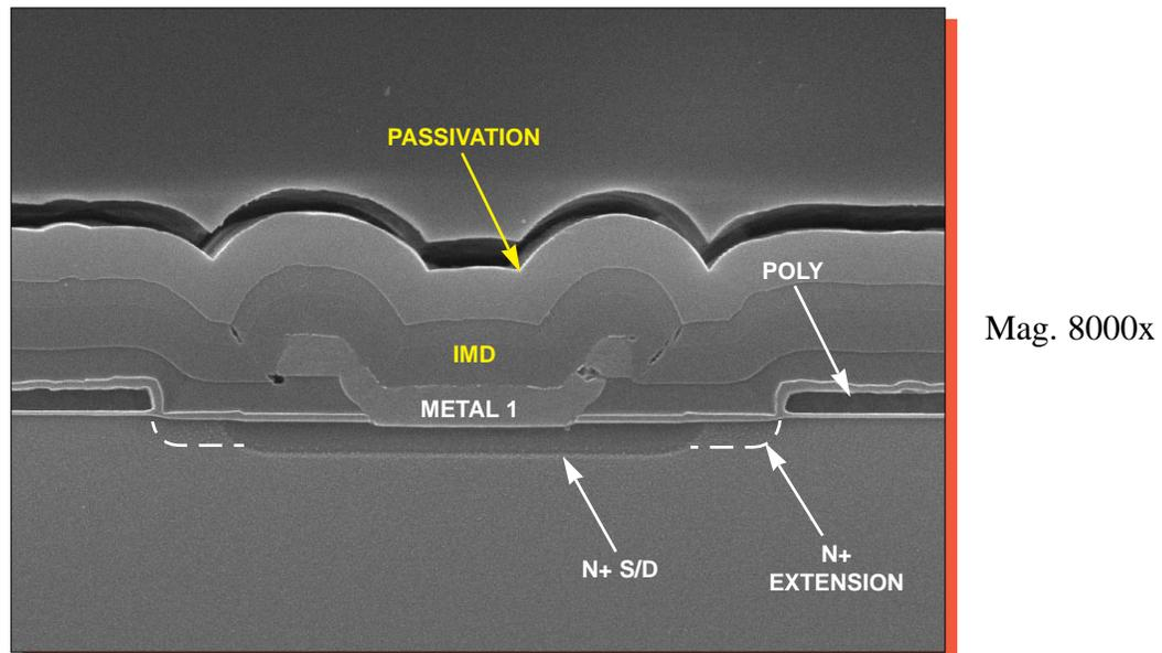
Figure 19. SEM section views of various N-channel structures.
