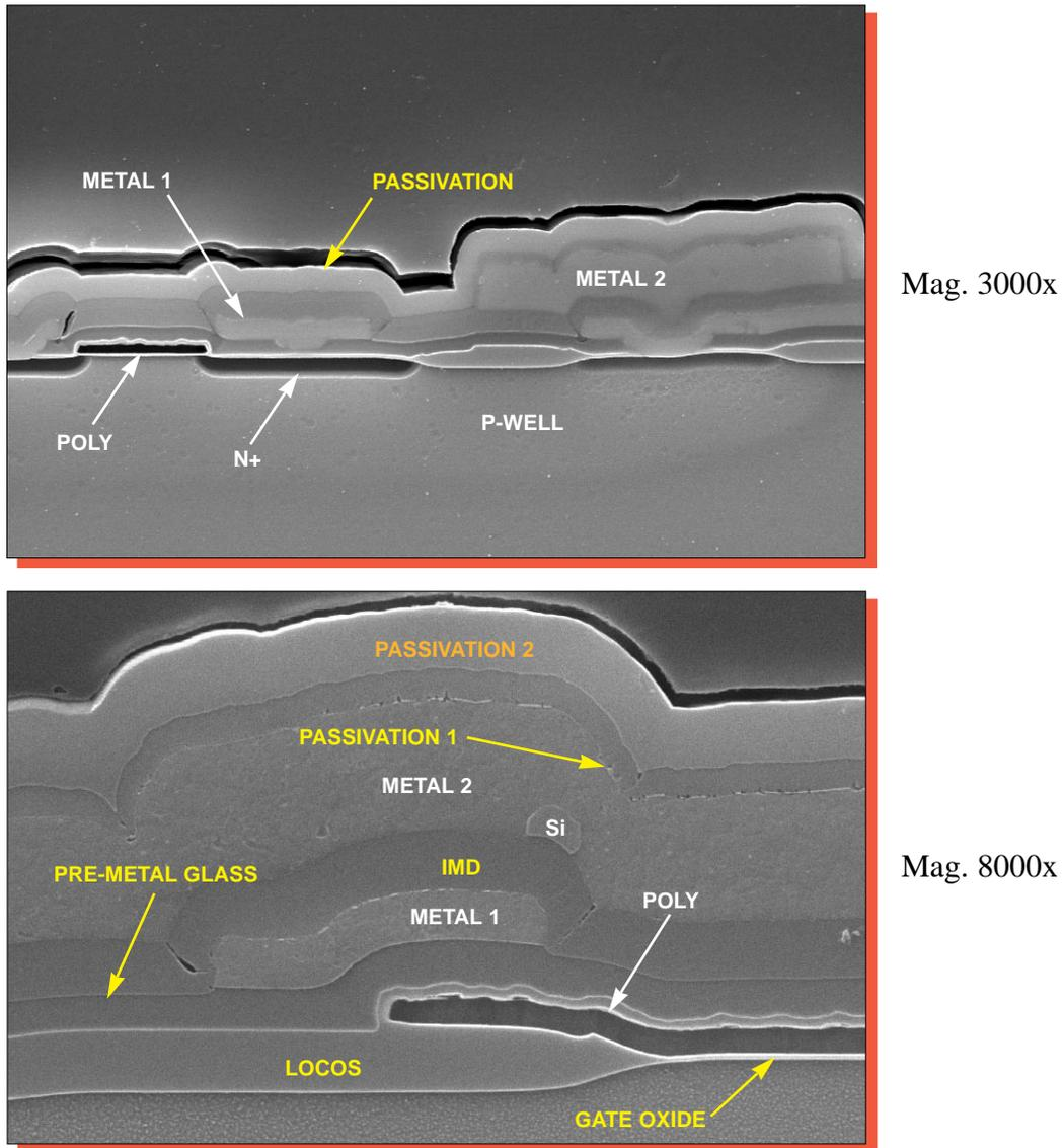
Figure 8a. SEM section views illustrating general construction.
