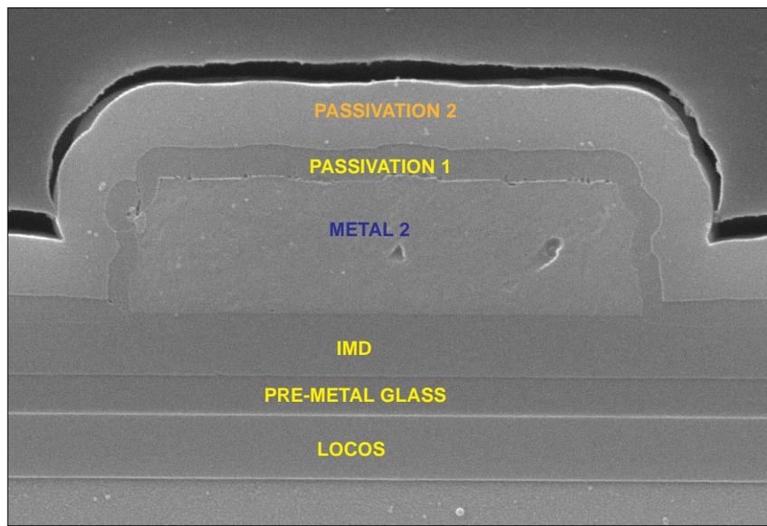
Figure 9. SEM section view of a metal 2 line profile. Mag. 10,000x.
