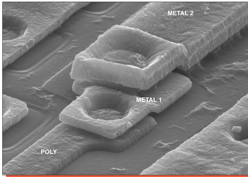
Figure 11a. Detailed SEM view of a metal 2-to-metal 1 via. Mag. 5000x, 60°.
