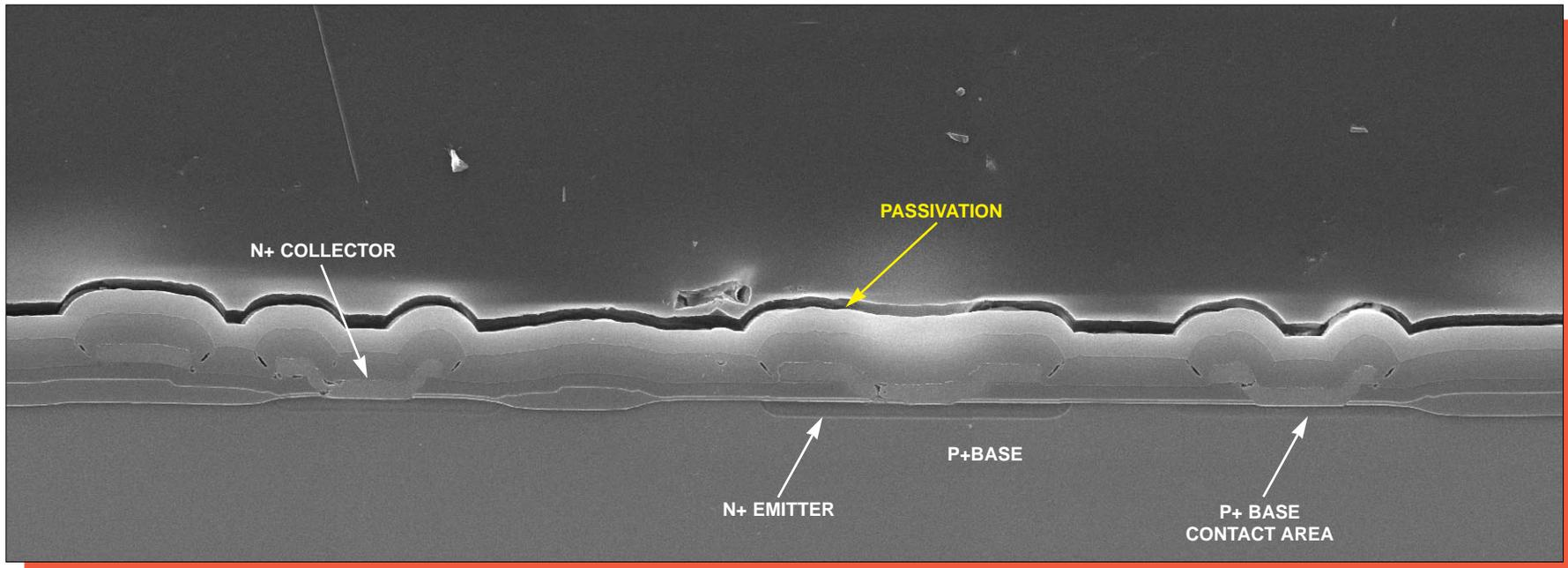
Figure 26. SEM section view of an NPN transistor. Mag. 3500x.
