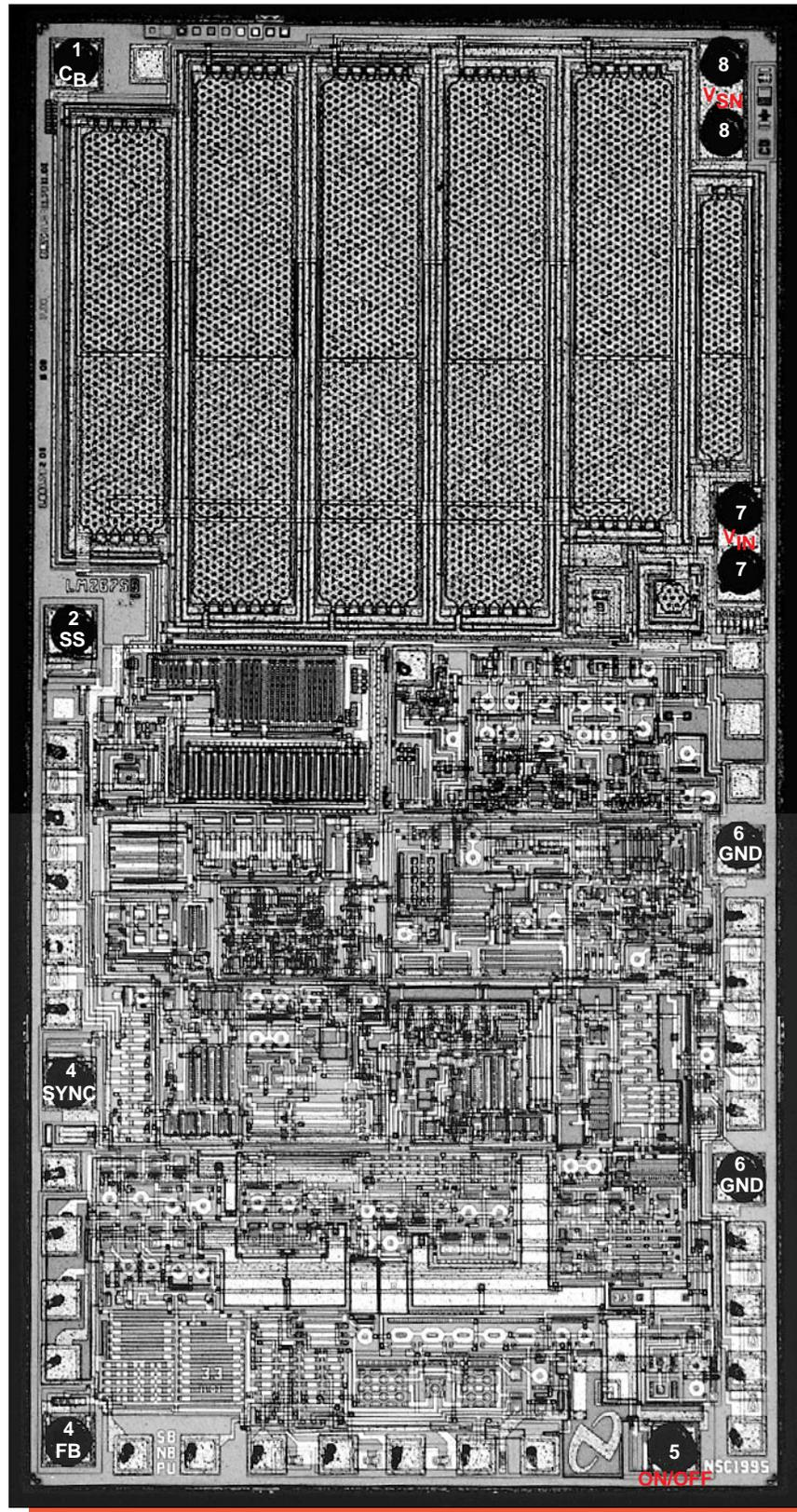
Figure 5. Whole die photograph of the National LM2672 device. Mag. 60x.
