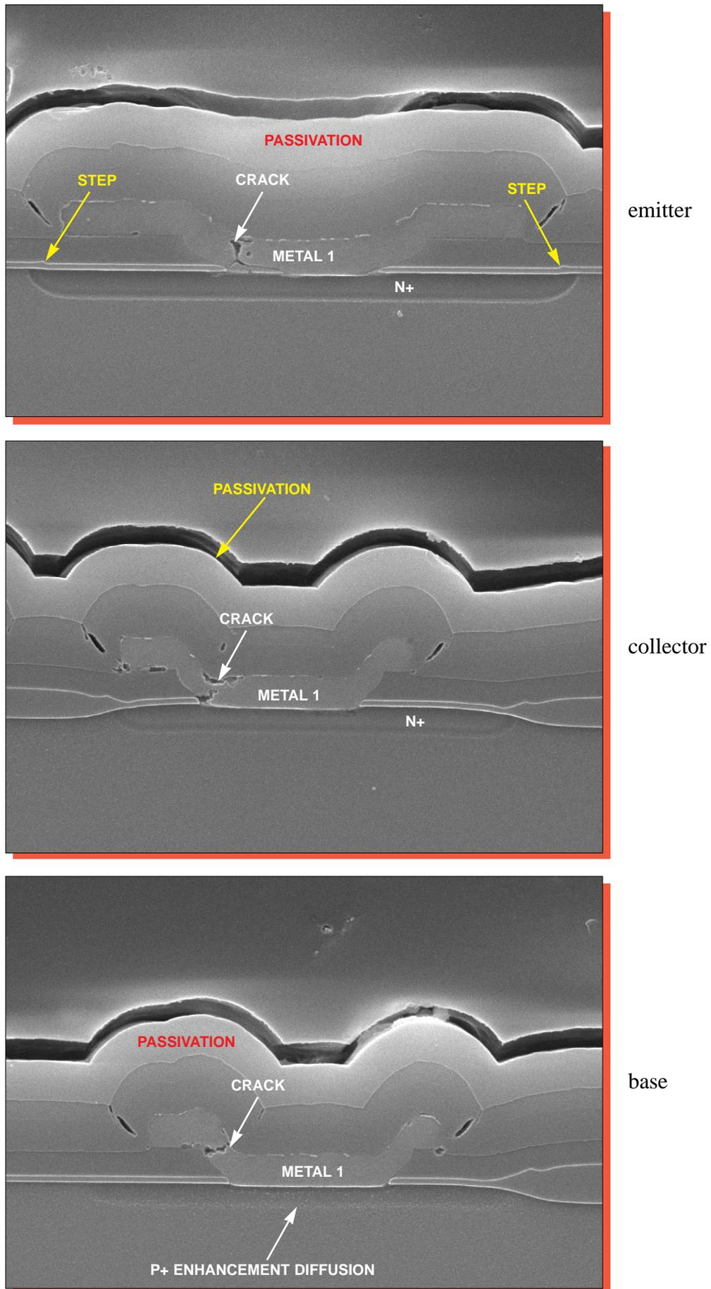
Figure 27. Detailed views of the NPN transistor. Mag. 8000x.
