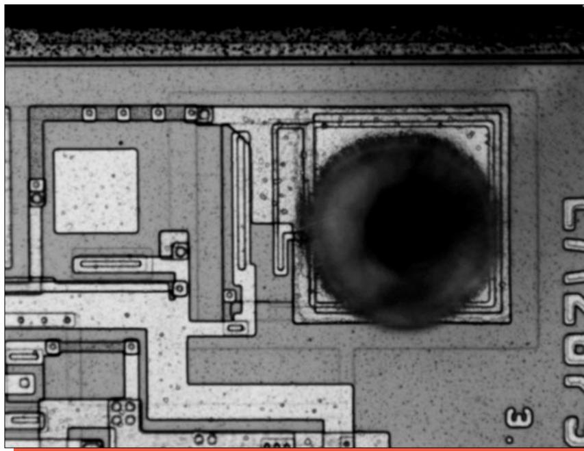
Figure 30. Optical views of probe damage and input layout (Pin 2, SS). Mag. 320x.
