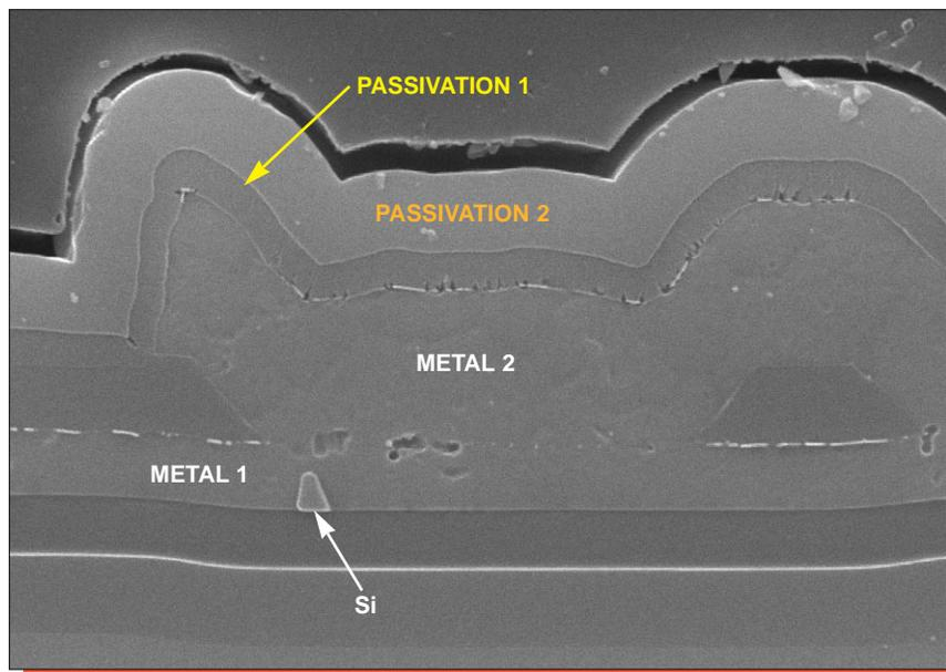
Figure 11b. SEM section view of a metal 2-to-metal 1 via. Mag. 10,000x.
