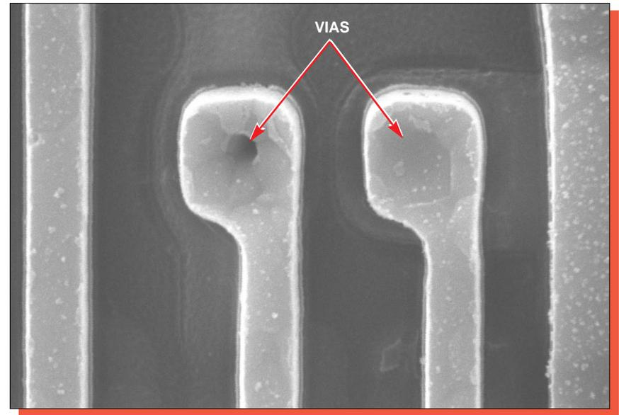
Figure 12. Topological SEM views of metal 2 design rule features. Mag. 13,000x, 0°.
