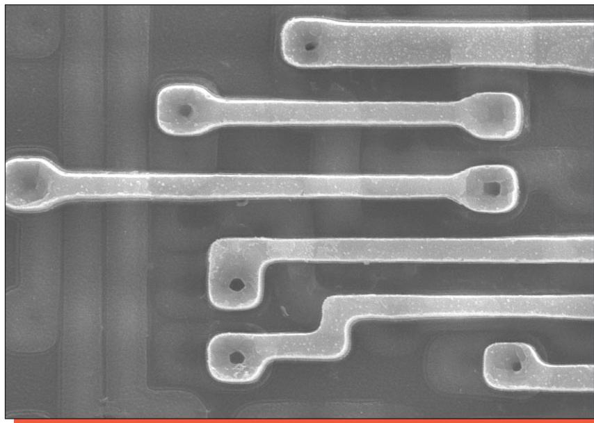
Figure 11. Topological SEM views of metal 2 patterning. Mag. 5500x, 0°.
