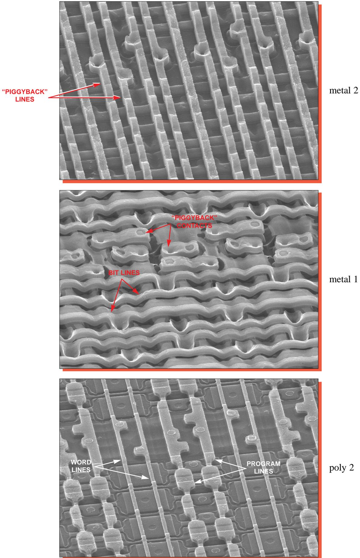
Figure 32. Perspective SEM views of the EEPROM array. Mag. 4000x, 55°.
