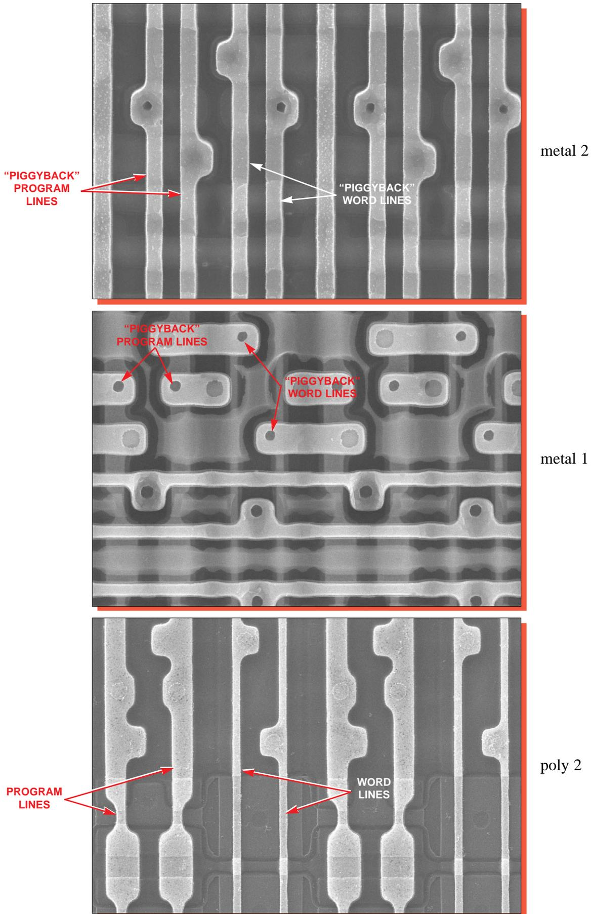
Figure 31. Topological SEM views of the EEPROM array illustrating “piggyback” word line connections. Mag. 5000x, 0°.
