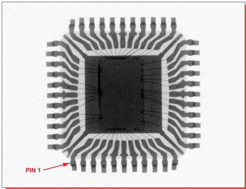
Figure 1. Package photograph and x-ray view of the Xilinx XC9536. Mag. 6x.
