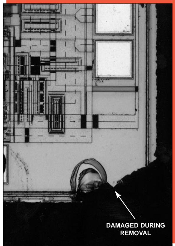
Figure 5. Optical views of die corners. Mag. 160x.
