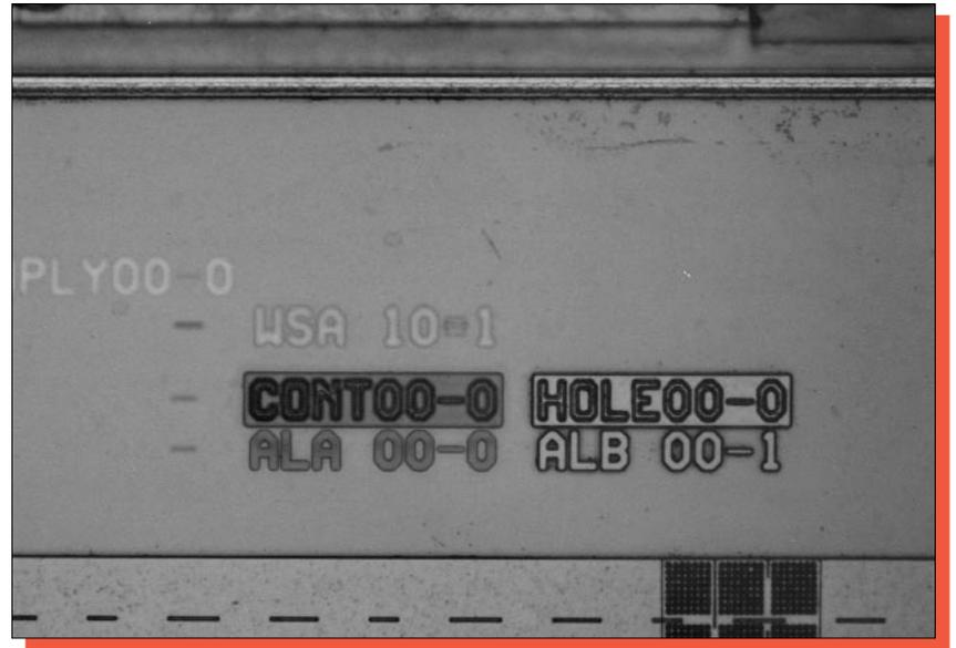
Figure 3. Die identification markings. Mag. 400x.
