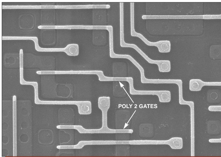
Figure 23. Topological SEM views of poly patterning. Mag. 4000x, 0°.
