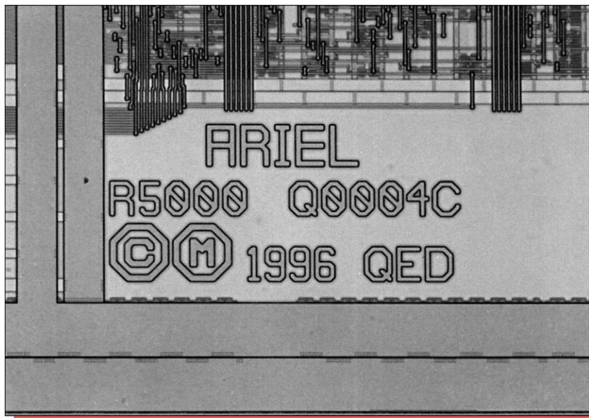
Figure 7. Die identification markings from the surface. Mag. 320x.
