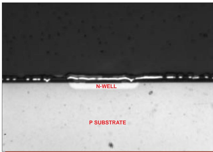
Figure 19. Optical section view illustrating the well structure. Mag. 800x.
