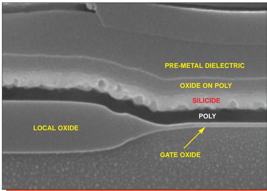
Figure 18. SEM section view of a typical local oxide birdsbeak. Mag. 40,000x.
