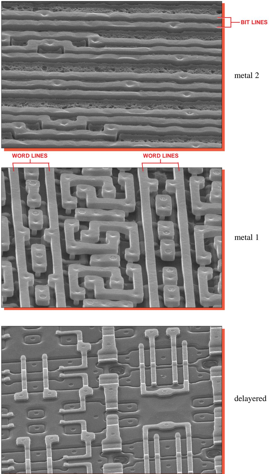
Figure 29. Perspective SEM views of the SRAM cell array. Mag. 5000x, 60°.
