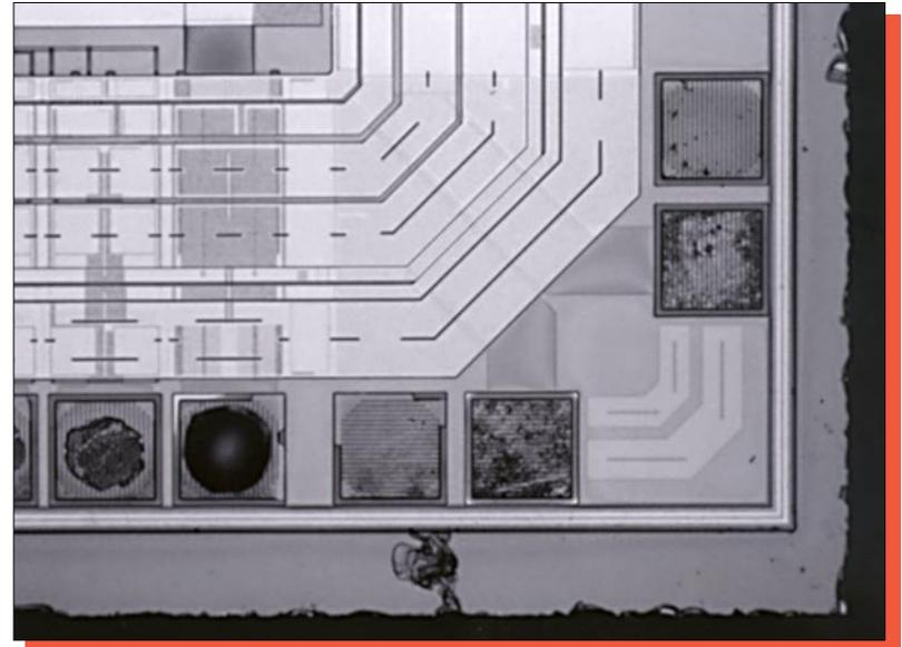
Figure 9a. Optical views of the die corners on the PLX Technology PCI9080 device. Mag. 160x.
