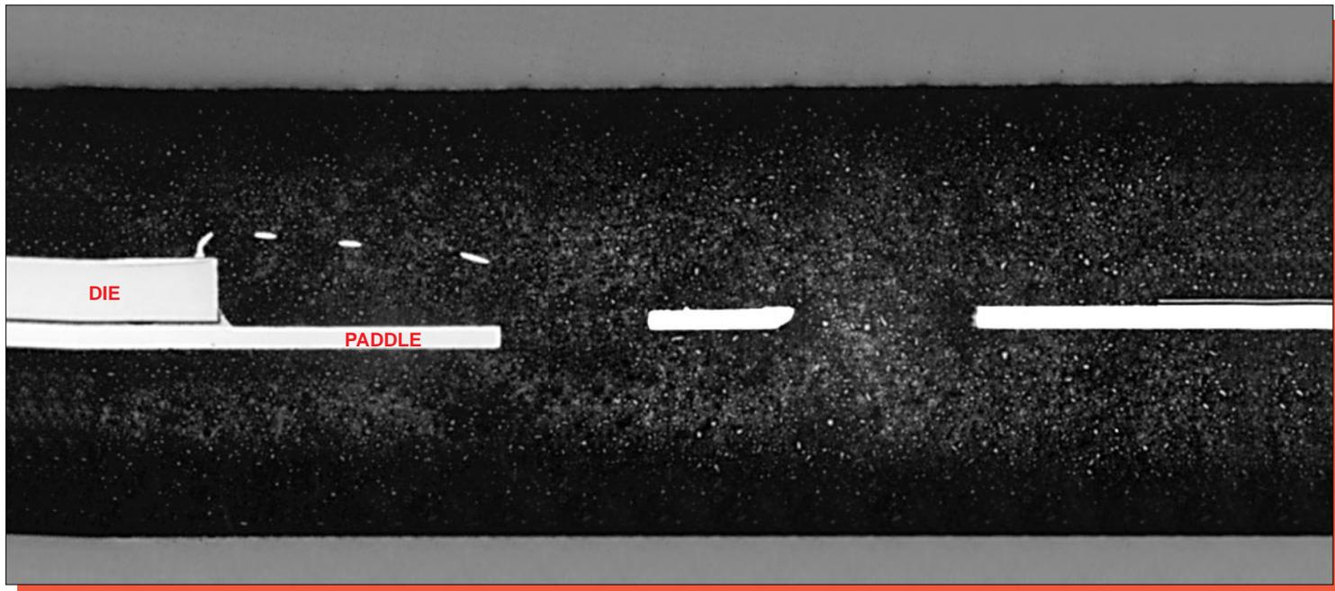
Figure 4a. Optical views of the PLX Technology package illustrating general construction. Mag. 20x.
