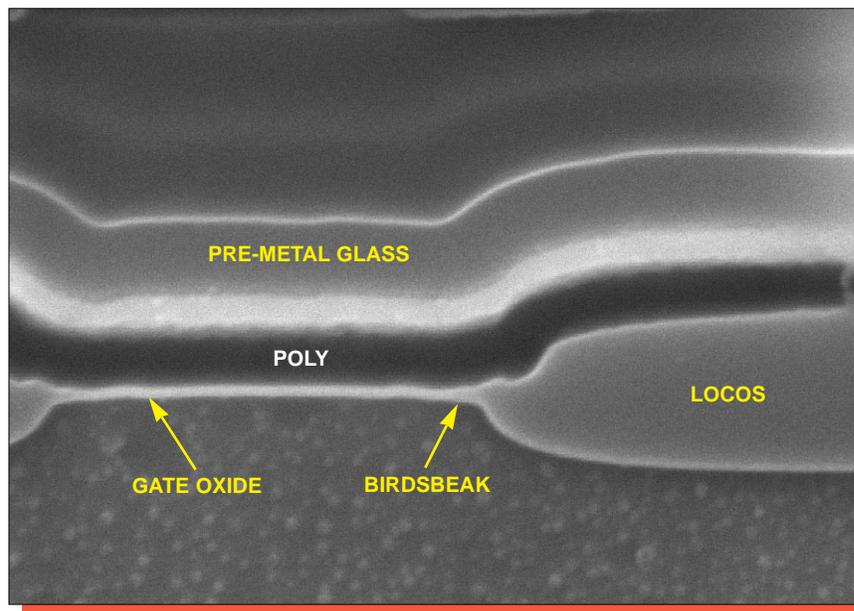
Figure 27. SEM section view of a local oxide birdsbeak. Mag. 52,000x.
