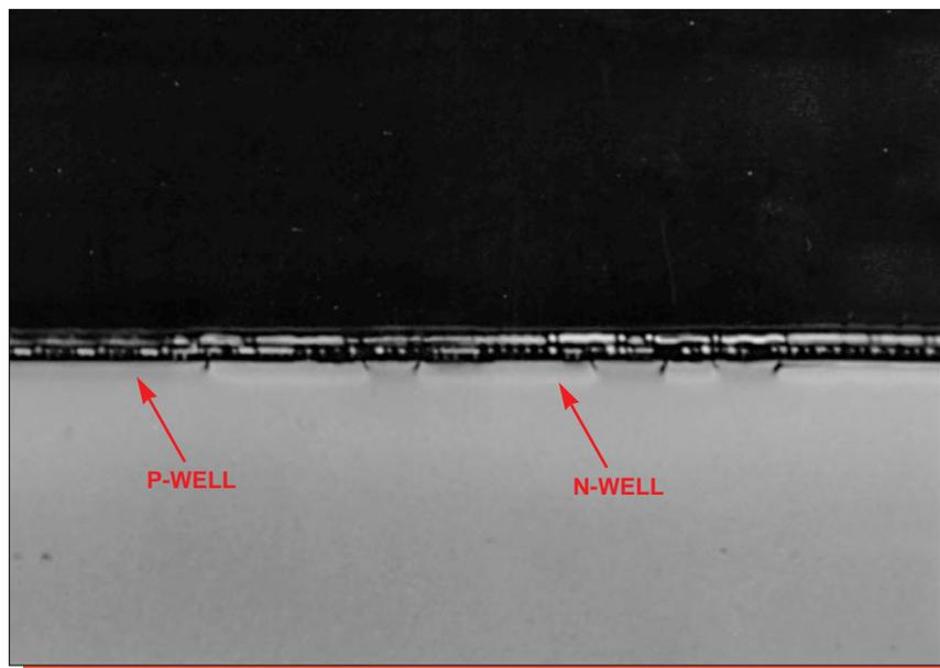
Figure 28. Optical section view of the well structure. Mag. 800x.
