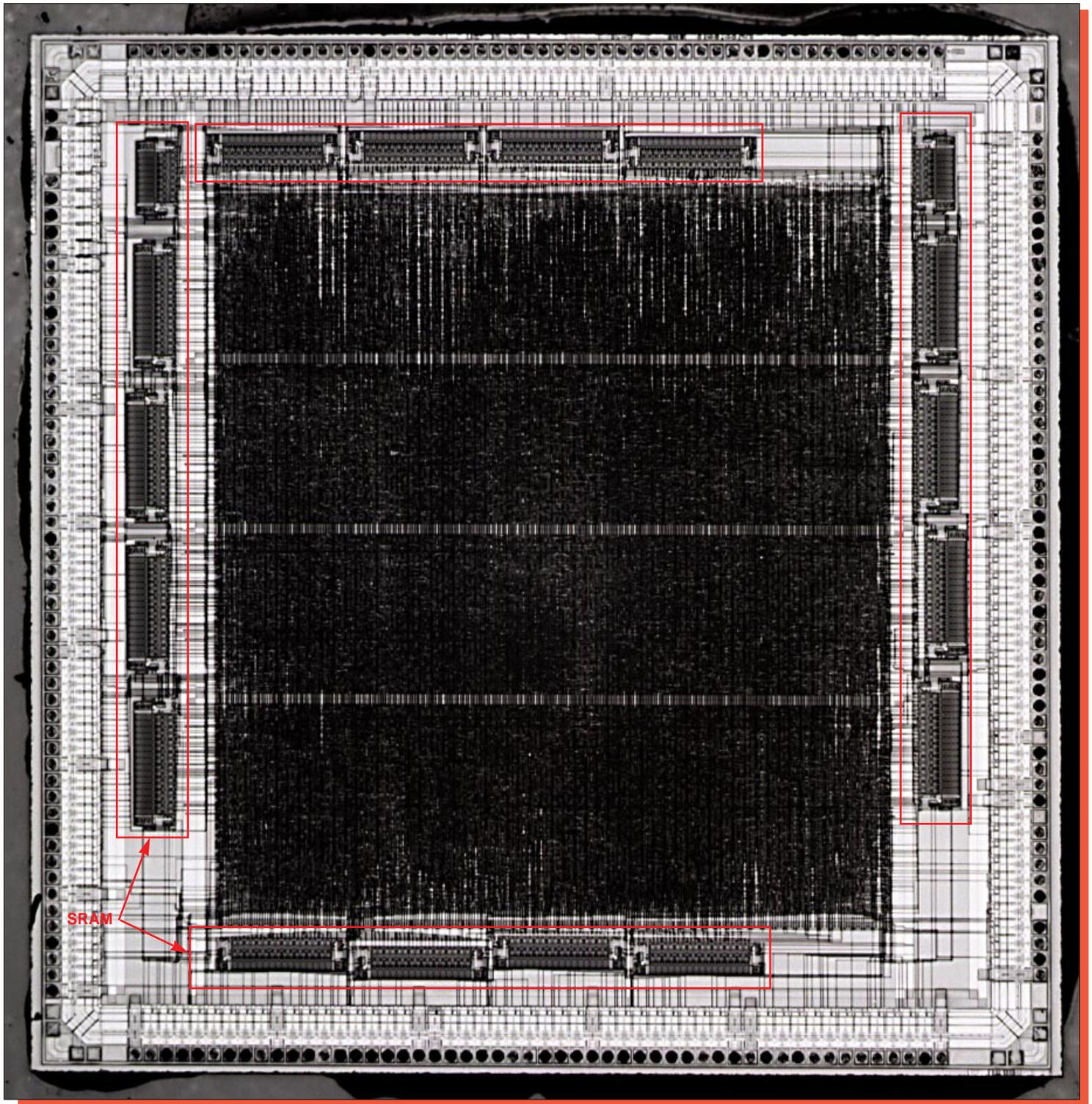
Figure 9. The PLX Technology PCI9080 intact circuit die. Mag. 29x.
