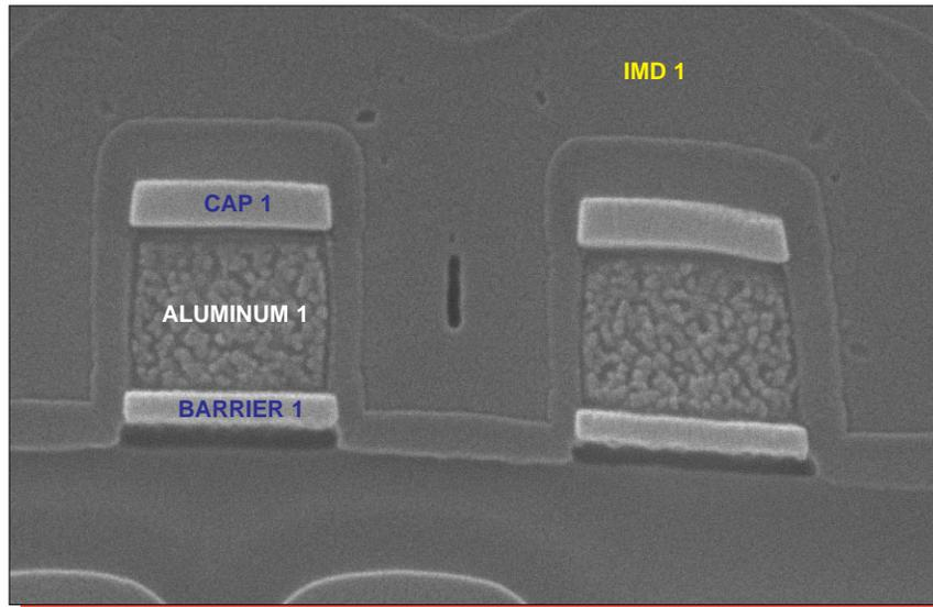
Figure 21. SEM section view of metal 1 line profiles. Mag. 40,000x.
