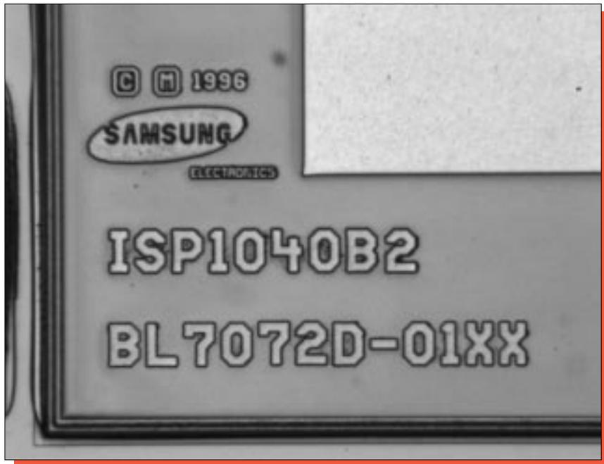
Figure 9a. Optical view of markings from the surface of the die. Mag. 300x.
