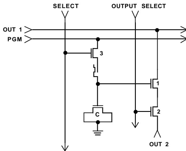
Figure 26. SEM section views and schematic of the EEPROM cell array (cell A).
