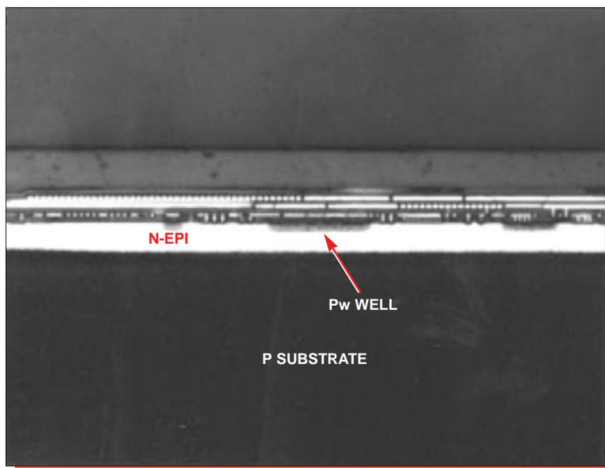
Figure 20. Section view illustrating the well structure. Mag. 800x.
