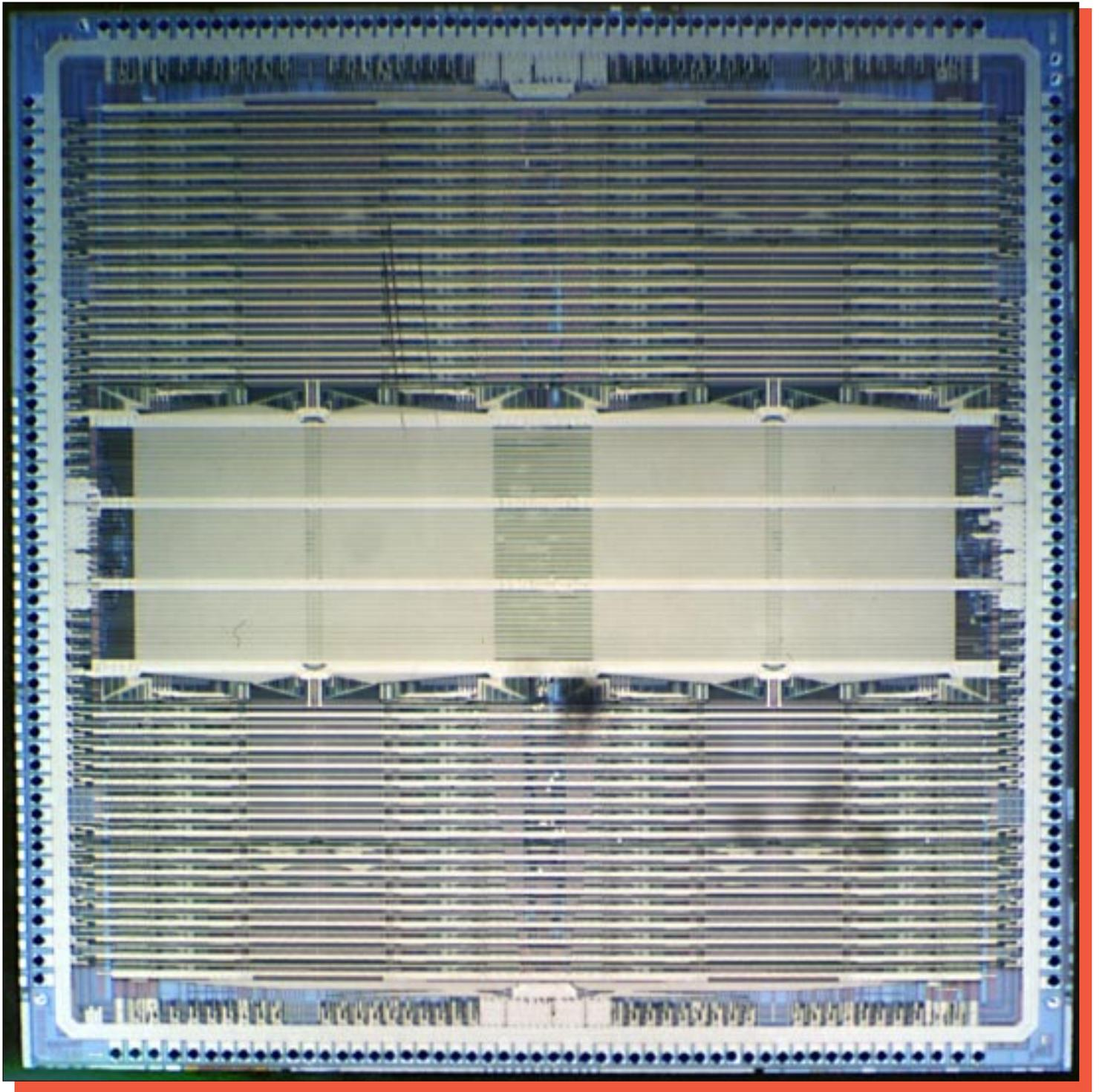
Figure 1. Whole die photograph of the AMD/Vantis MACHL V466-10. Mag. 10x.
