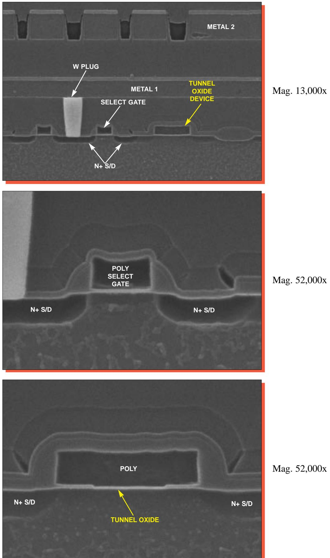
Figure 27. SEM section views of an EEPROM cell (cell A). X-direction.
