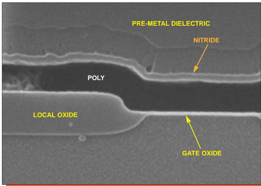
Figure 19. SEM section view of a typical local oxide birdsbeak. Mag. 52,000x.
