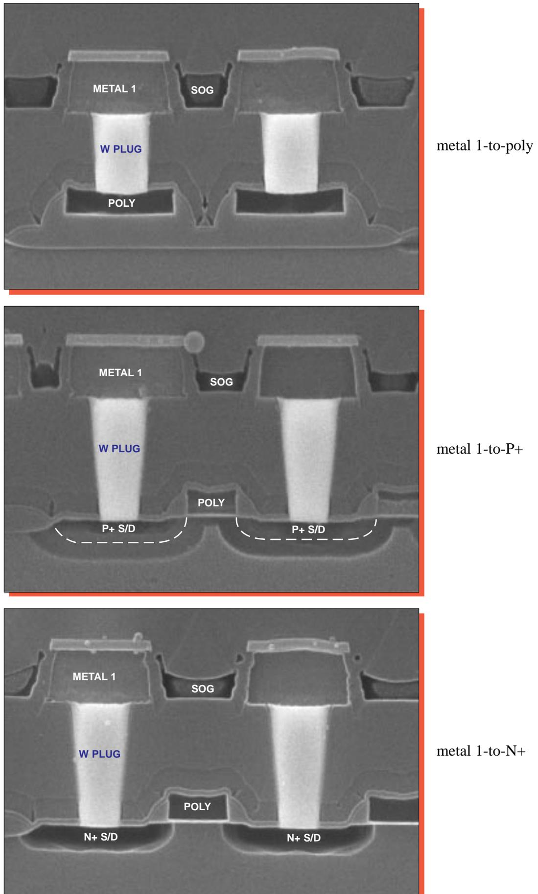
Figure 15. SEM section views of metal 1 contacts (silicon etch). Mag. 26,000x.
