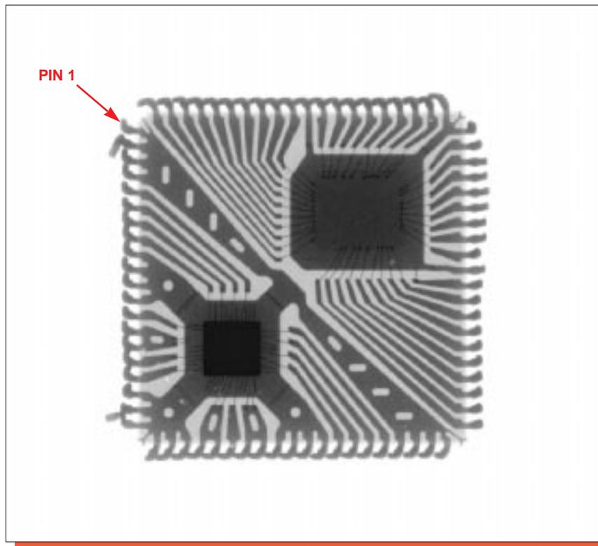
Figure 2. X-ray view of the package. Mag. 4.5x.
