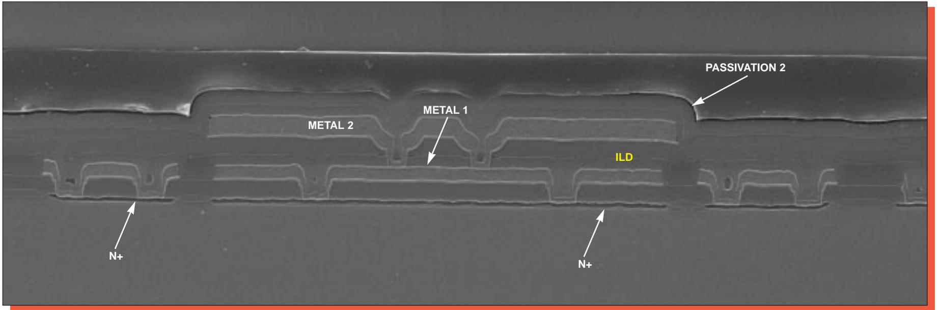
Figure 33. SEM section view of the I/O circuitry. Mag. 6500x.
