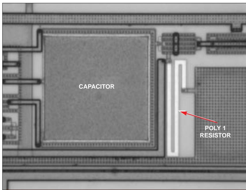
Figure 28. Optical views of resistors and a capacitor. Mag. 600x.
