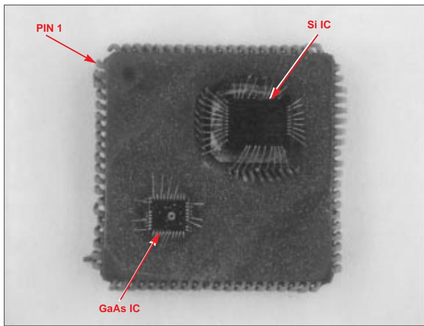
Figure 3. Optical view illustrating decapsulated package. Mag. 4.5x.
