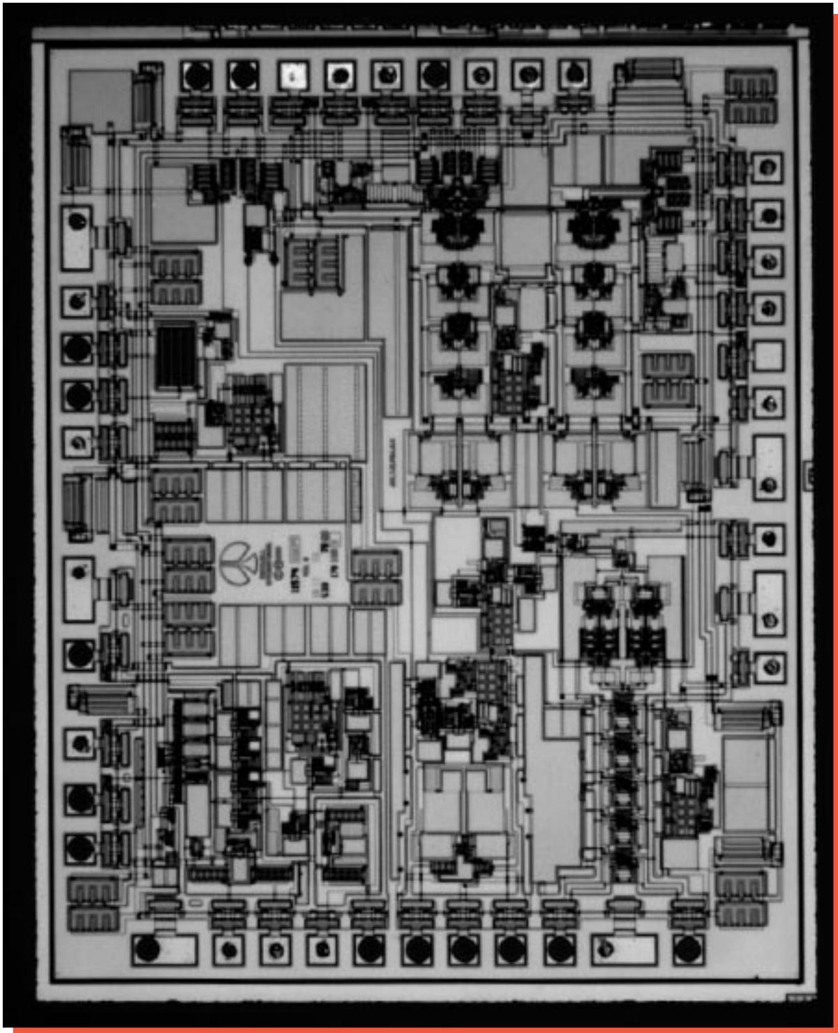
Figure 7. Whole die photograph of the Silicon IC. Mag. 45x.
