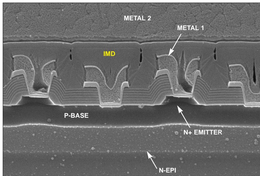
Figure 44. Additional SEM section view of the mesa emitter contacts. Mag. 13,000x.
