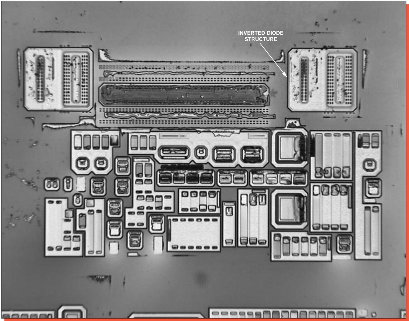
Figure 11b. Delayed optical view of circuit C. Mag. 540x.
