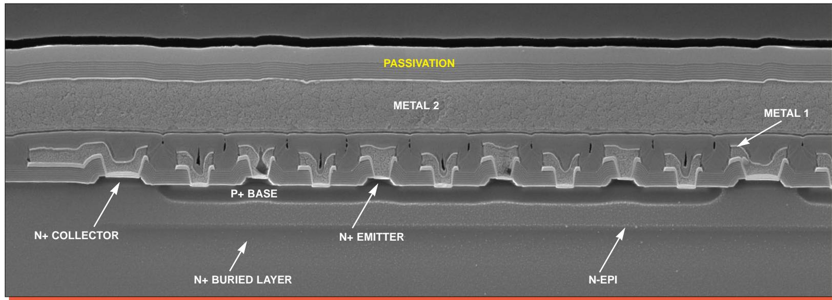
Figure 41a. SEM section view of a large input device with multiple emitter and base contacts (requested section). Mag. 6500x.
