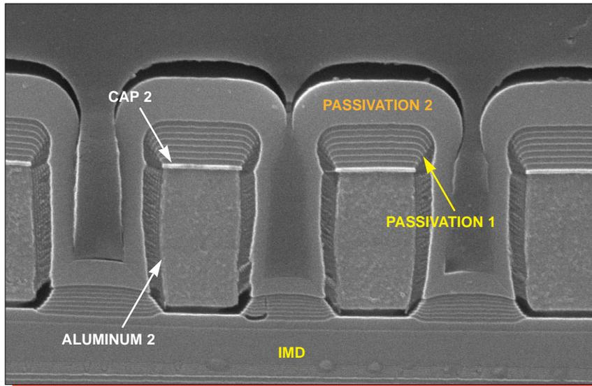
Figure 15. SEM section view of metal 2 line profiles. Mag. 13,000x.
