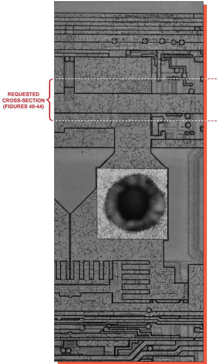
Figure 40. Optical view of a typical input structure. Mag. 400x.
