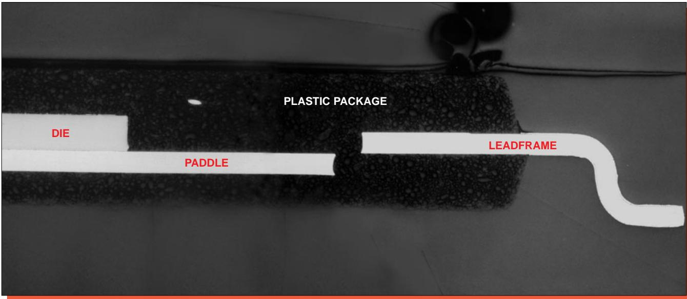
Figure 3. Package section views illustrating general construction. Mag. 40x.
