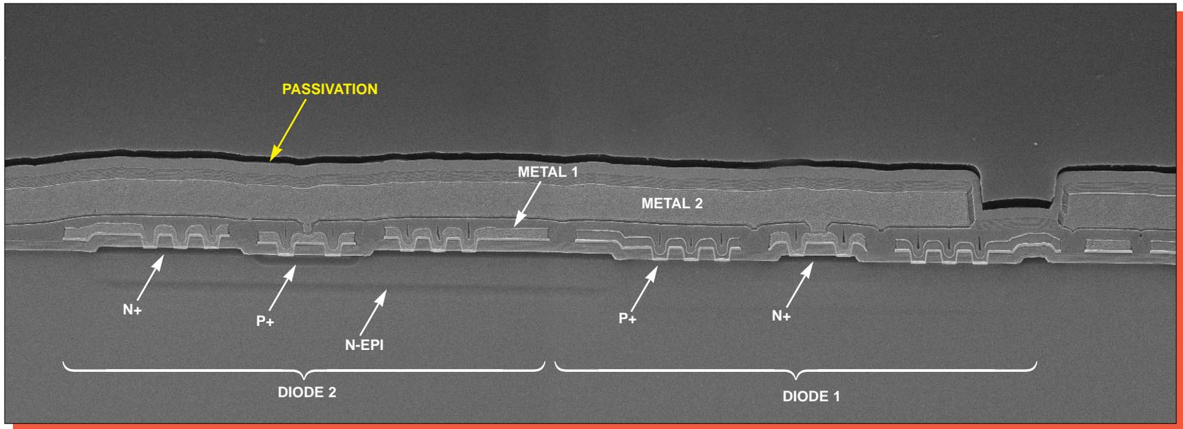
Figure 31. SEM section views illustrating an inverted diode structure. Mag. 3000x.
