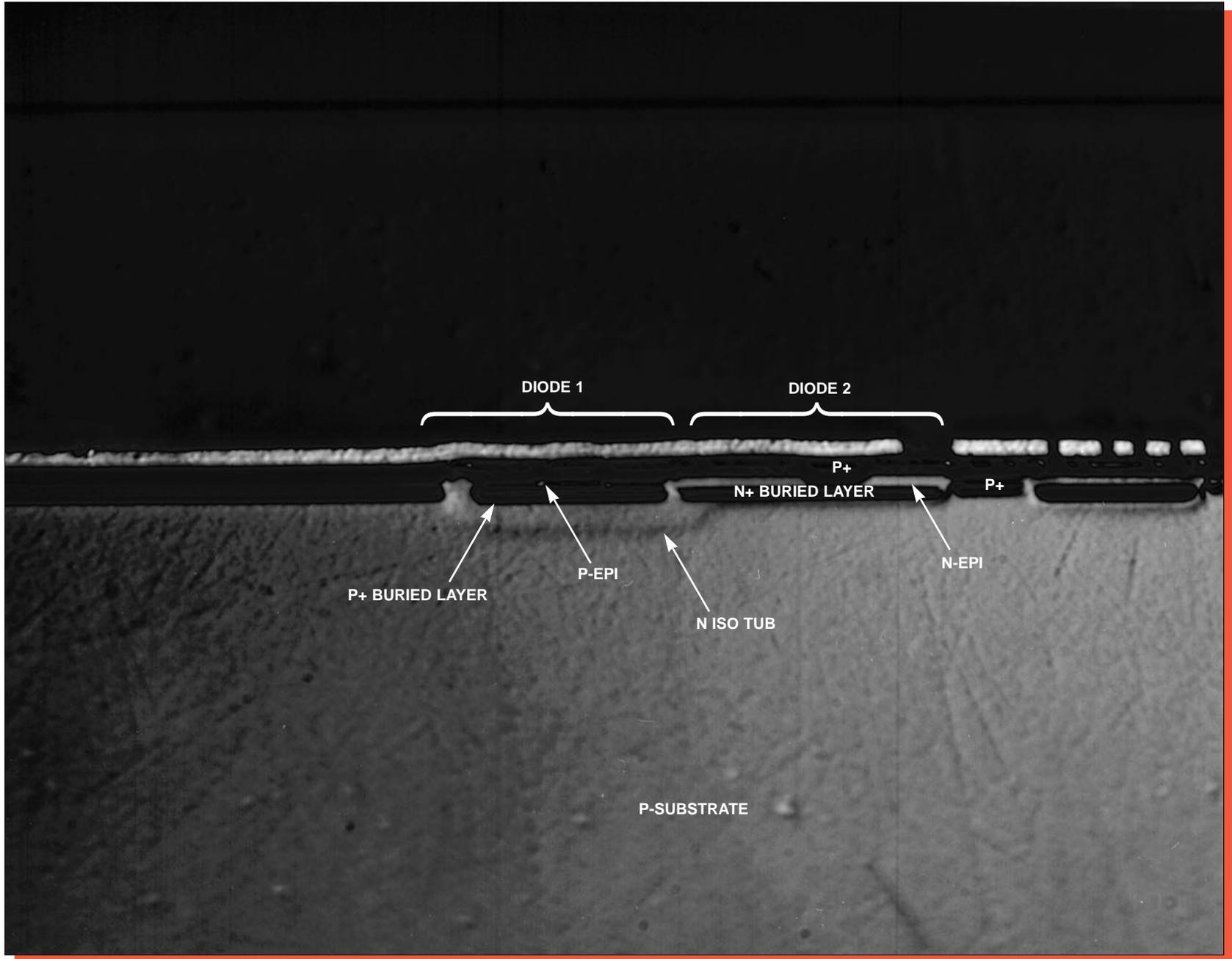
Figure 34. Optical view illustrating the inverted diode structure. Mag. 1600x.
