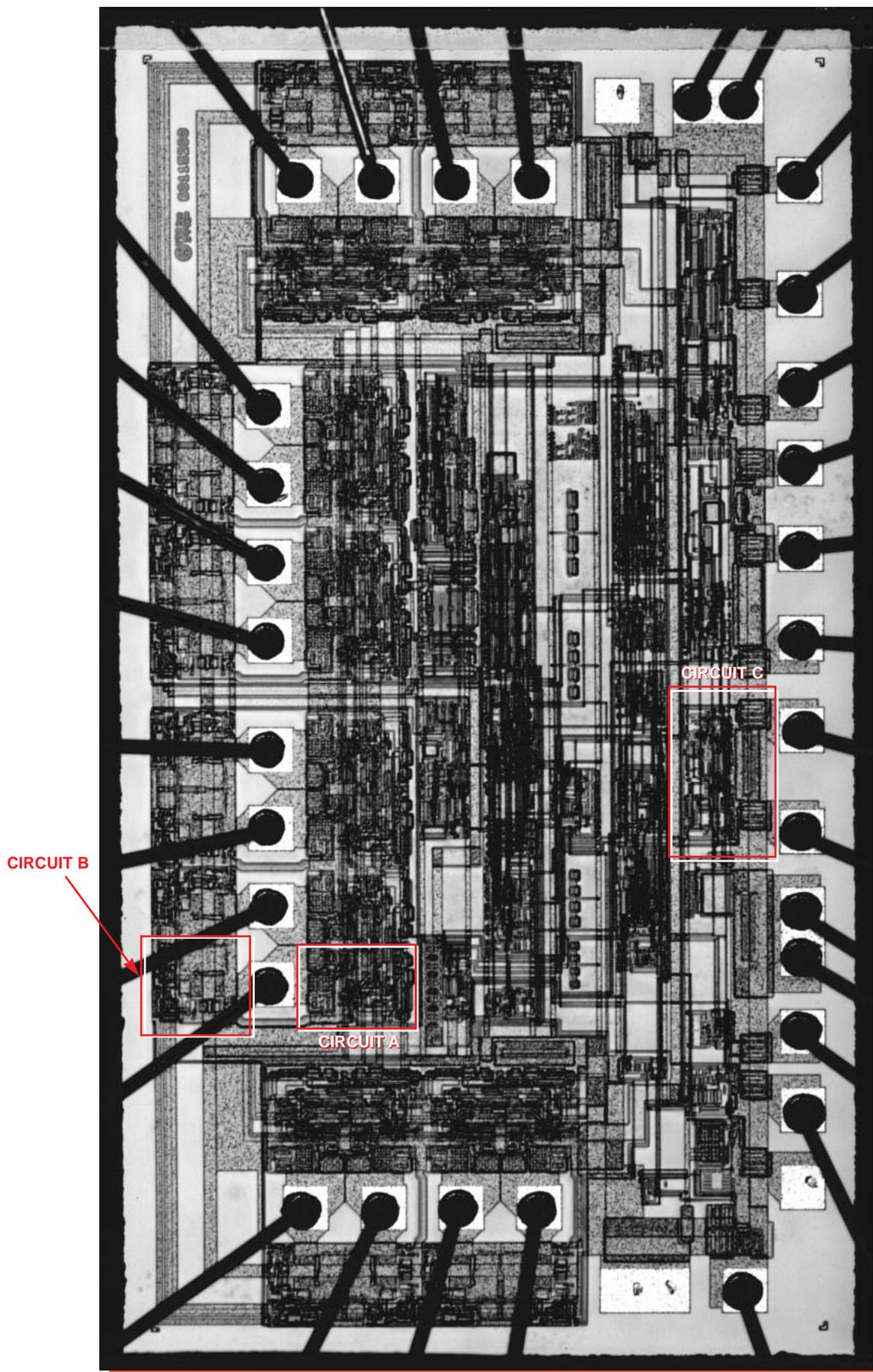
Figure 11. Whole die photograph of the VTC VM365830VSJ device. Mag. 80x.
