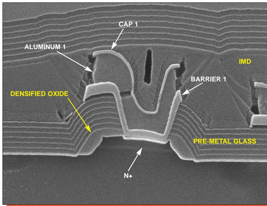
Figure 28. Detailed SEM section views through the capacitor and diode contacts.
