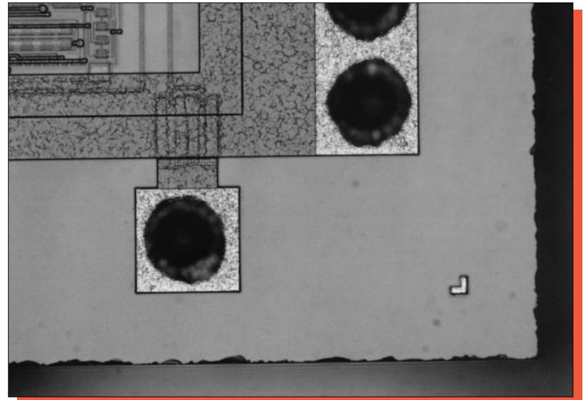
Figure 12. Optical views of the die corners on the VTC VM365830VSJ device. Mag. 200x.
