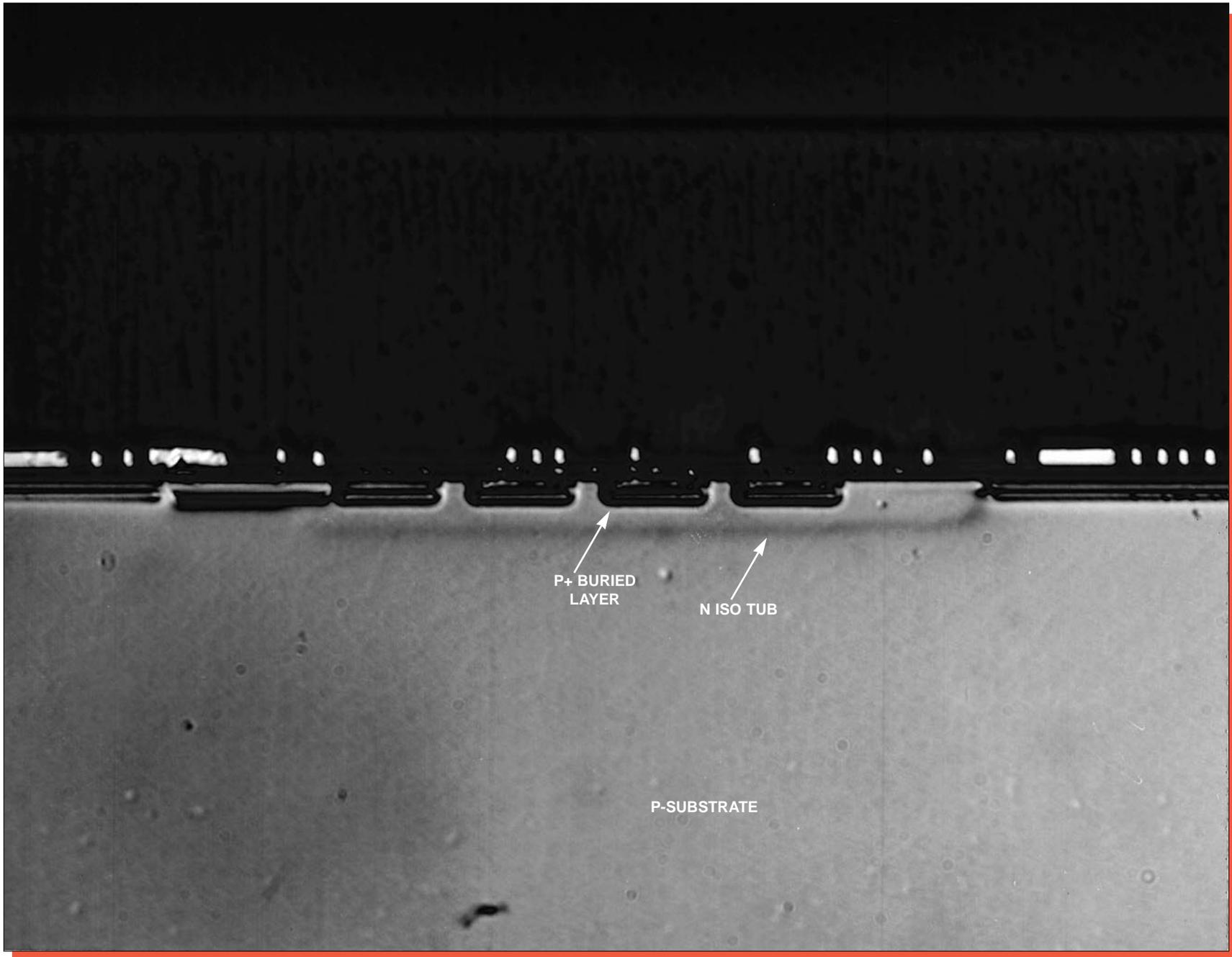
Figure 37. Optical section view illustrating the PNP transistors structure. Mag. 1600x.
