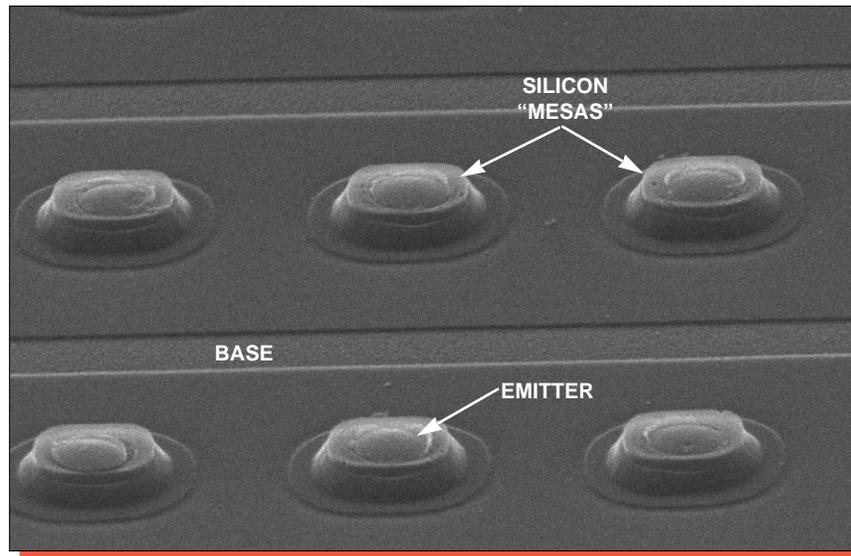
Figure 43. Perspective SEM view of the silicon "mesas". Mag. 13,500x.
