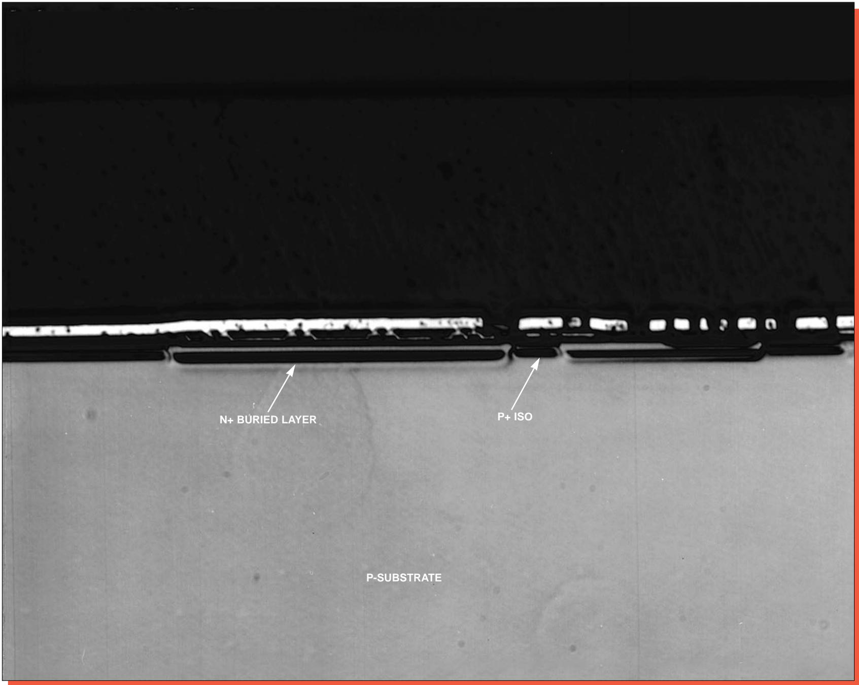
Figure 23a. Optical view illustrating general bipolar structure. Mag. 1600x.
