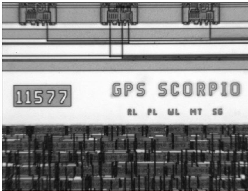
Figure 6. Optical views of die markings. Mag. 155x.
