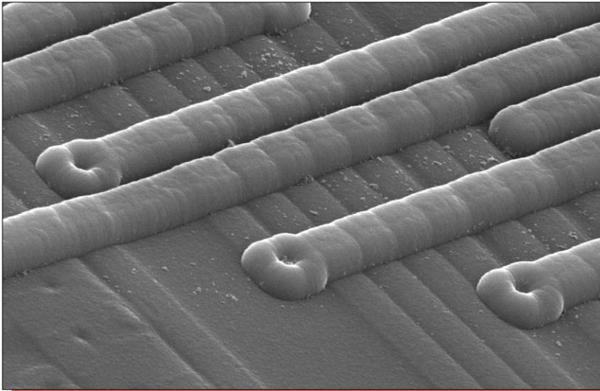
Figure 9. SEM view illustrating final passivation. Mag. 4800x, 60°.
