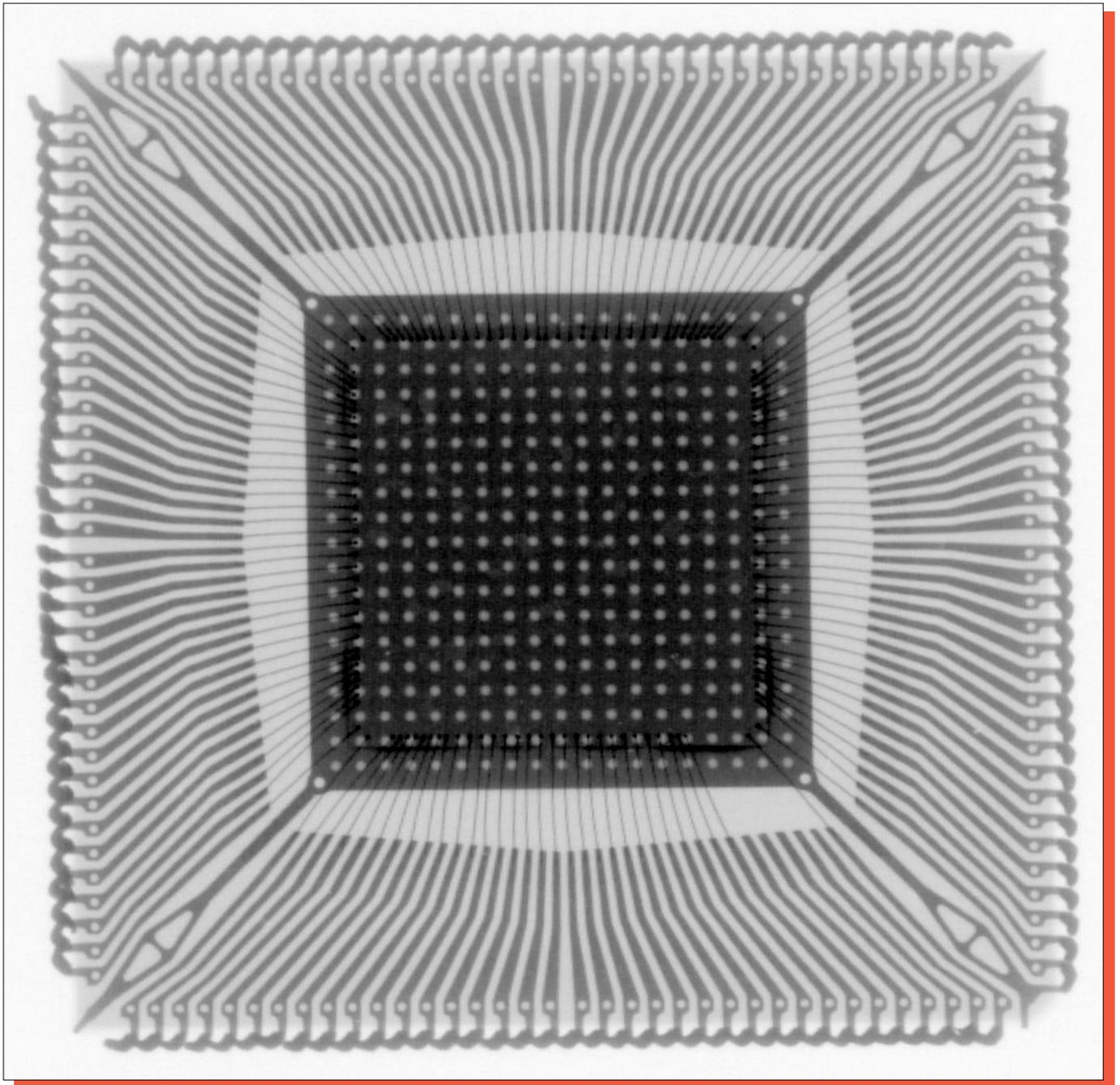
Figure 2. X-ray of the Rockwell 11577-11. Mag. 8x.
