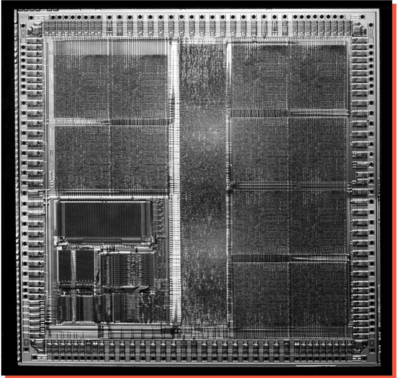
Figure 5. Whole die photograph of the Rockwell 11577-11. Mag. 20x.
