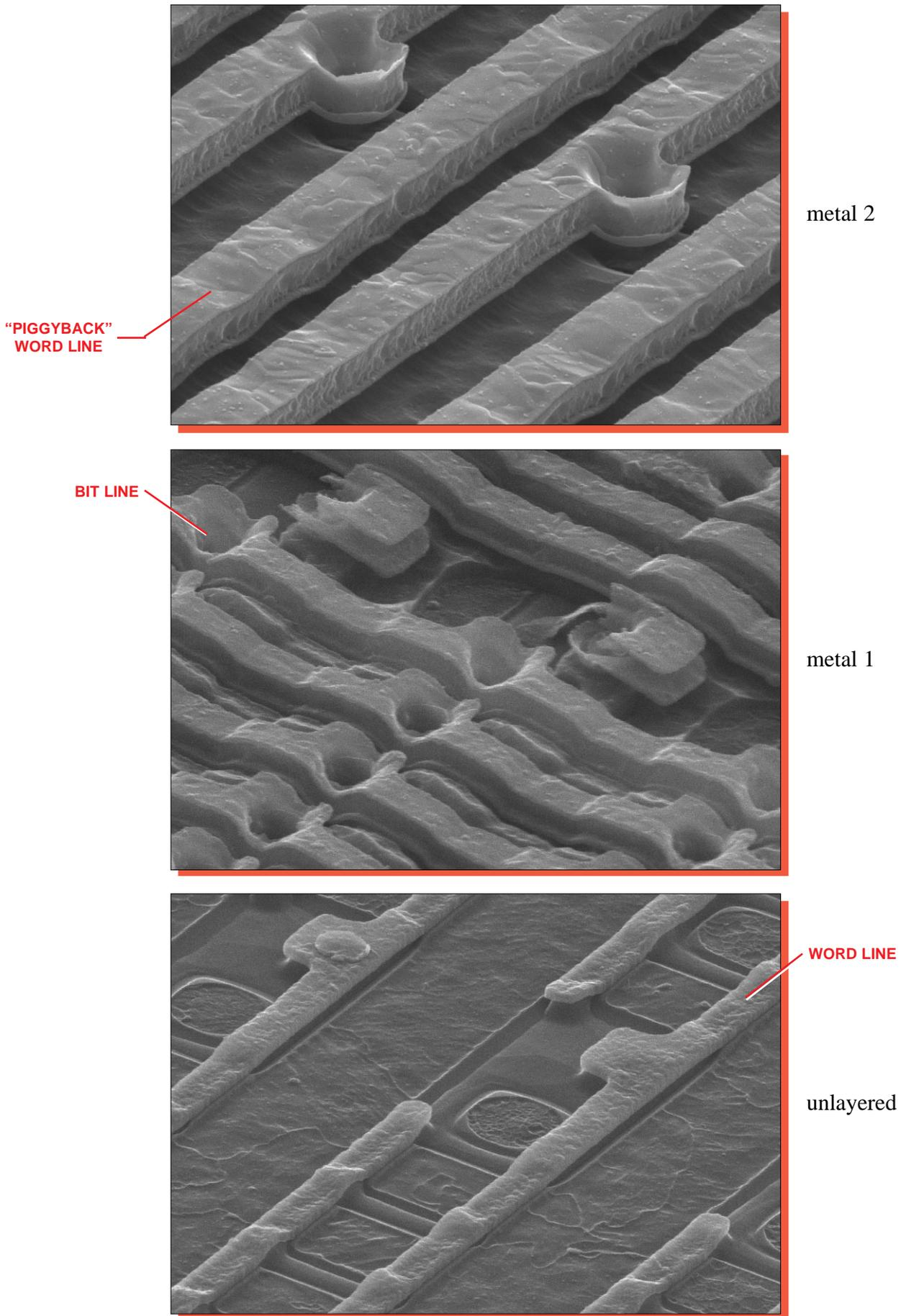
Figure 27. Detailed perspective SEM views of the MROM array. Mag. 10,000x, 60°.
