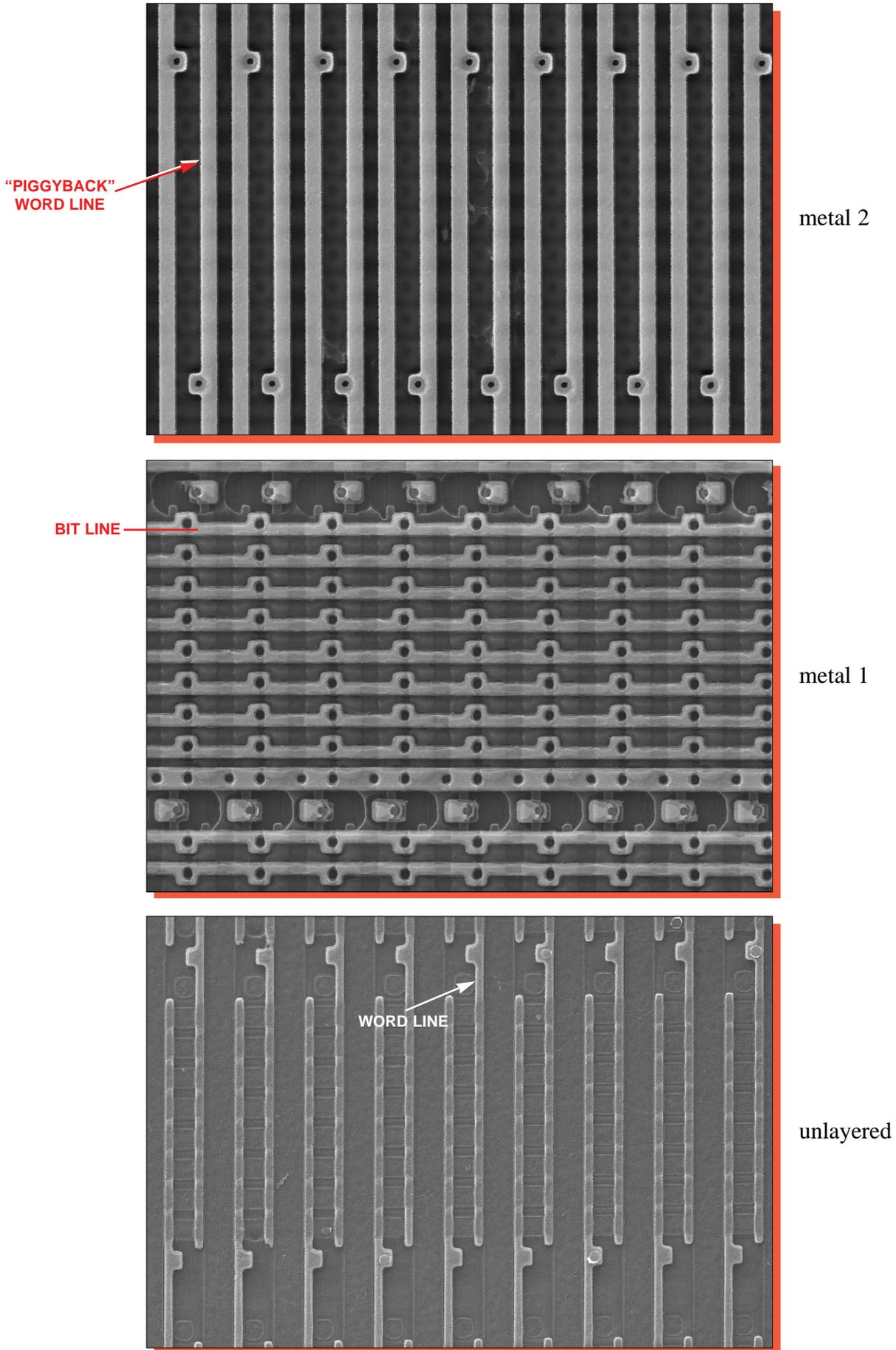
Figure 29. Topological SEM views of the MROM array. Mag. 2100x, 0°.
