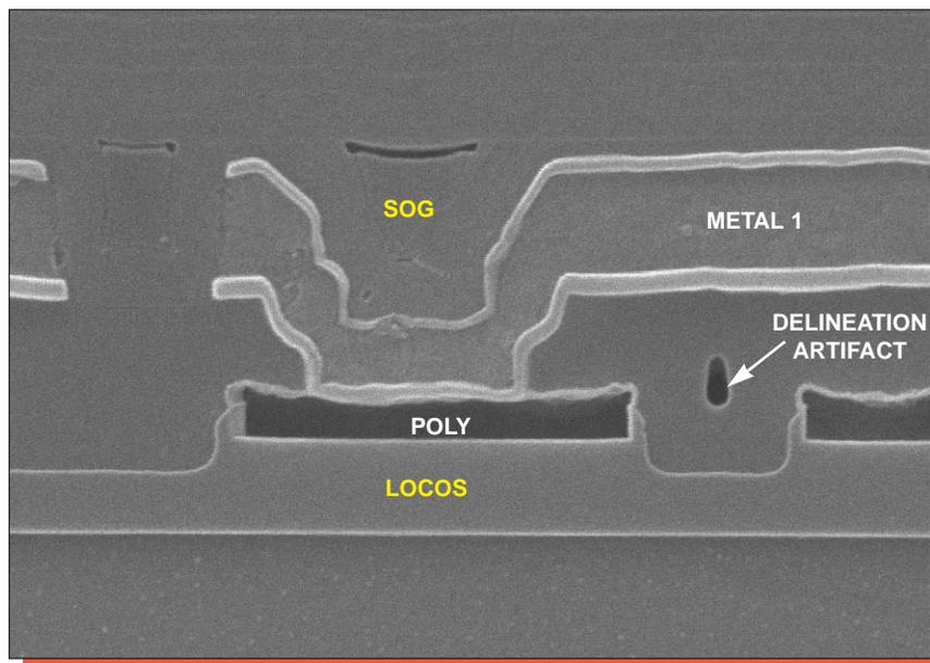
Figure 17. SEM section views of typical metal 1 contacts. Mag. 26,000x.
