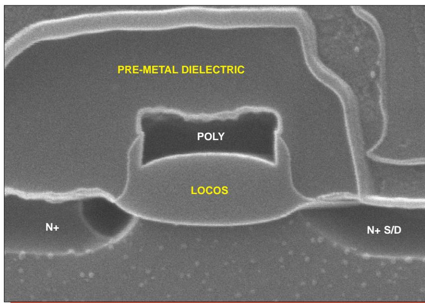
Figure 32. SEM section views of programmed cells. Mag. 52,000x.
