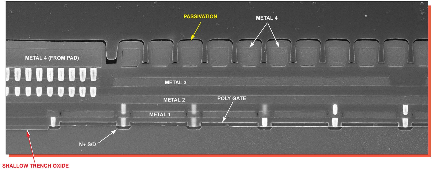
Figure 6. SEM section views of an I/O structure. Mag. 6000x.
