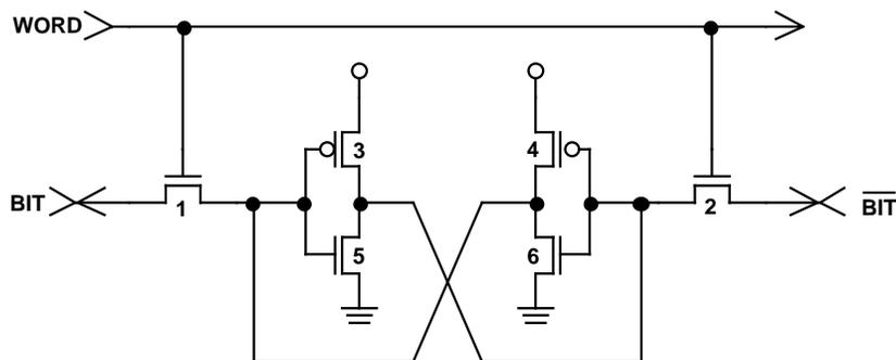
Figure 46. Topological SEM views and schematic of a Cache SRAM cell. Mag. 15,000x, 0°.
