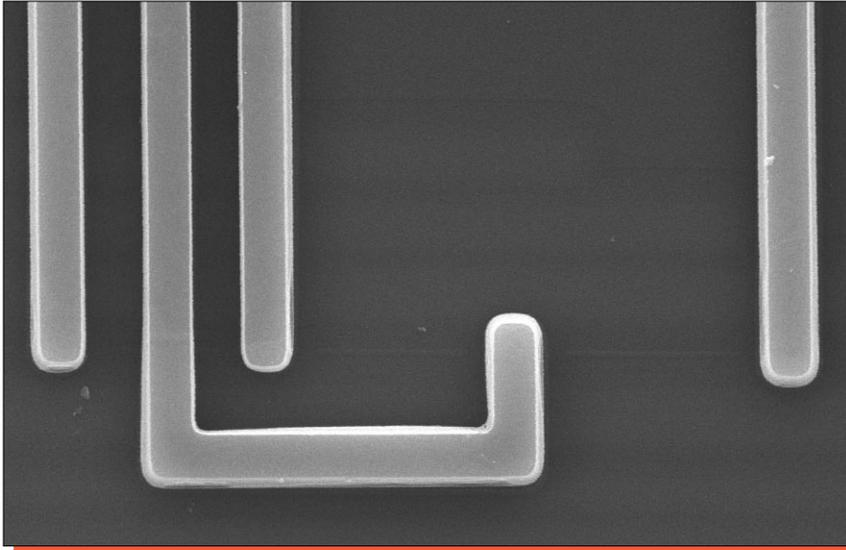
Figure 16. Topological SEM view of metal 4 patterning. Mag. 3700x, 0°.
