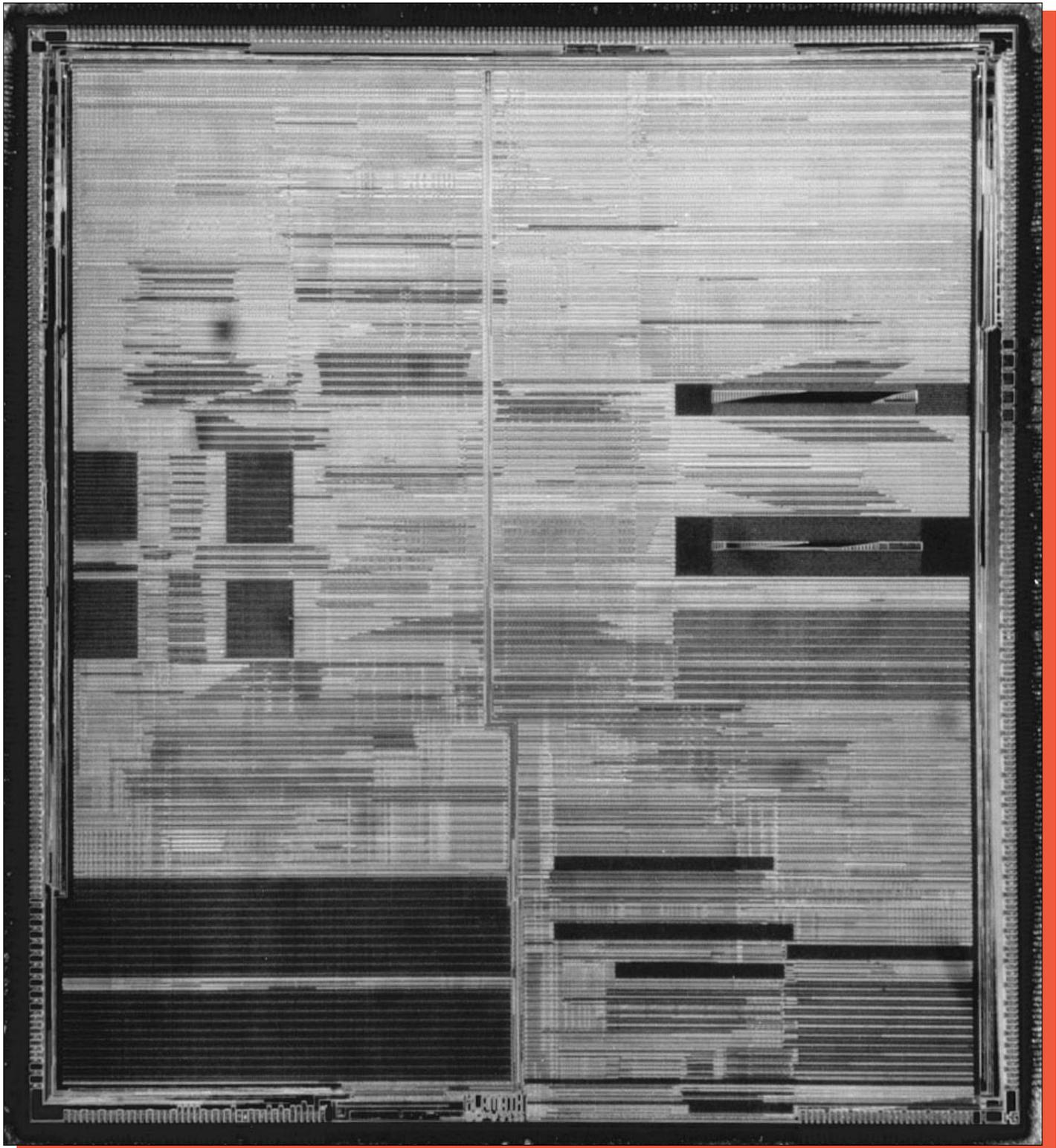
Figure 9. Whole die photograph of the Intel Pentium II Processor. Mag 14x.
