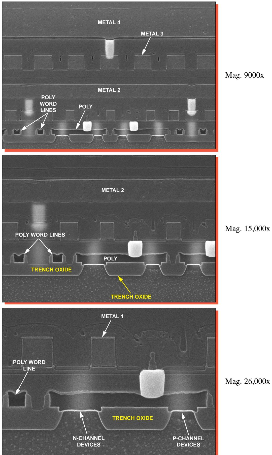
Figure 48. SEM section views of a Cache SRAM cell (parallel to storage and pull-up transistors).
