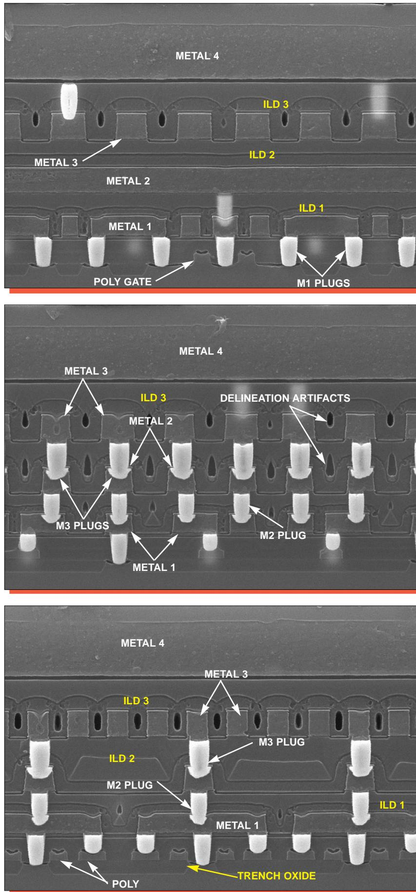
Figure 13. Glass etch section views illustrating general structure. Mag. 9000x.
