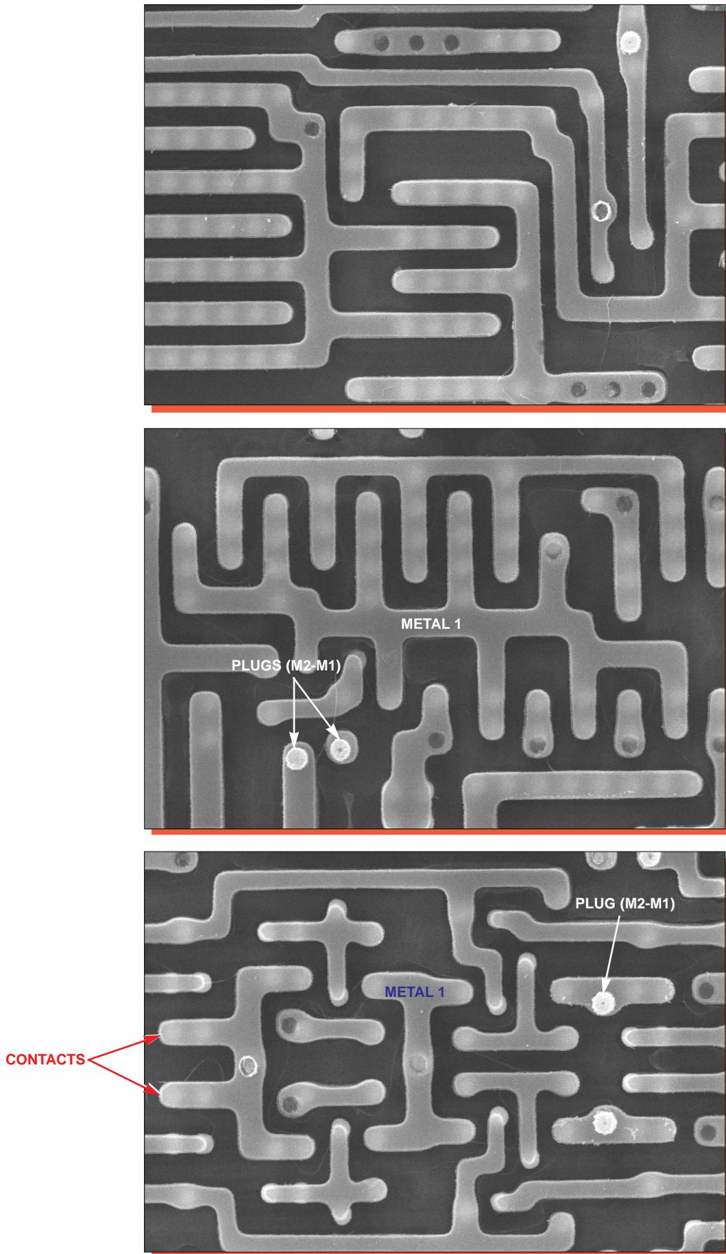
Figure 30. Topological SEM views of metal 1 patterning. Mag. 7000x, 0°.
