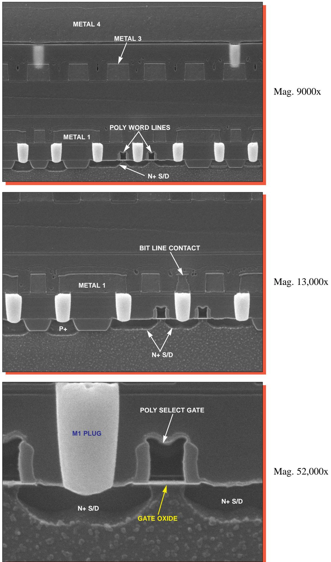
Figure 47. SEM section views of a Cache SRAM cell (perpendicular to word lines).
