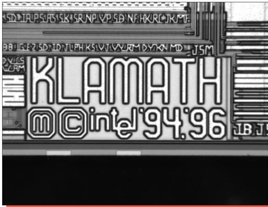
Figure 10. Die identification markings. Mag. 100x.
