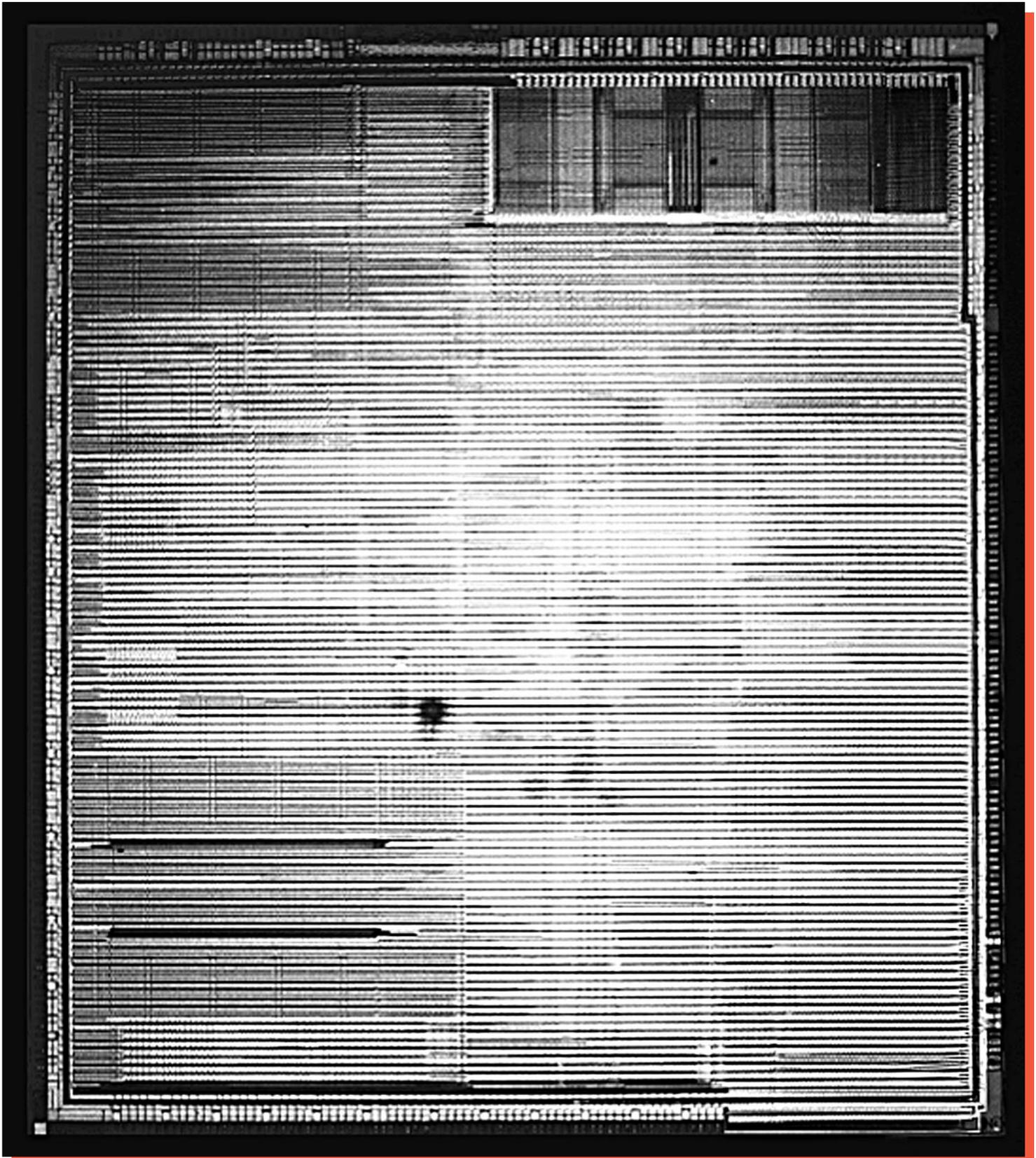
Figure 3. Whole die photograph of the Intel Pentium with MMX. Mag. 16x.
