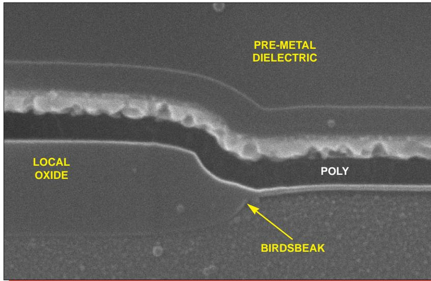
Figure 19. SEM section view of a local oxide birdsbeak. Mag. 52,000x.
