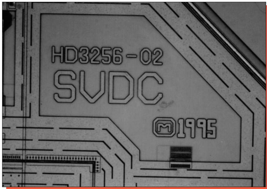
Figure 2. Markings from the die surface. Mag. 320x.
