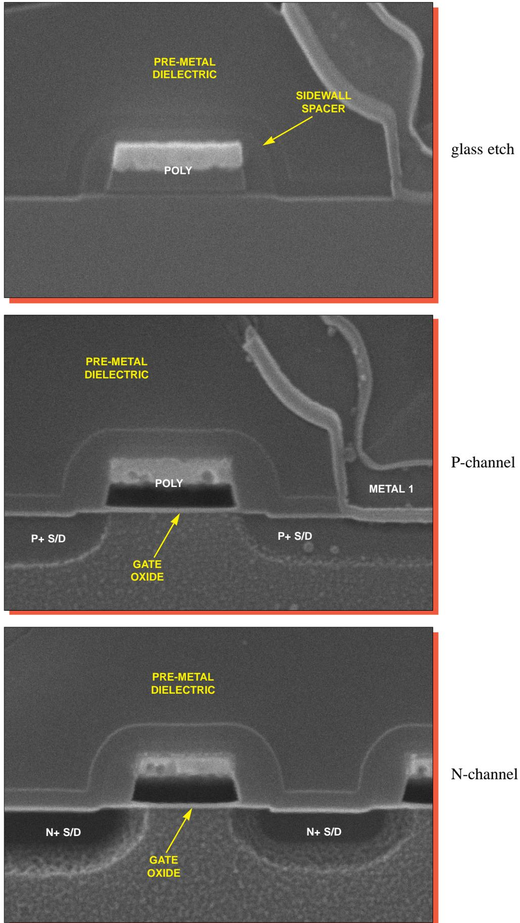
Figure 18. SEM section views of typical transistors. Mag. 52,000x.
