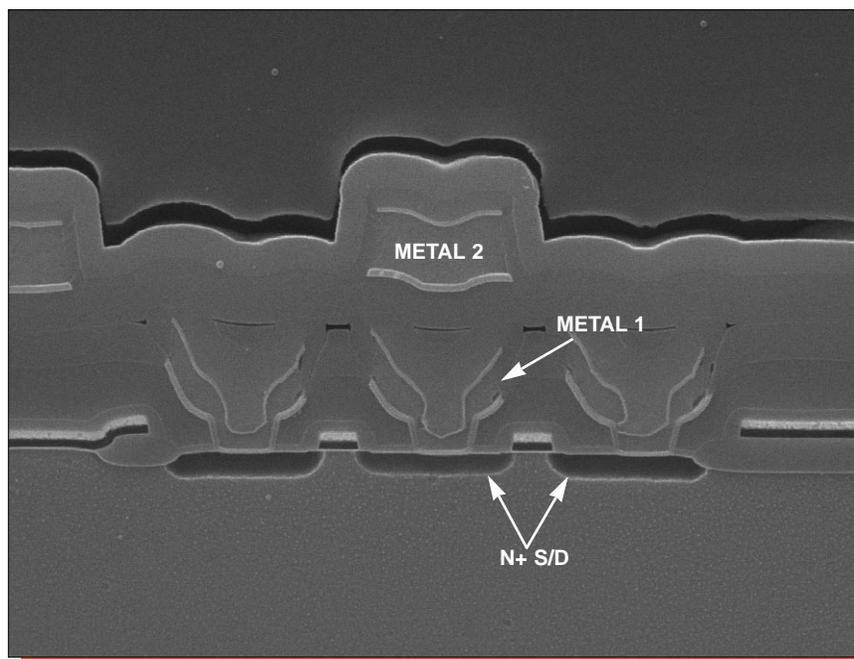
Figure 6. SEM section views of general device structure. Mag. 10,000x.
