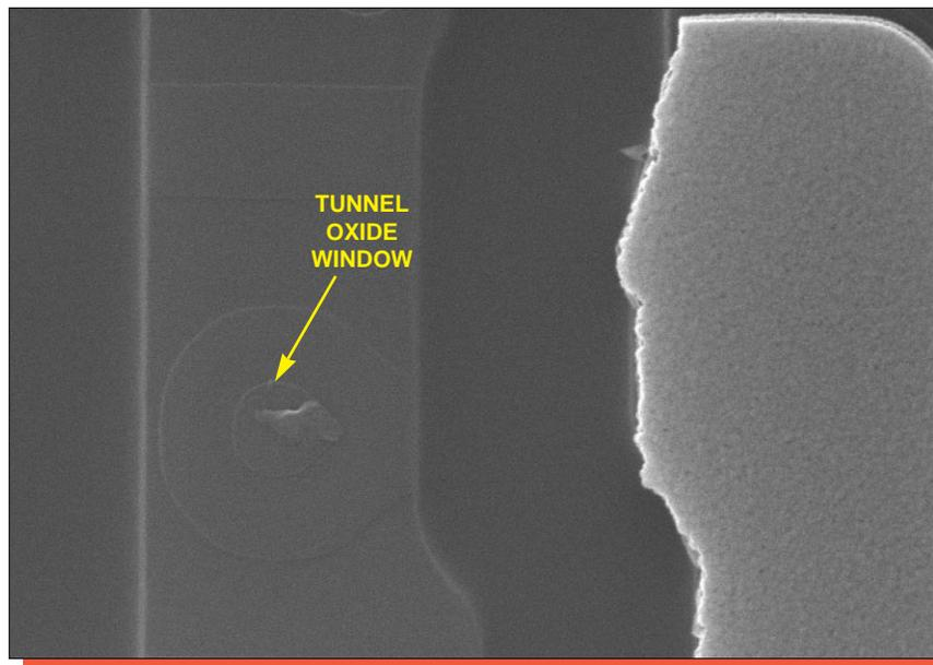
Figure 27. Topological SEM view of the tunnel oxide window. Array A,
