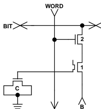
Figure 26. SEM view and schematic of the EEPROM cell. Array A, Mag. 3200x, 0°.
