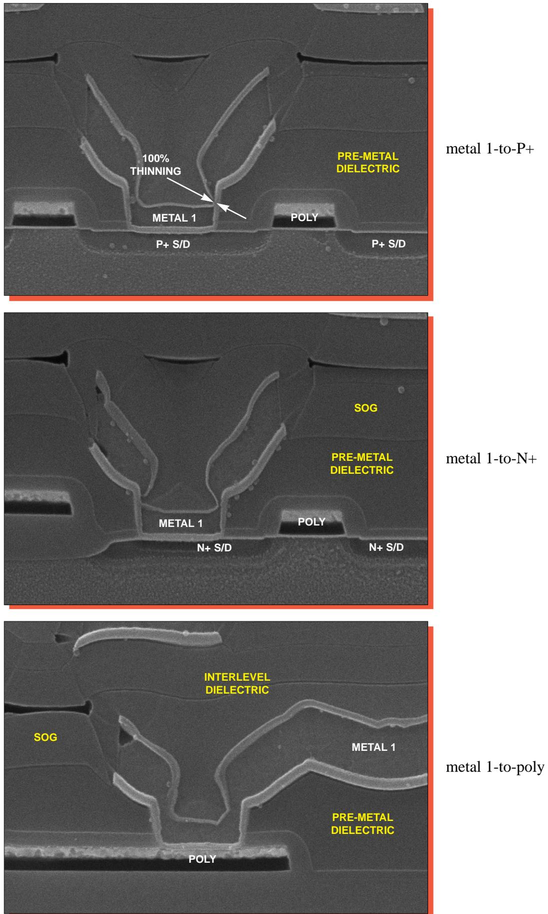
Figure 15. SEM section views of typical metal 1 contacts. Mag. 26,000x.
