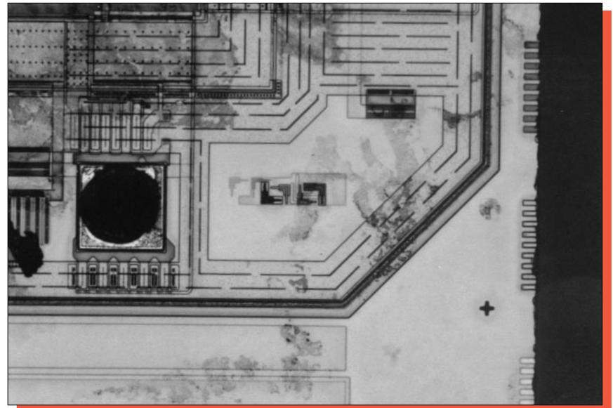
Figure 3. Optical views of the die corners on the Lattice 3256A-90LM. Mag. 160x.
