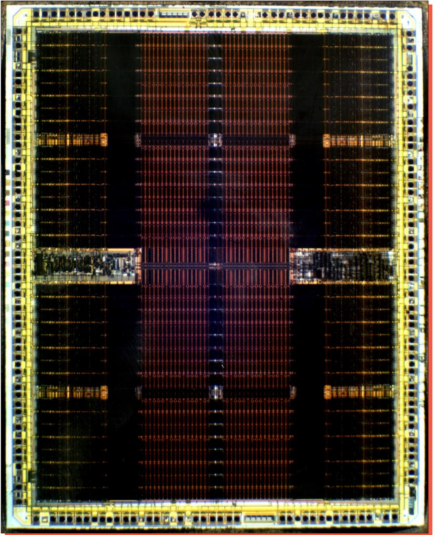
Figure 1. Whole die photograph of the Lattice 3256A-90LM. Mag. 25x.
