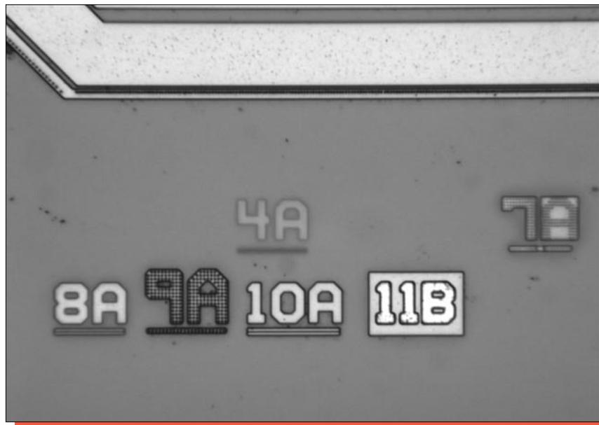
Figure 10. Optical views illustrating a slotted bus line and resolution patterns.
