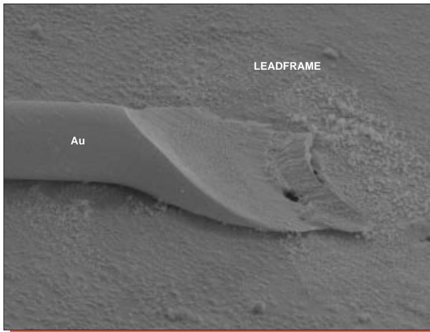
Figure 3. SEM views of typical wire bonding. Mag. 620x, 60°.
