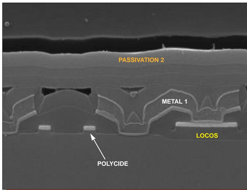
Figure 10. SEM section views illustrating general structure. Mag. 13,000x.
