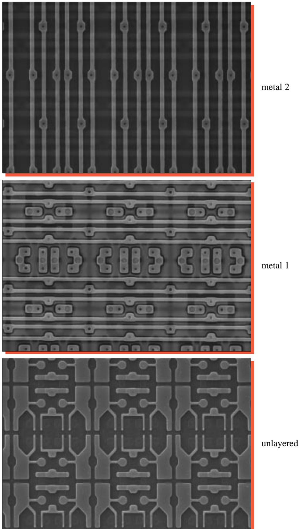
Figure 26. Topological SEM views illustrating the EEPROM cell array.
