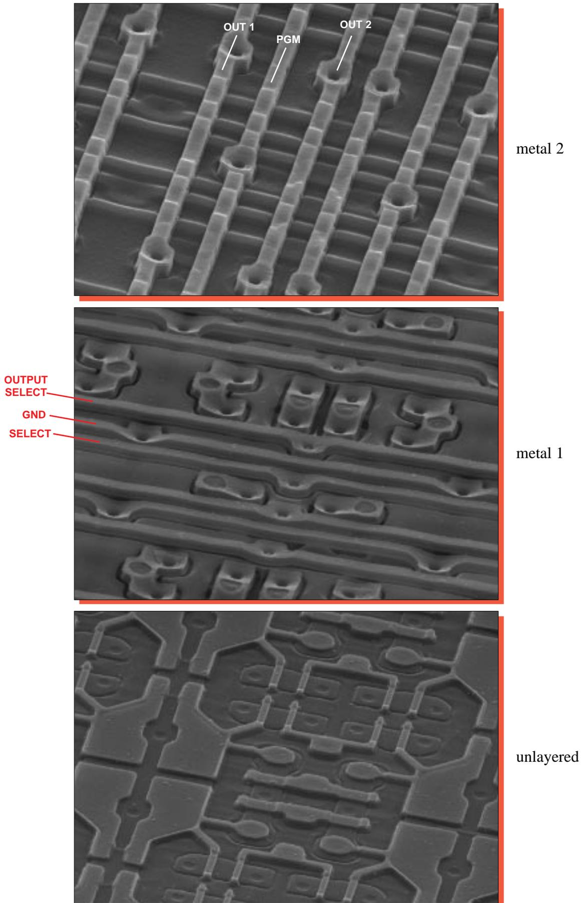
Figure 27. Perspective SEM views illustrating the EEPROM cell array.
