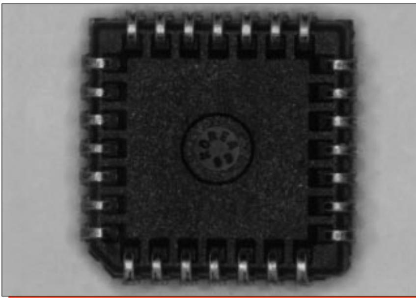
Figure 1. Package photographs and pinout of the Lattice GAL22LV10D PLD.
