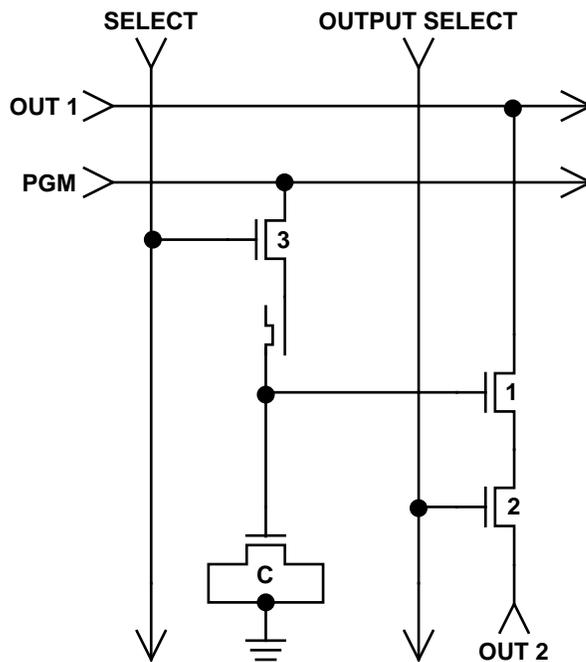
Figure 30. Topological SEM view and schematic of the EEPROM cell.
