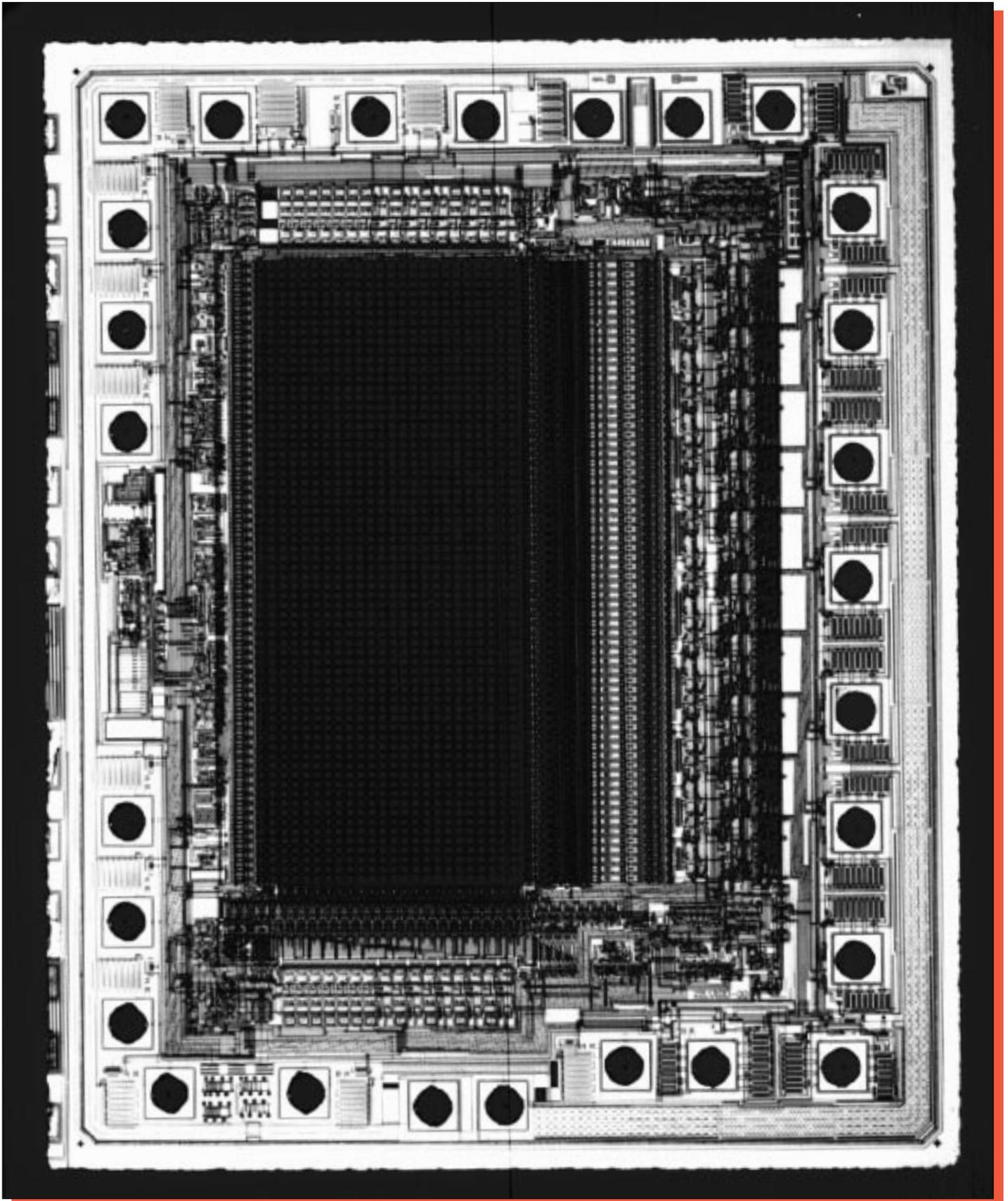
Figure 6. Whole die photograph of the Lattice GAL22LV10D. Mag. 75x.
