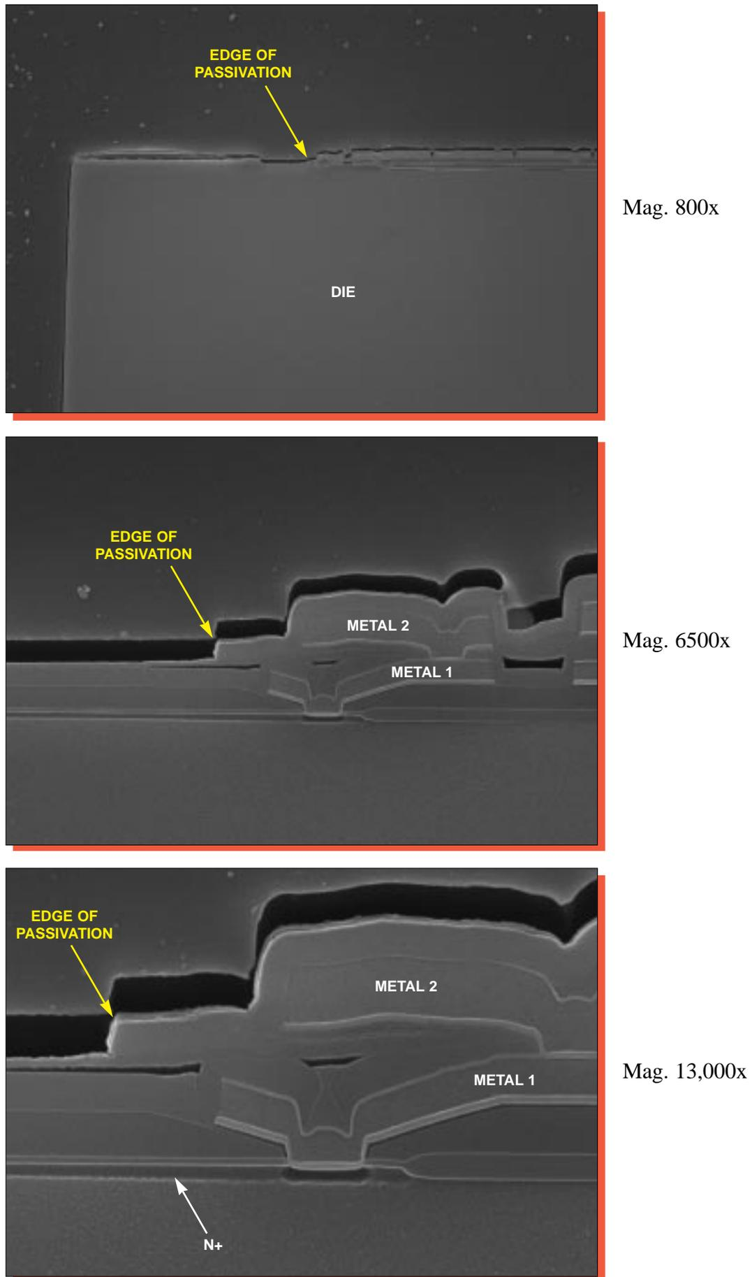
Figure 5. SEM section views of the edge seal.
