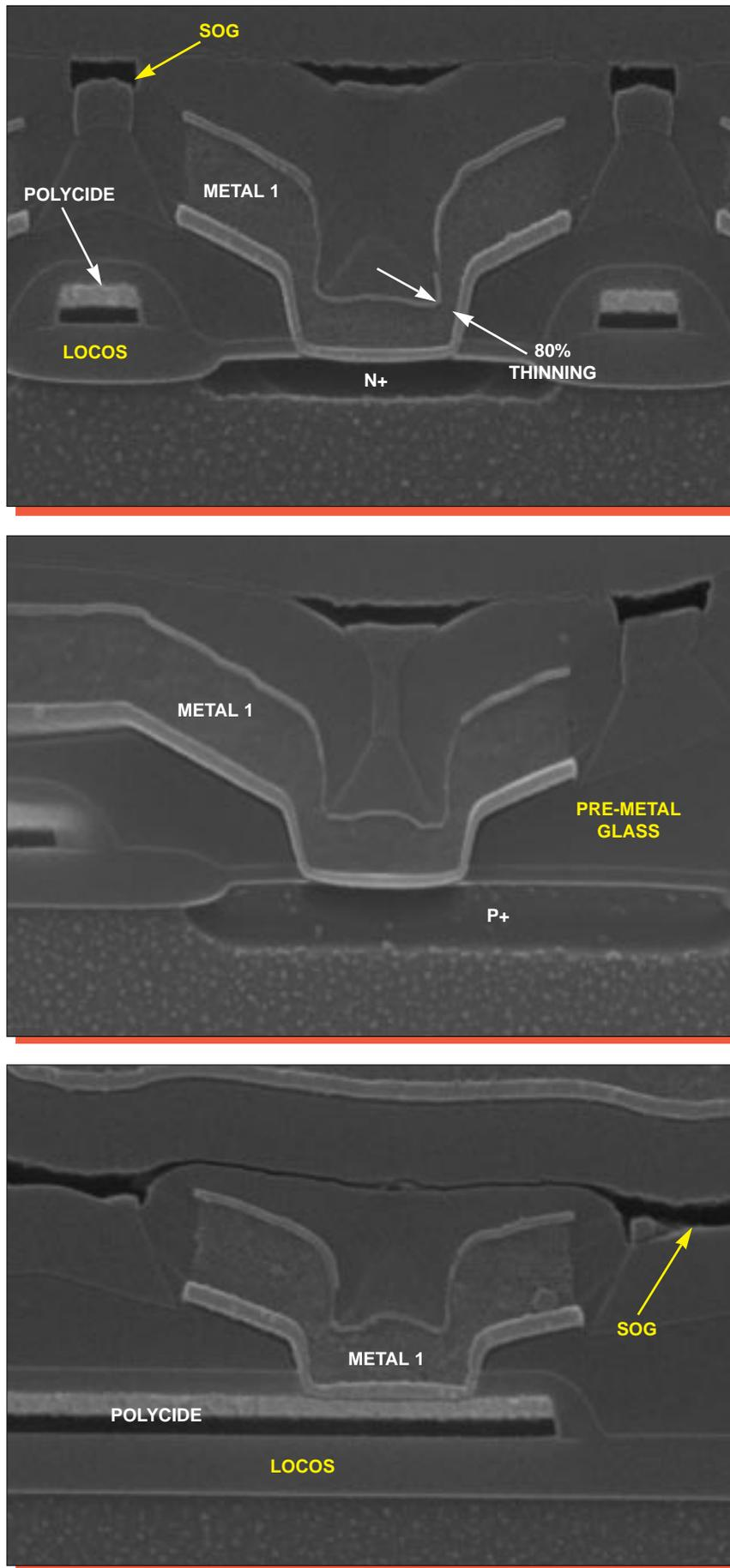
Figure 19. SEM section views of typical metal 1 contacts. Mag. 26,000x.
