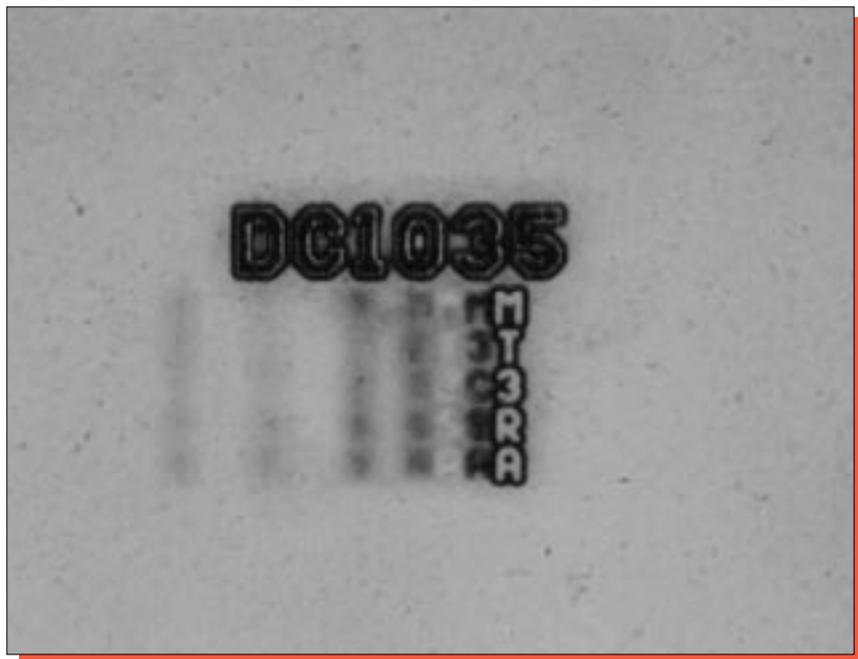
Figure 8. Die identification markings. Mag. 800x.
