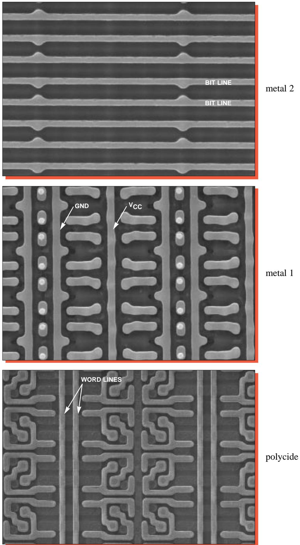
Figure 37. Topological SEM views of the Cache array. Mag. 5000x, 0°.
