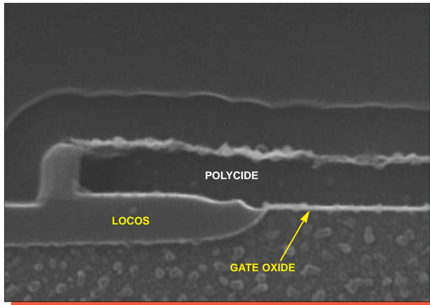
Figure 34. SEM section view of a local oxide birdsbeak. Mag. 50,000x.
