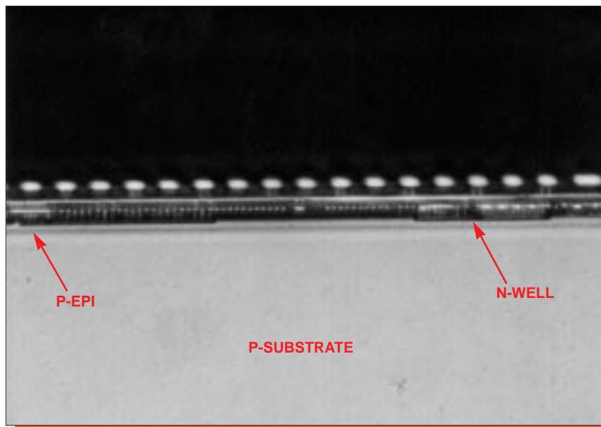
Figure 35. Optical view of the well structure. Mag. 800x.
