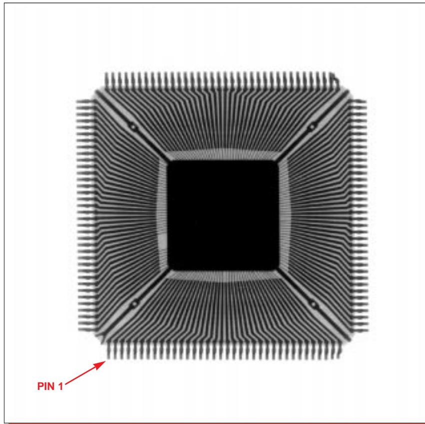
Figure 1. Package photograph and x-ray view of the DEC SA-110S StrongARM.
