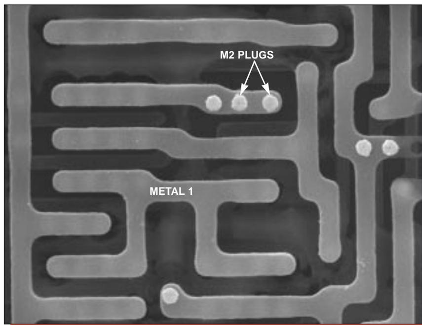
Figure 23. Topological SEM views of metal 1 patterning. Mag. 8000x, 0°.
