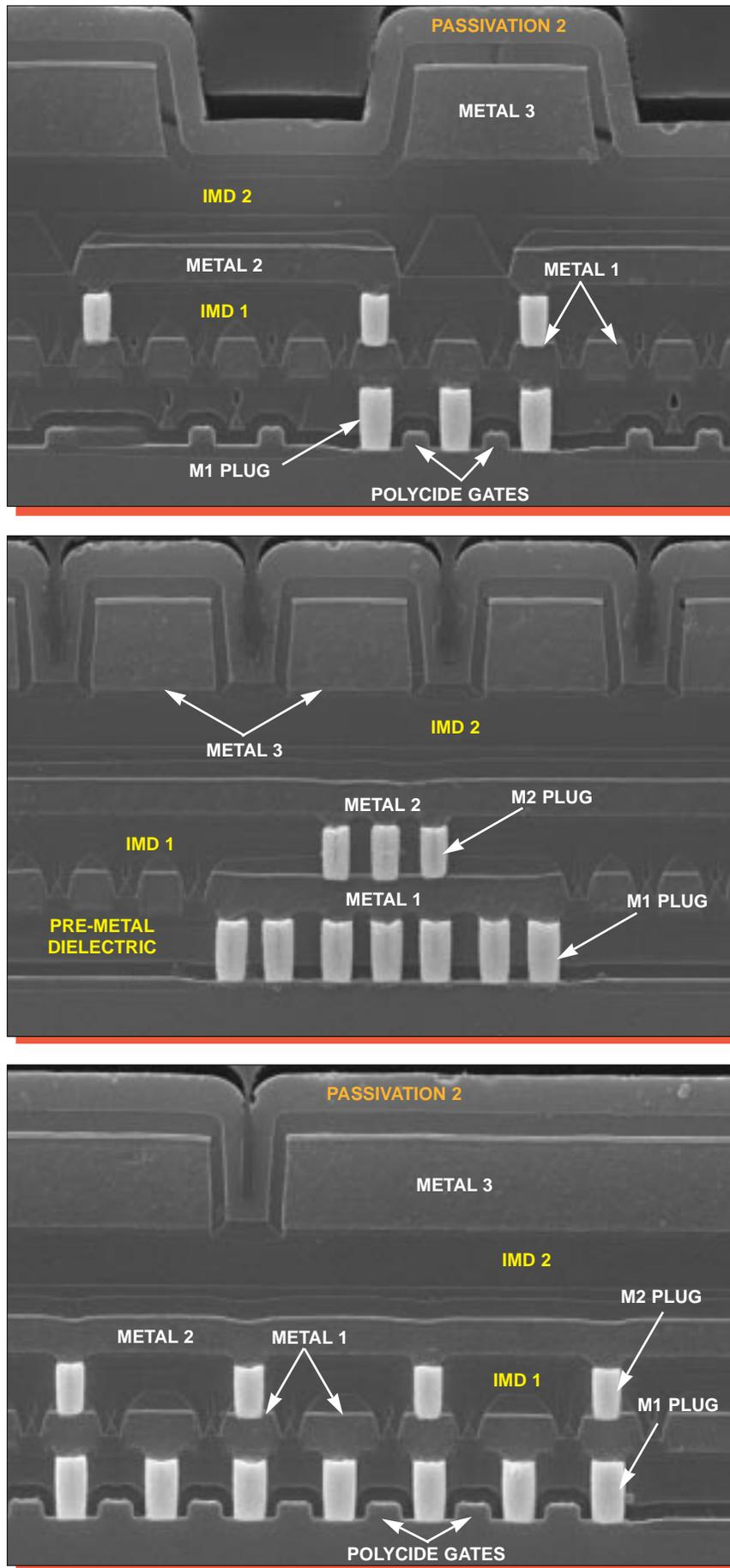
Figure 11. Glass etch section views illustrating general structure. Mag. 9000x.
