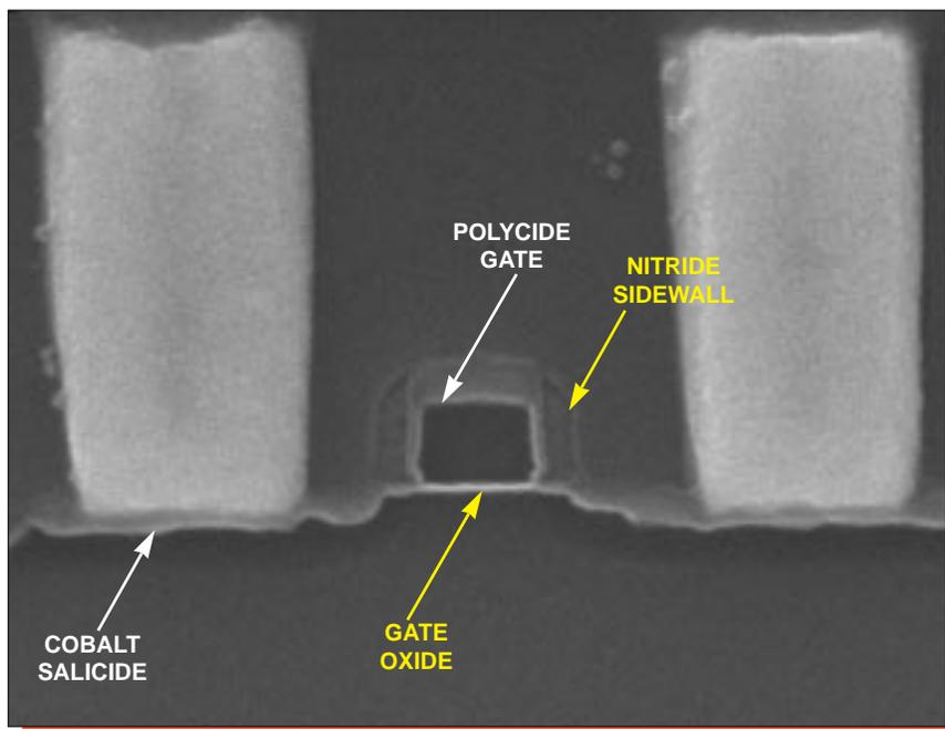
Figure 33. SEM section views of typical transistors. Mag. 52,000x.
