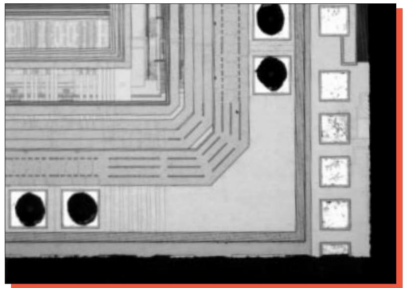
Figure 9. Optical views of the die corners. Mag. 100x.
