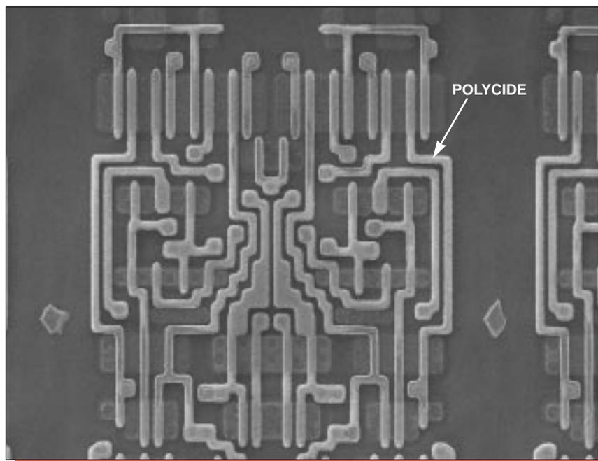
Figure 30. Topological SEM views of polycide in the decode areas. Mag. 3500x, 0°.
