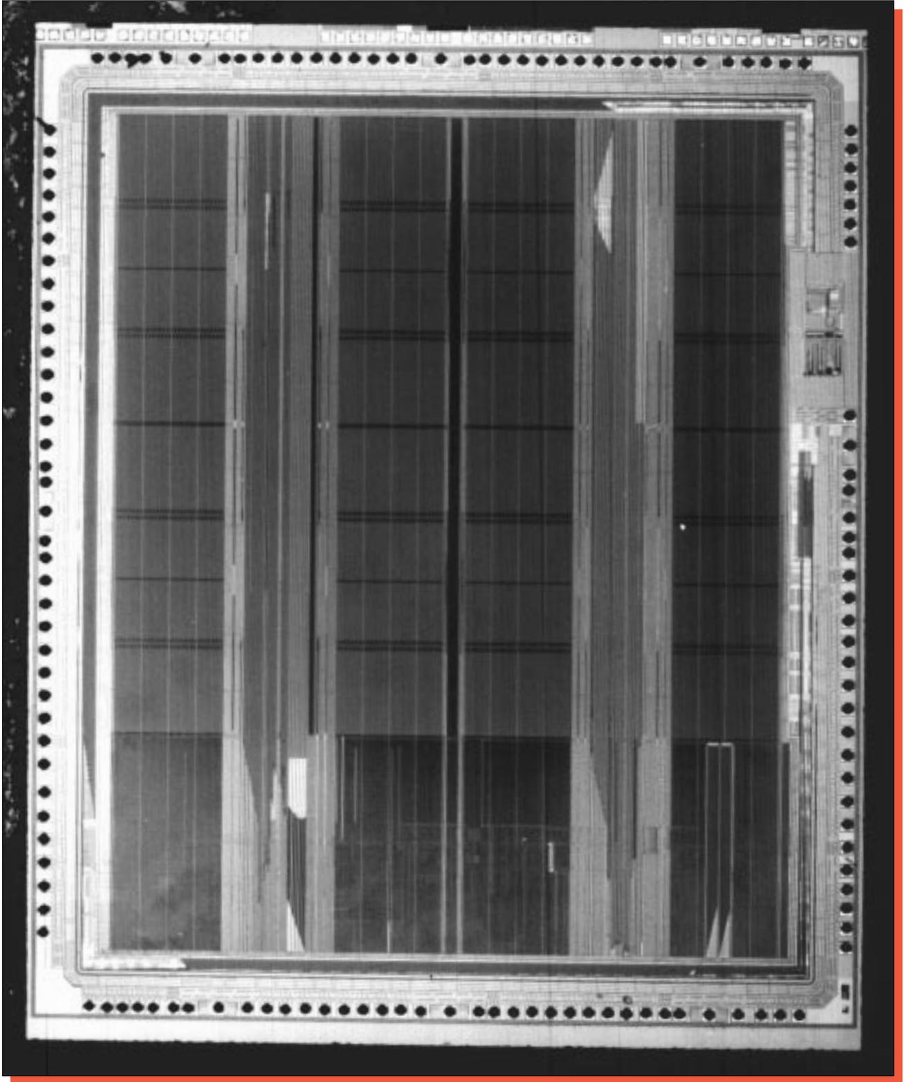
Figure 7. Whole die photograph of the DEC SA-110S StrongARM. Mag. 25x
