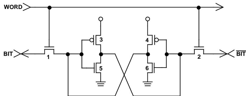
Figure 40a. Topological SEM view of Cache SRAM cells along with the cell schematic.
