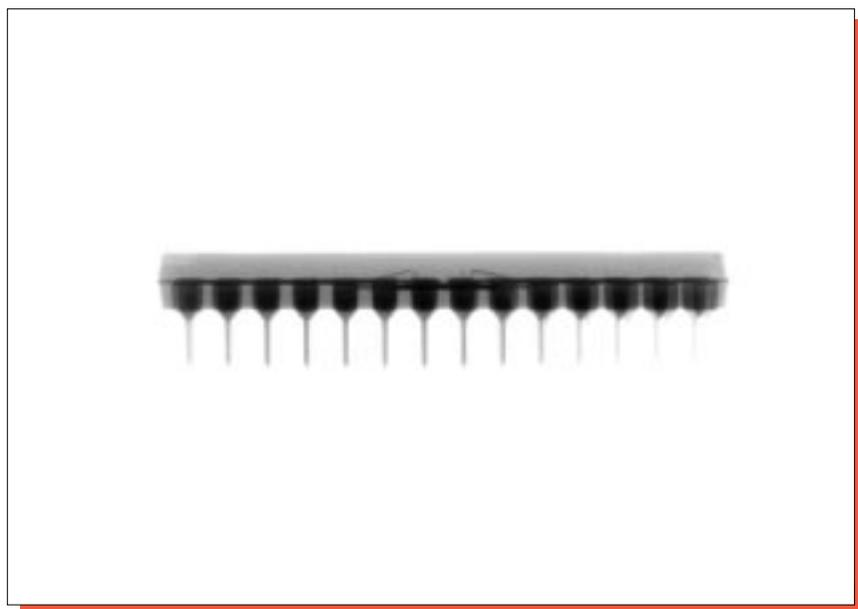
Figure 4. X-ray views of the 256K Flash package. Mag. 2x.
