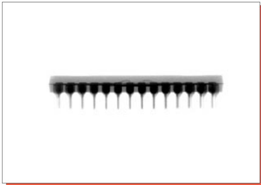
Figure 3. X-ray views of the 512K Flash package. Mag. 2x.
