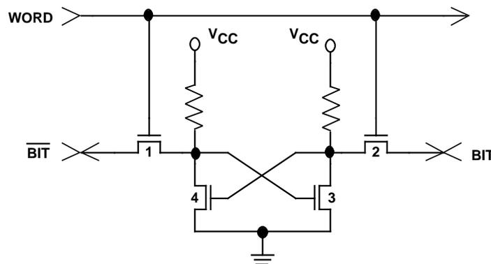
Figure 29. Detailed topological SEM views and schematic of the SRAM cell.
