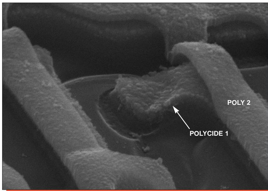
Figure 27. Detailed SEM views of the SRAM cell at poly. Mag. 30,000x, 60°.
