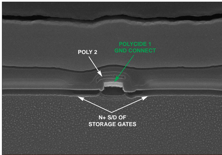
Figure 31. Additional SEM section views of the SRAM cell array.
