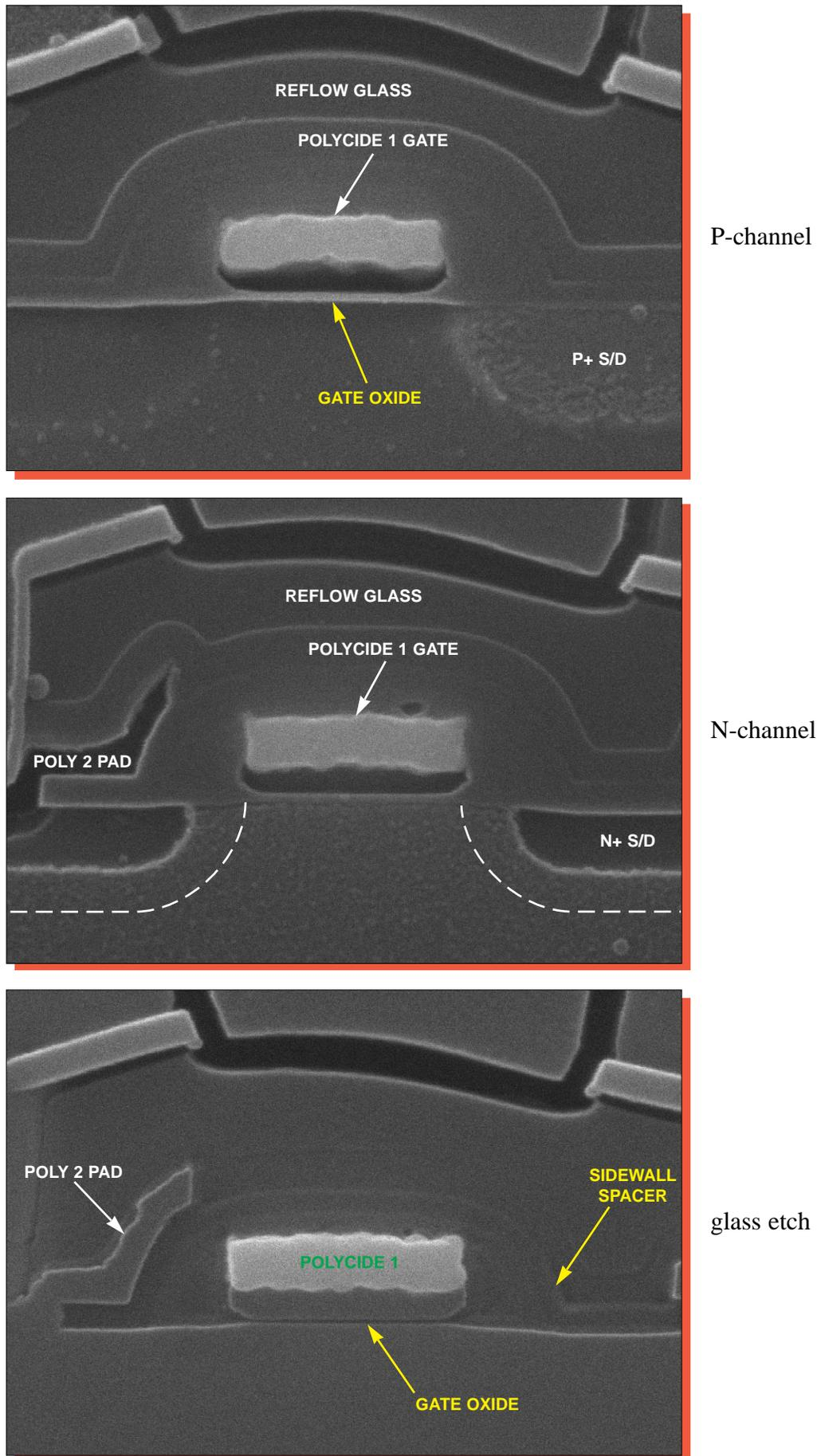
Figure 19. SEM section views of typical transistors. Mag. 52,000x.
