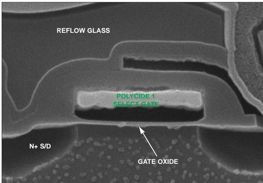
Figure 30. SEM section views of the SRAM cell array.
