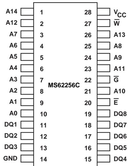
Figure 1. Package photographs and pinout of the Mosel Vitelic MS62256CLL-70PC.
