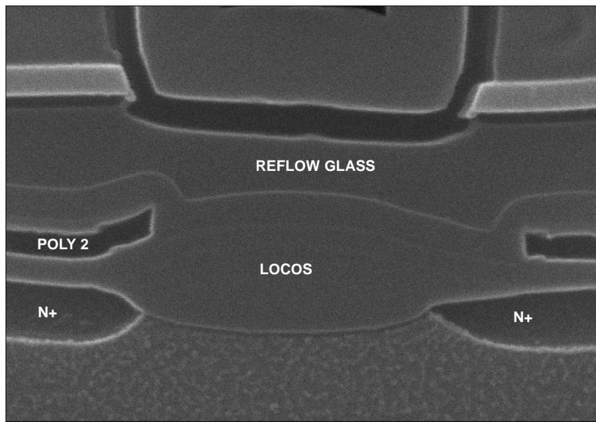
Figure 20. SEM section views illustrating a birdsbeak and field oxide isolation.
