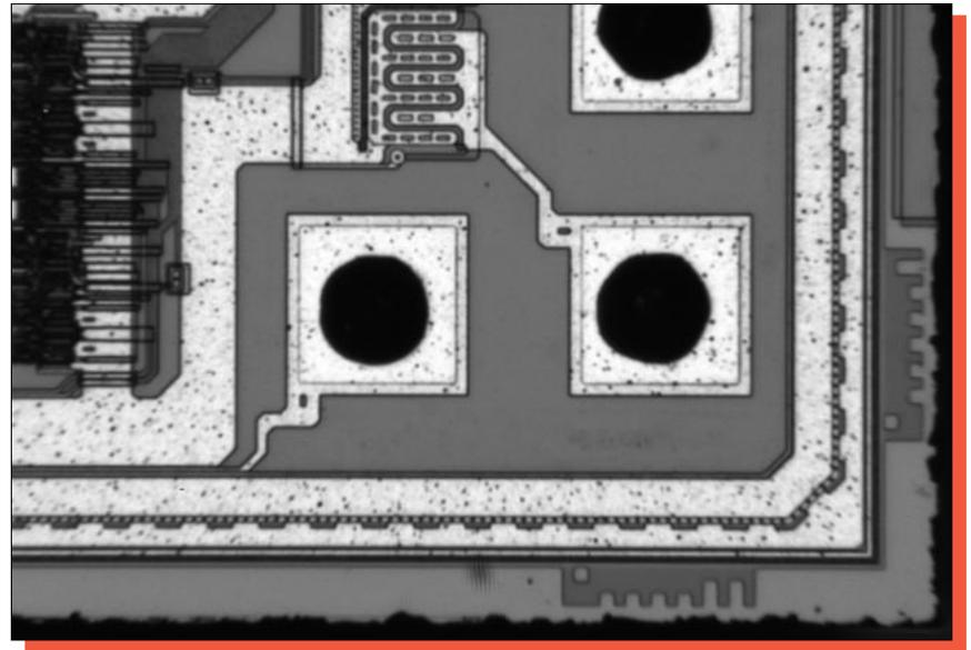
Figure 8. Optical views of die corners. Mag. 150x.
