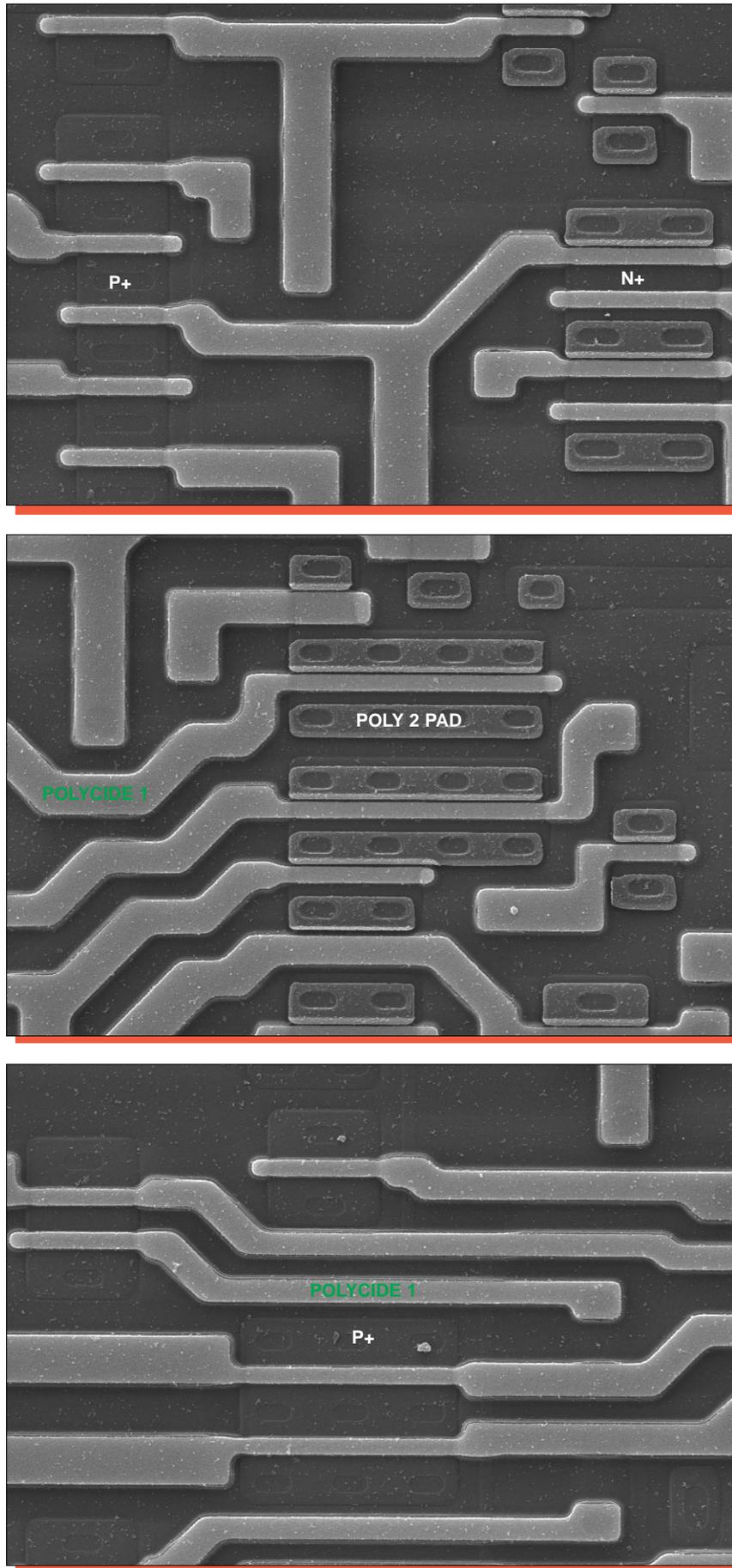
Figure 17. Topological SEM views of polycide 1 patterning. Mag. 3200x, 0°.
