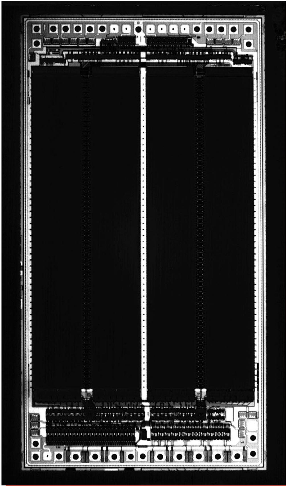
Figure 6. Whole die photograph of the Mosel Vitelic MS62256CLL-70PC. Mag. 32x.
