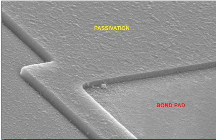
Figure 10. SEM view of a bond pad. Mag. 3000x, 60°.
