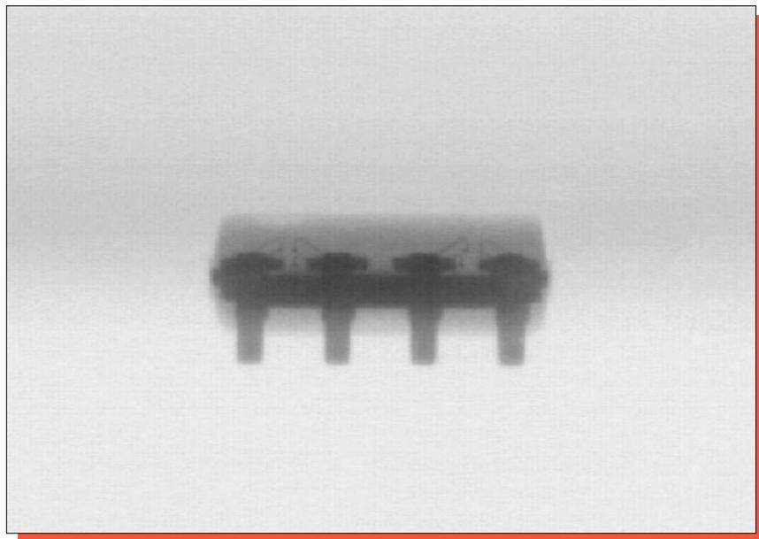
Figure 2. X-ray views of the Microchip 93LC86 16K Serial EEPROM. Mag 10x.
