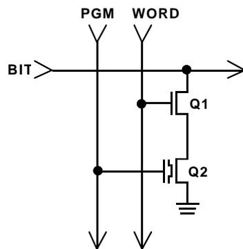
Figure 31. Topological SEM views illustrating EEPROM cell array and schematic.
