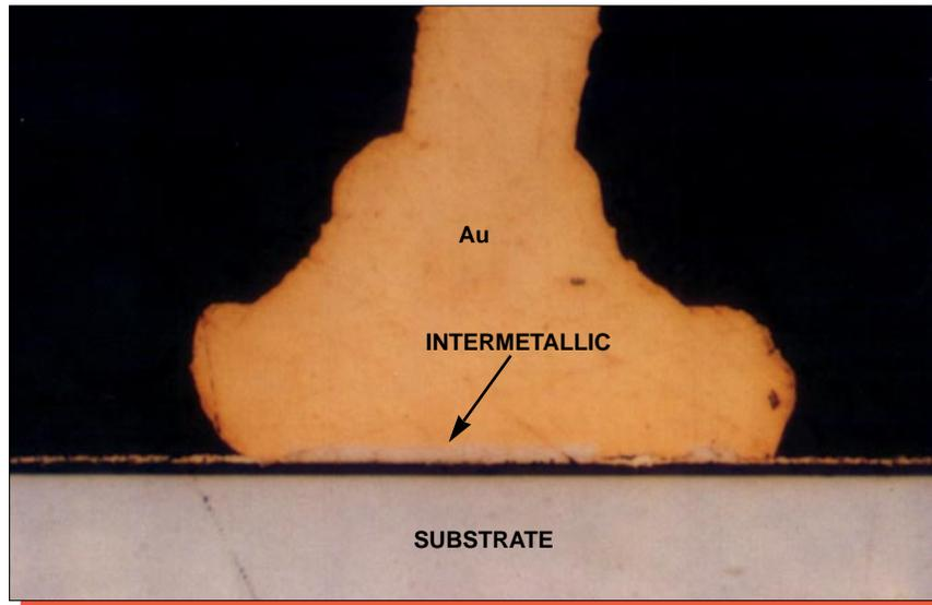
Figure 8. Optical section view of a ball bond. Mag 800x.
