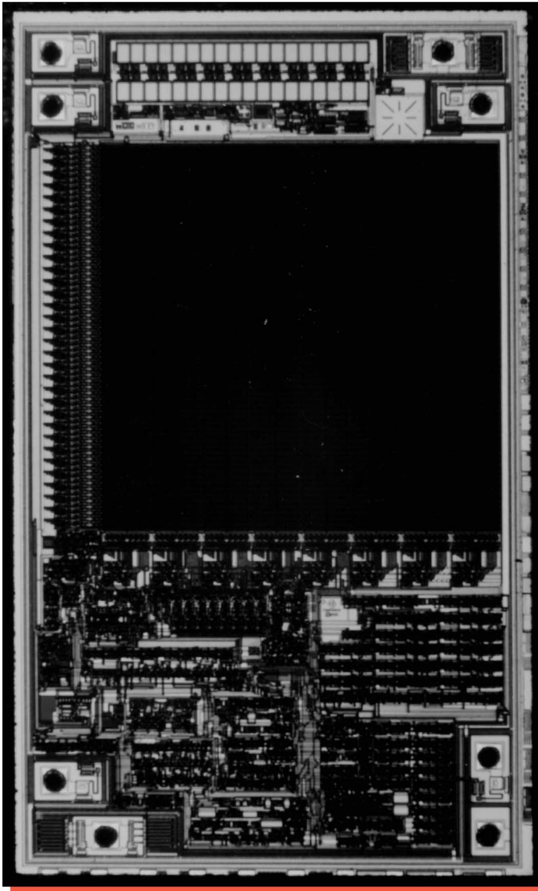
Figure 12. Whole die photograph of the Microchip 93LC86 16K Serial EEPROM.
