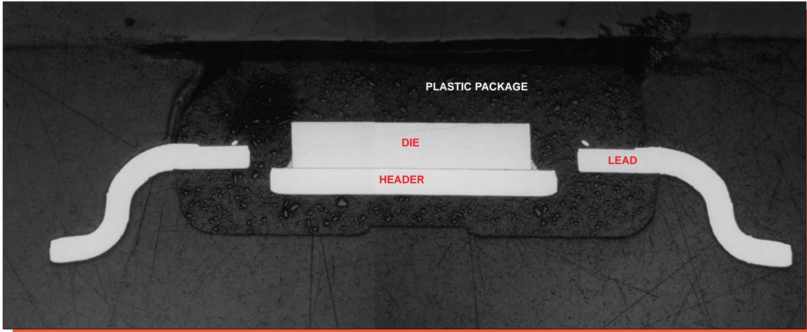
Figure 3. Optical section view of general package construction. Mag. 30x.
