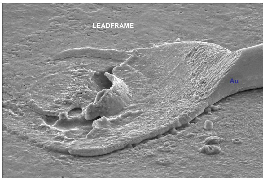
Figure 9. SEM views of typical wirebonds. Mag. 700x, 60°.
