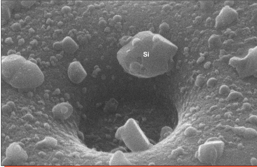
Figure 20. SEM view illustrating a contact cut. Mag. 24,000x.
