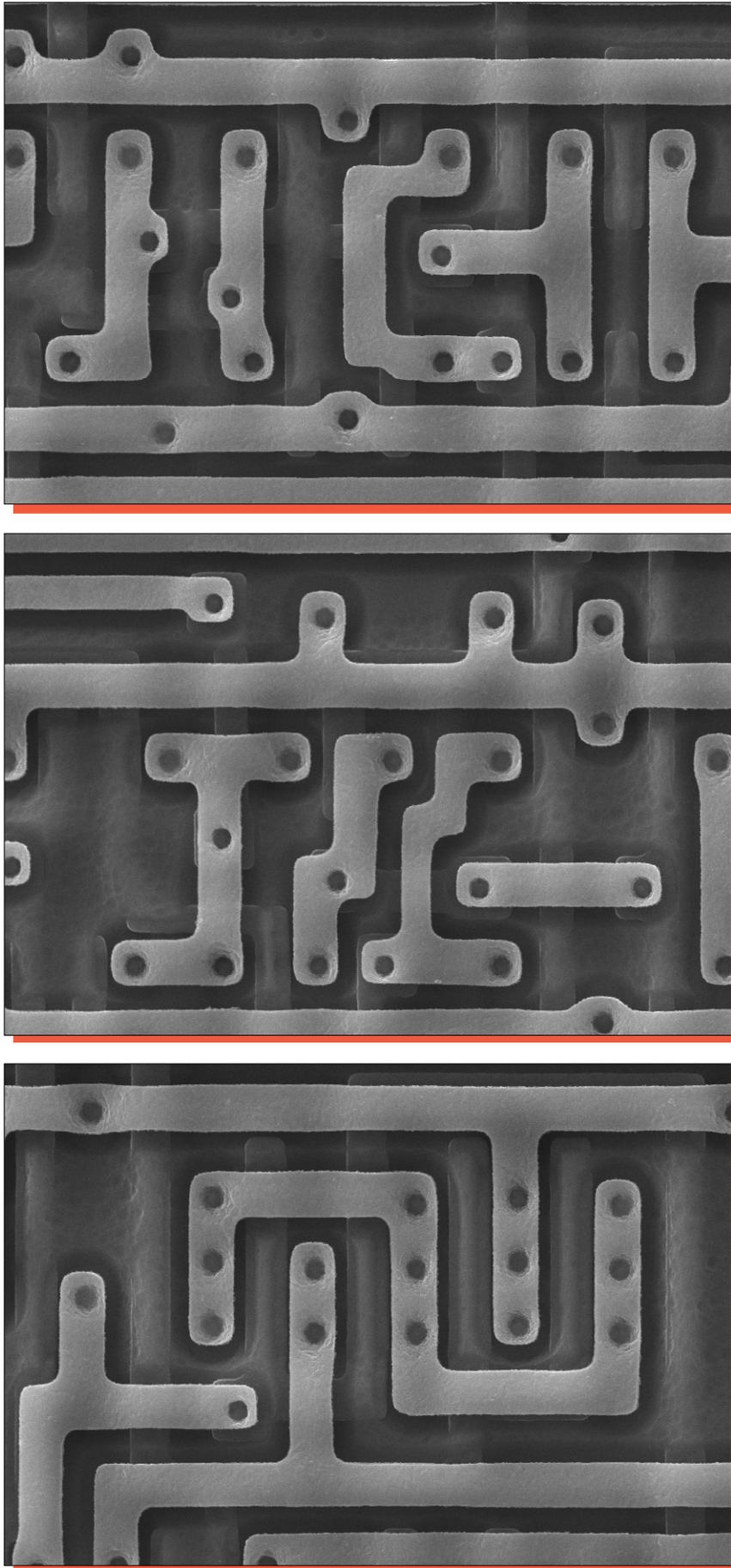
Figure 17. Topological SEM views of metal patterning. Mag. 24,000x, 0°.
