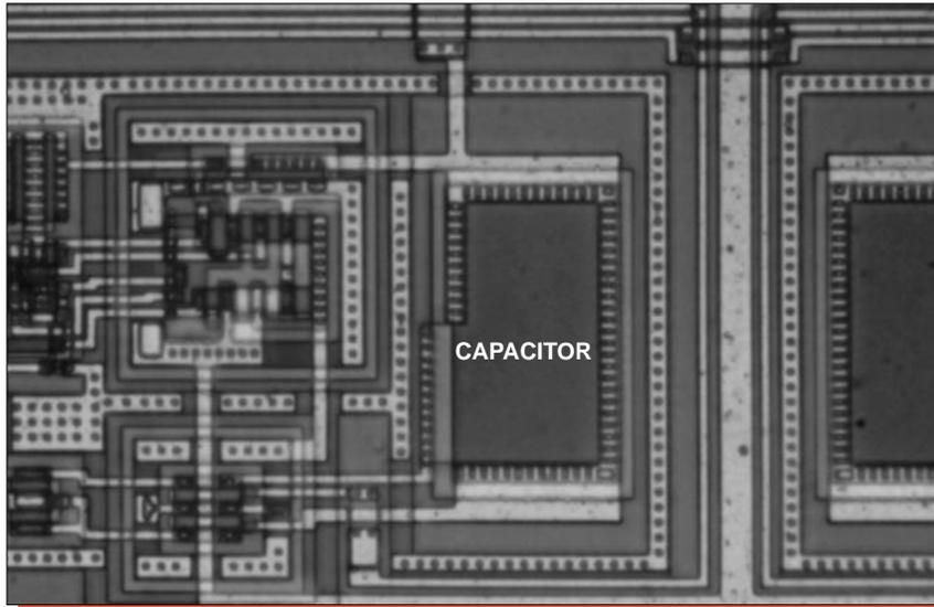
Figure 20. Optical view of a typical capacitor. Mag. 400x.
