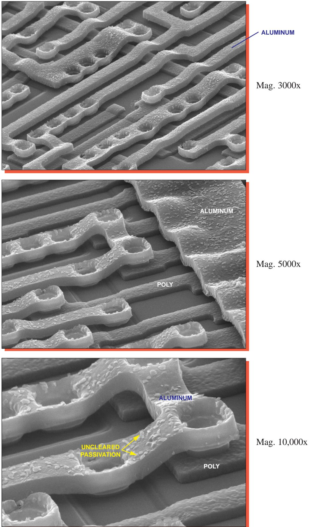
Figure 7. SEM views illustrating metal step coverage. 60°.
