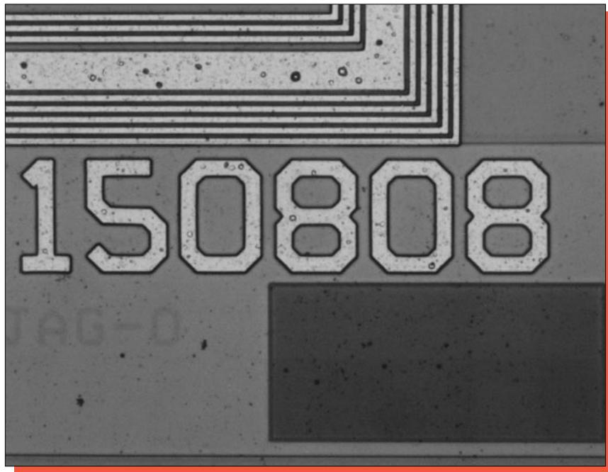
Figure 3. Die identification markings. Mag. 500x.
