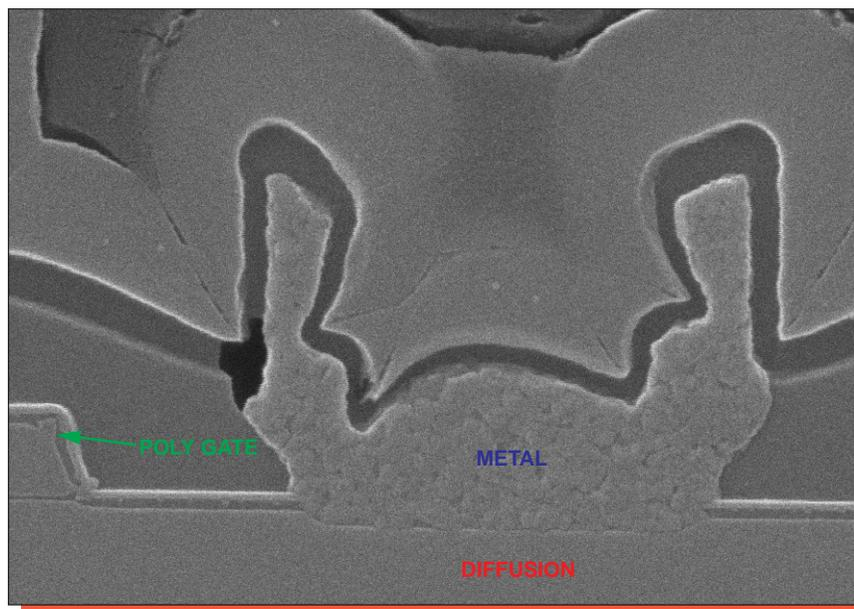
Figure 9b. SEM details of contacts. Glass etch, Mag. 26,000x.
