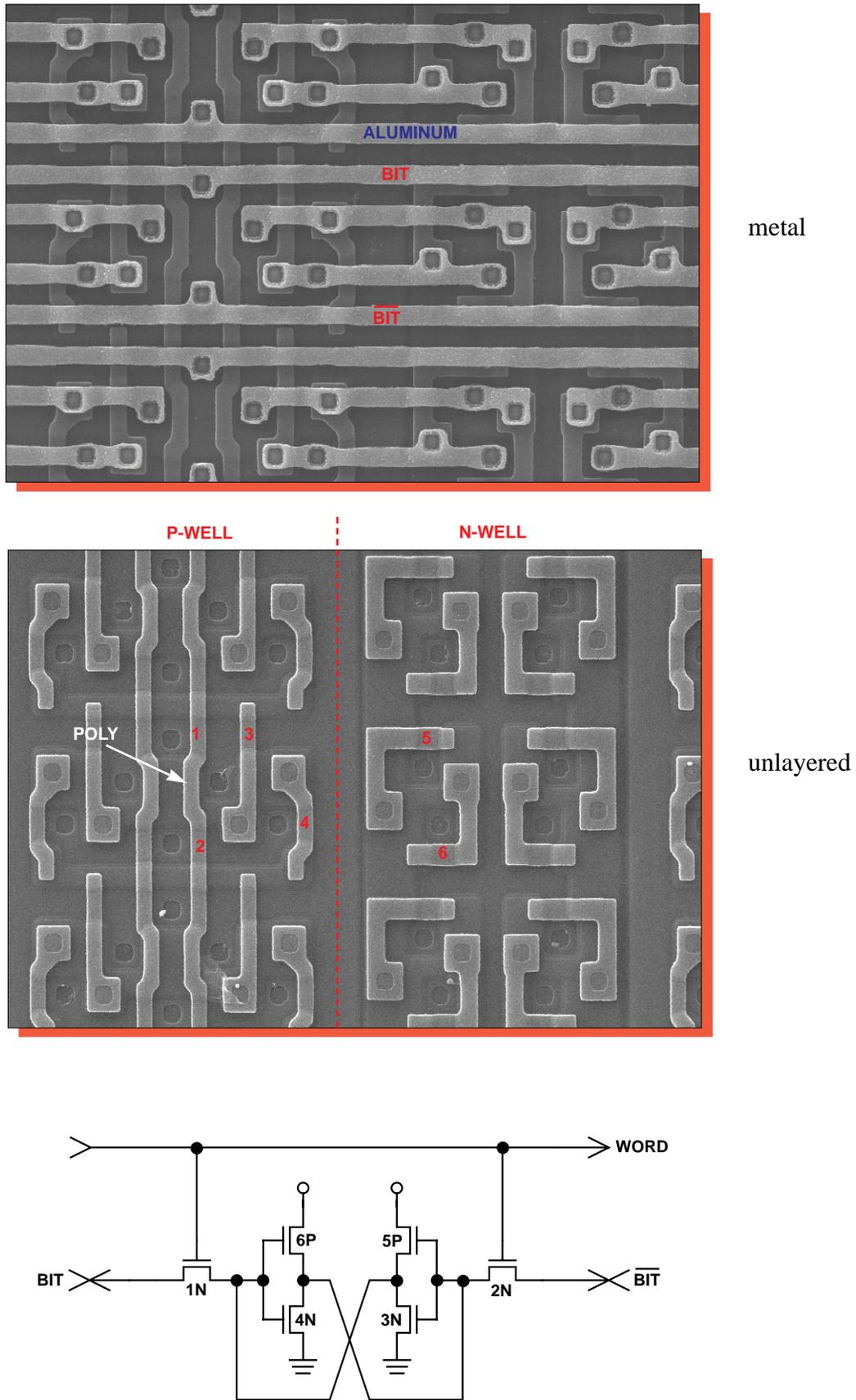
Figure 18b. Topological SEM view illustrating 6T SRAM cell array along with schematic. Mag. 1500x, 0°.
