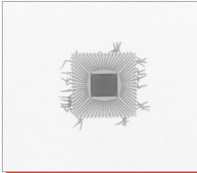
Figure 1. Package photograph and x-ray view of the Panasonic MN150808KJAG.
