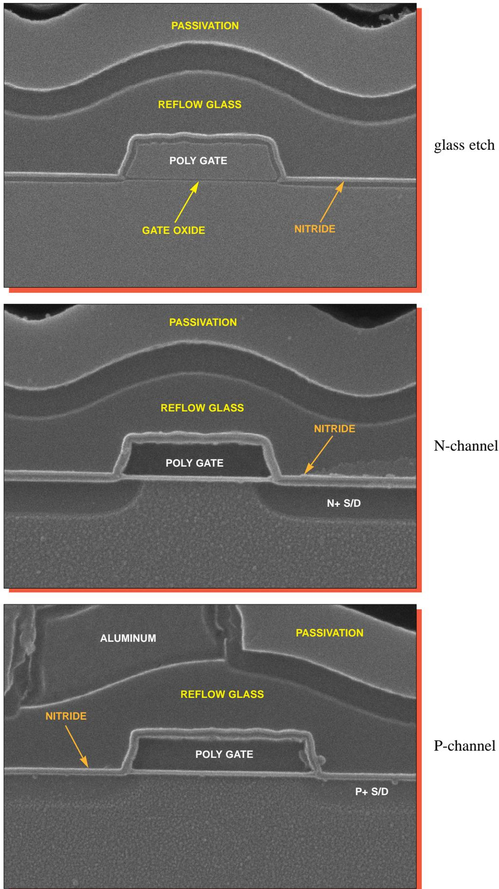
Figure 13. SEM views illustrating typical gate structures. Mag. 26,000x.
