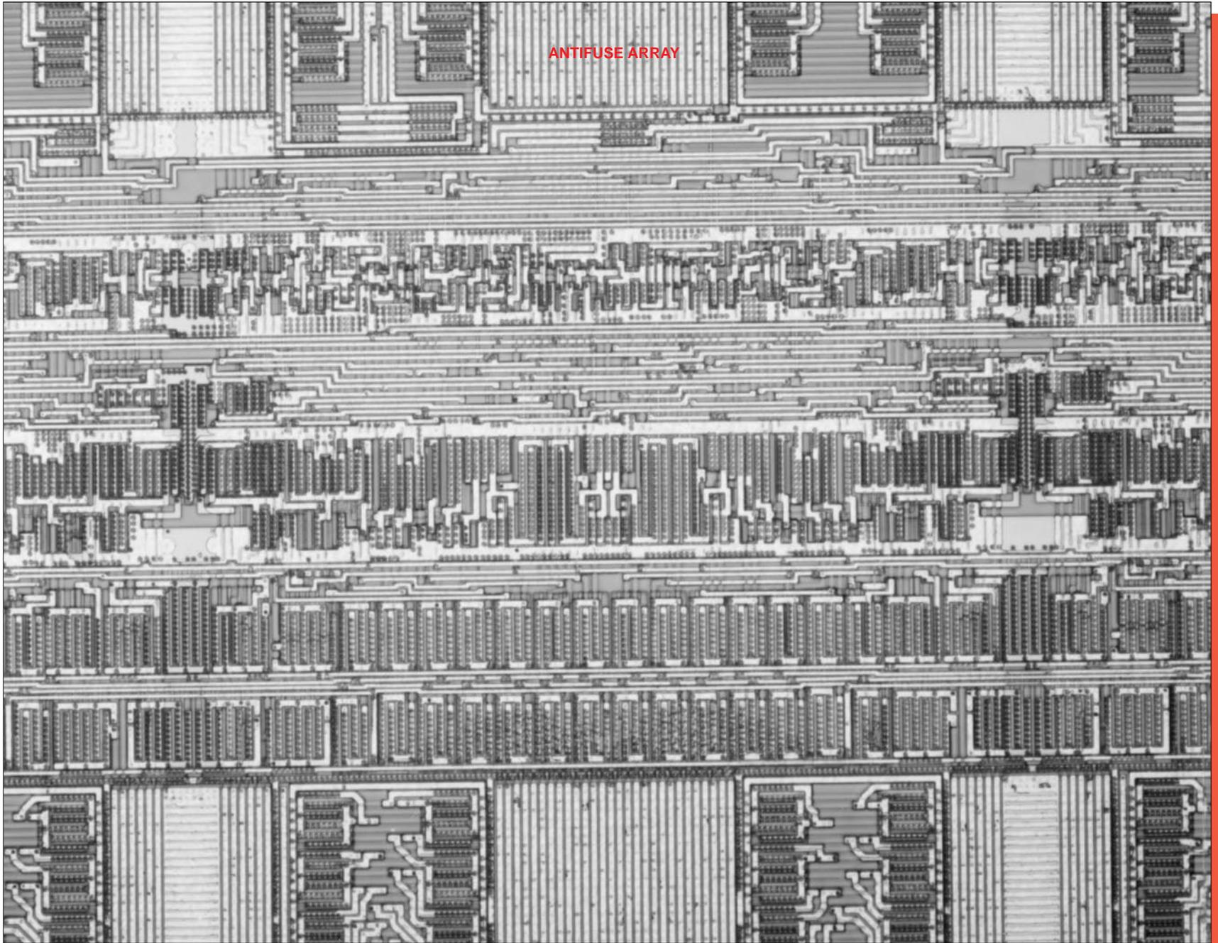
Figure 21a. Optical view of typical device circuitry. Metal 1, Mag. 520x.
