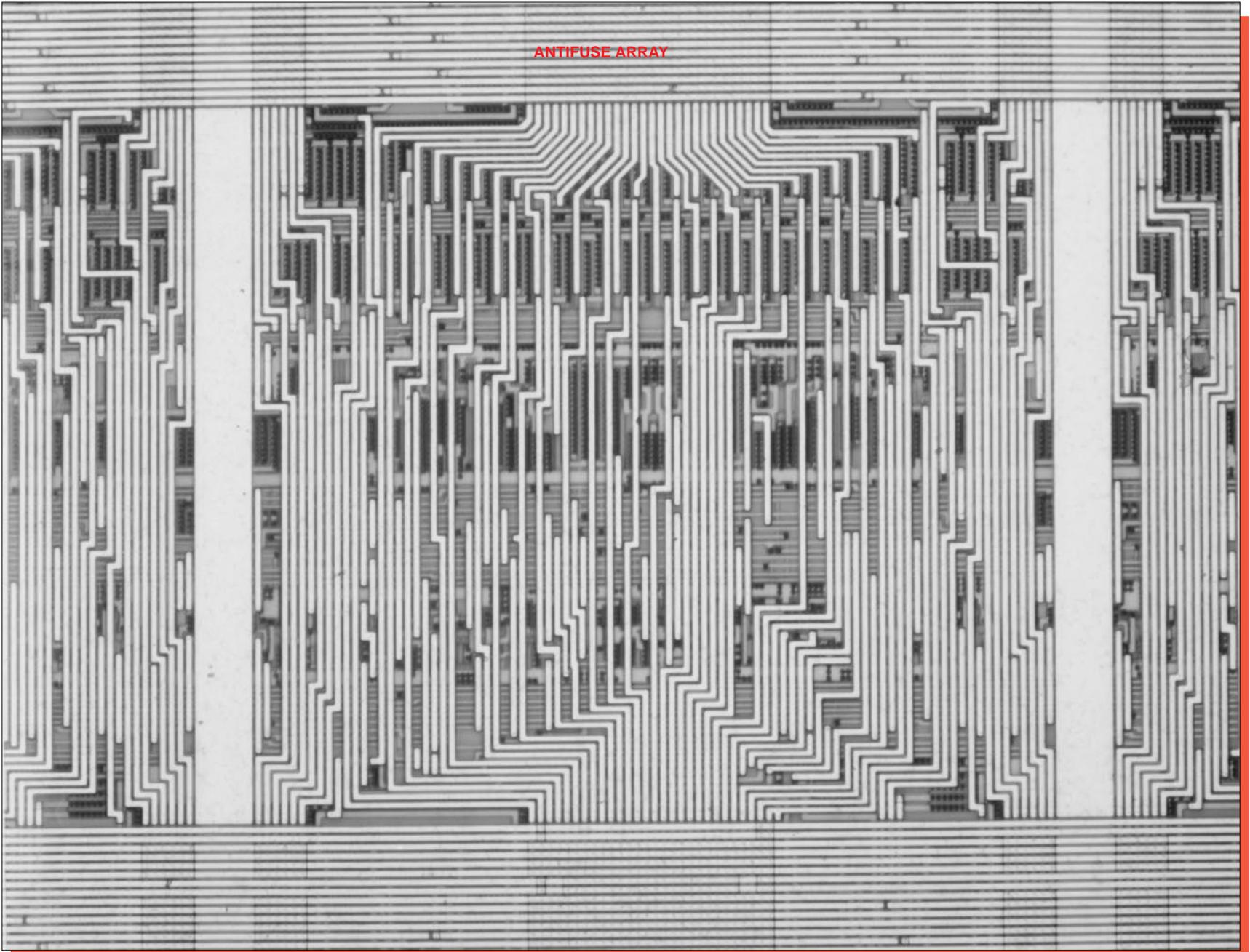
Figure 21. Optical view of typical device circuitry. Metal 2, Mag. 520x.
