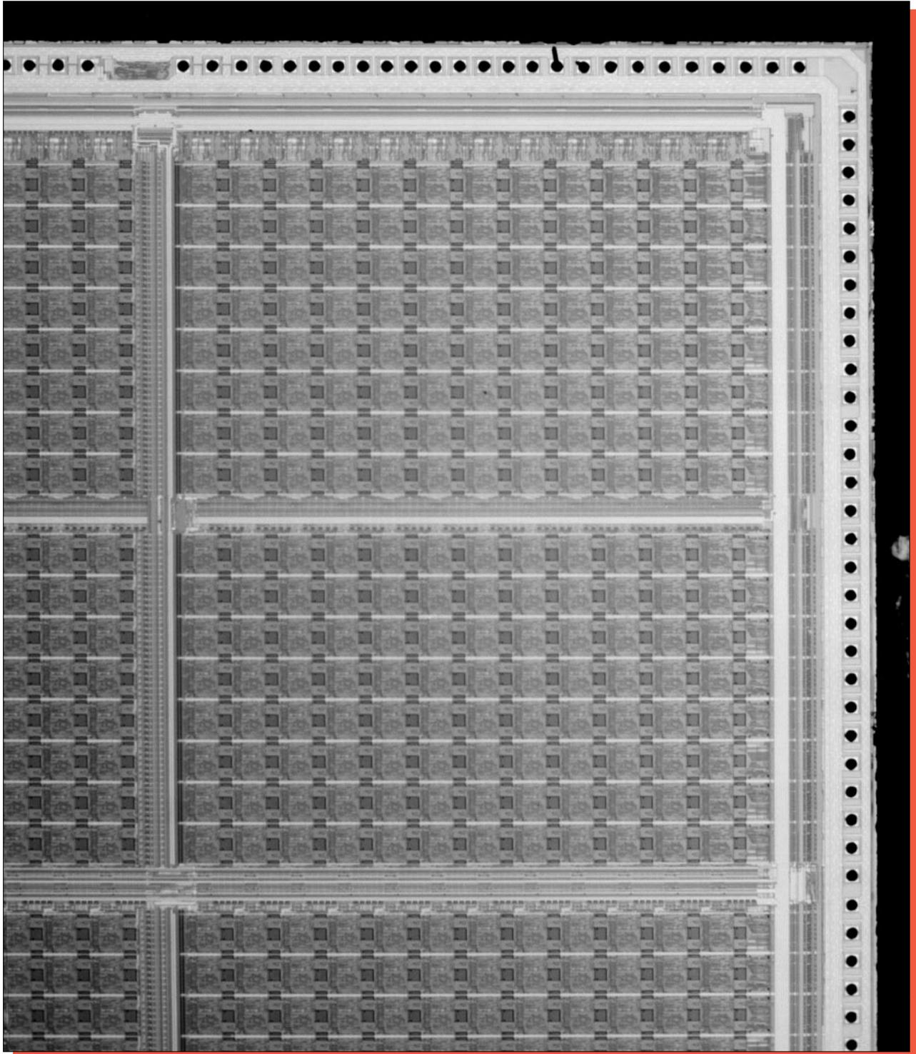
Figure 1c. Remaining portion of the QuickLogic 24X32 intact circuit die. Mag. 26x.
