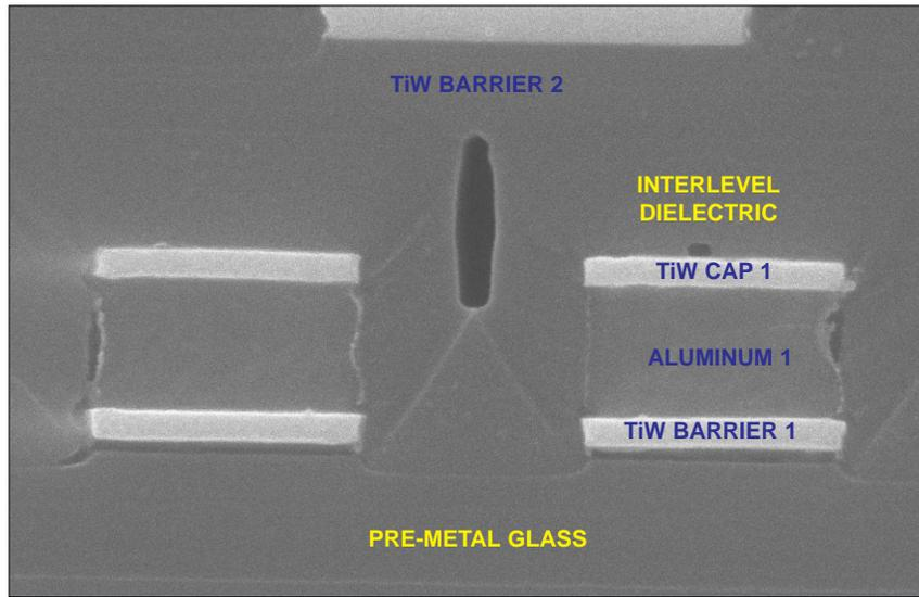
Figure 11. SEM section view of metal 1 line profiles. Mag. 26,000x.
