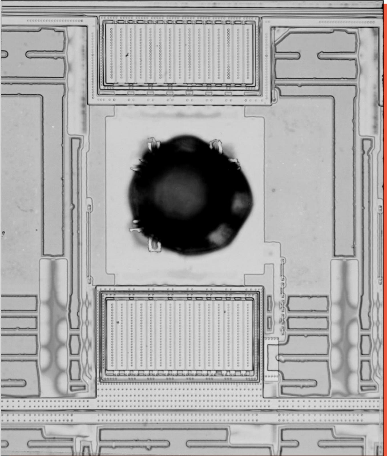
Figure 27. Optical view of the I/O layout. Poly, Mag. 640x.
