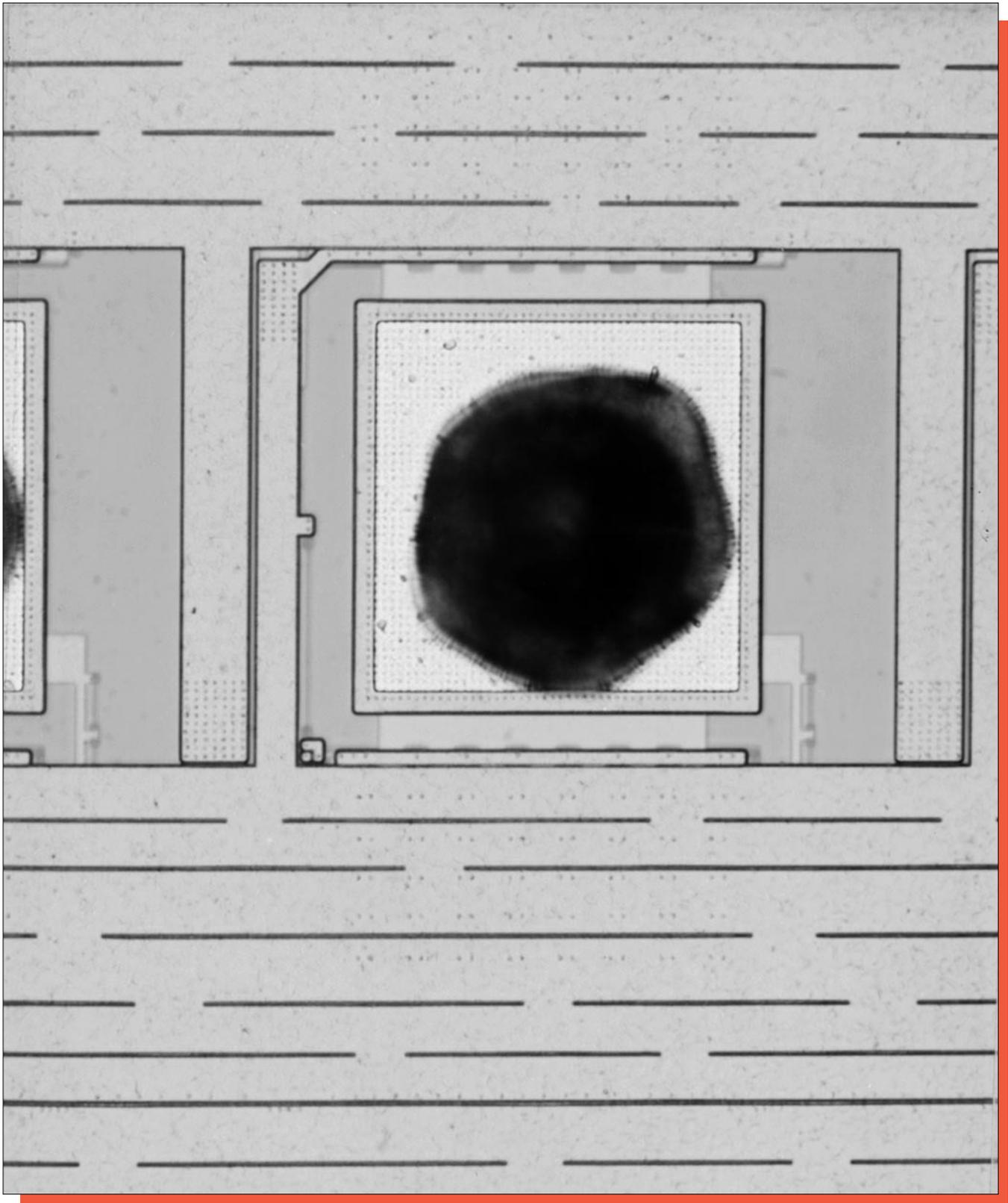
Figure 25. Optical view of the I/O layout. Metal 2, Mag. 640x.
