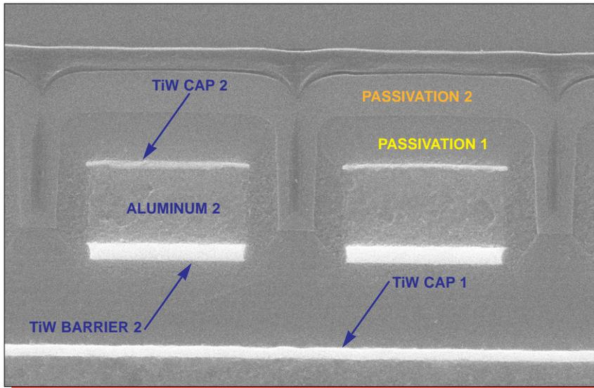
Figure 7. SEM section view of metal 2 line profiles. Mag. 16,000x.
