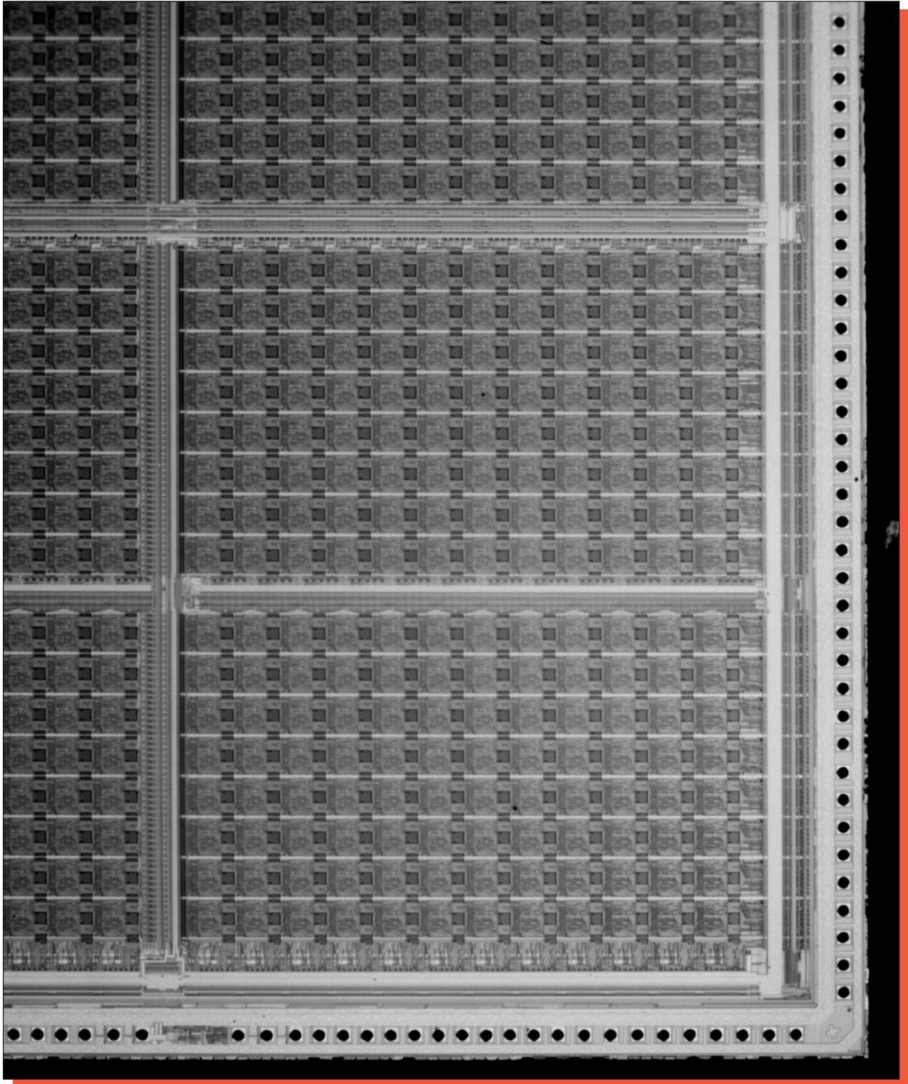
Figure 1b. Portion of the QuickLogic 24X32 intact circuit die. Mag. 26x.
