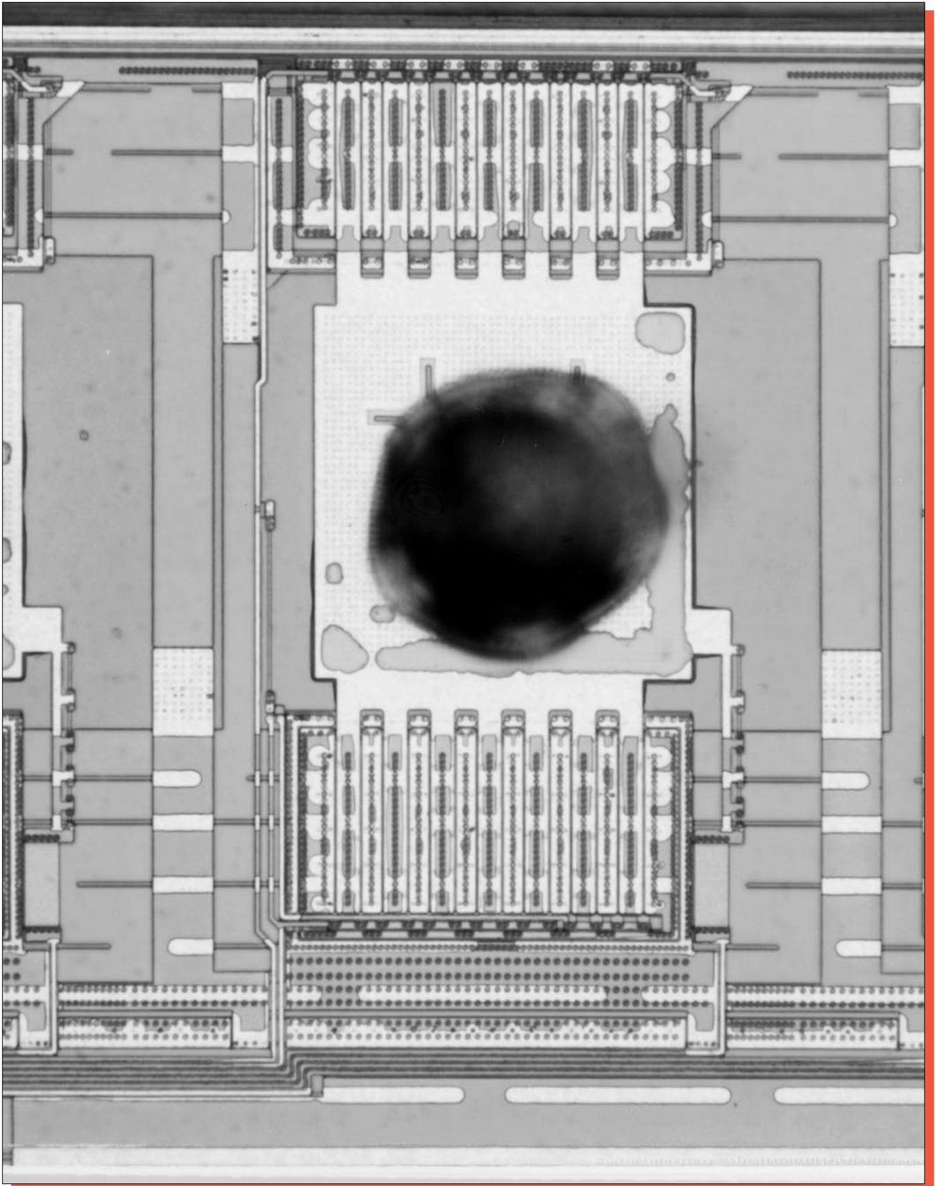
Figure 26. Optical view of the I/O layout. Metal 1, Mag. 640x.
