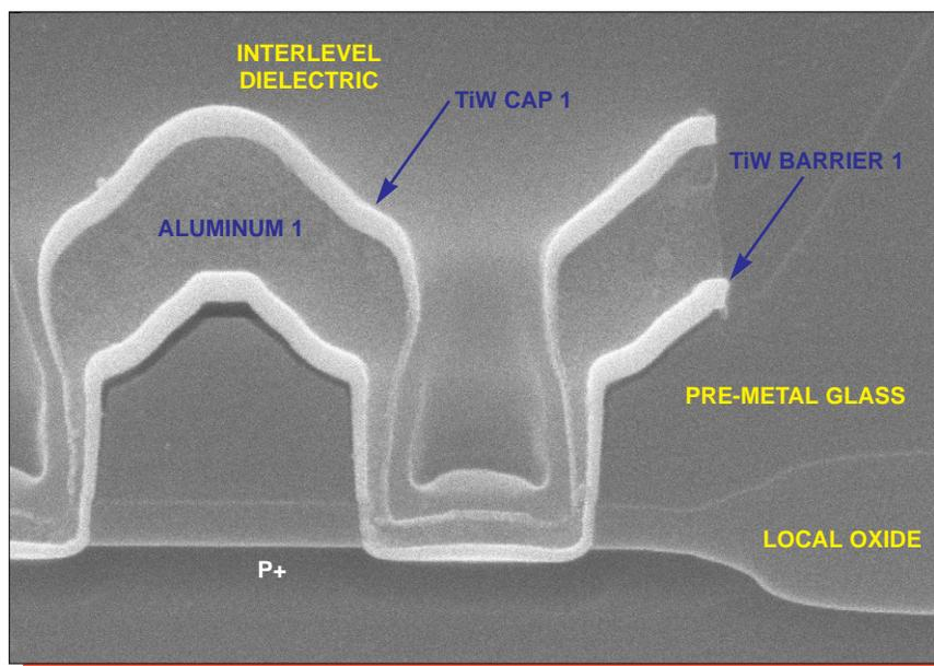
Figure 14. SEM section views of metal 1-to-diffusion contacts. Mag. 26,000x.
