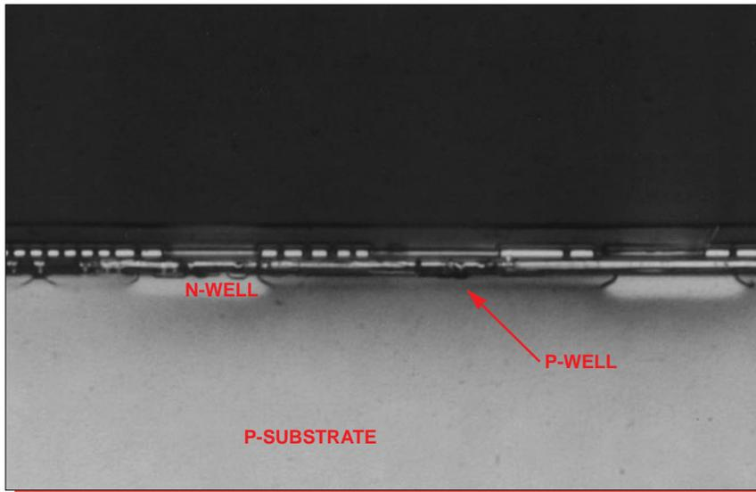
Figure 19. Optical view of the well structure. Mag. 800x.
