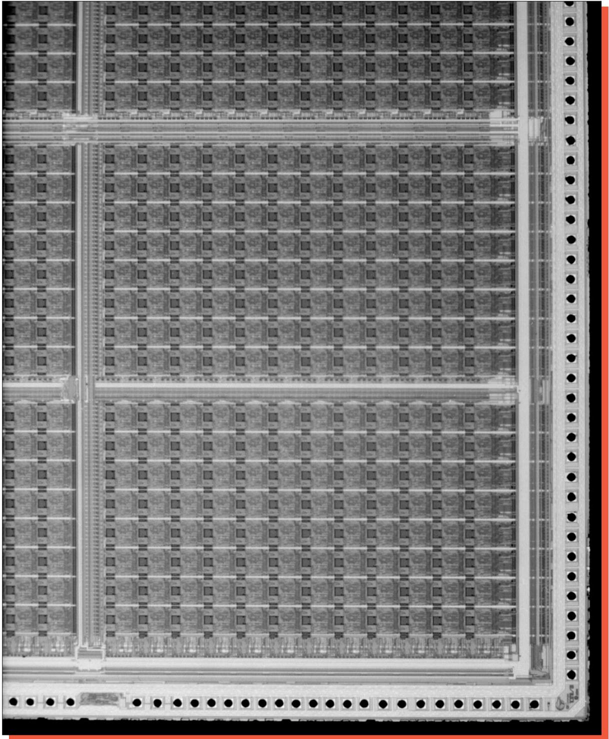
Figure 1a. Portion of the QuickLogic 24X32 intact circuit die. Mag. 26x.
