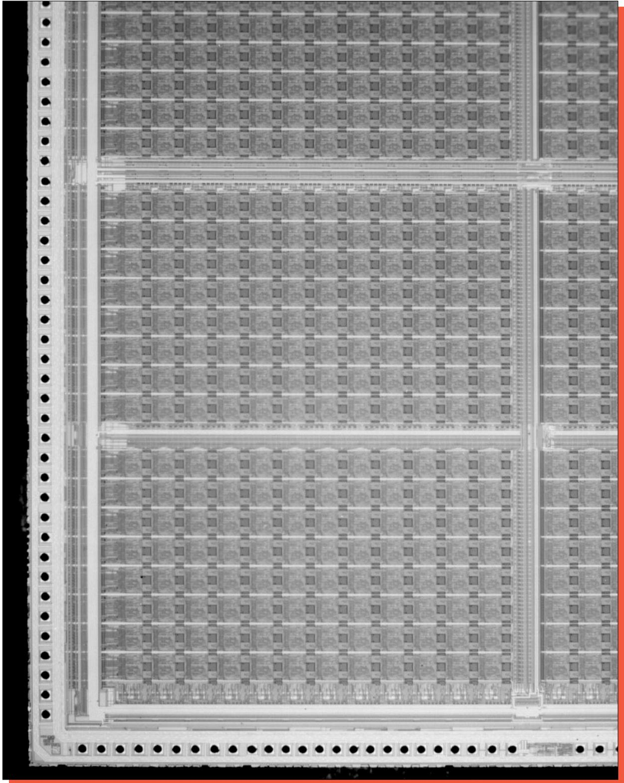
Figure 1. Portion of the QuickLogic 24X32 intact circuit die. Mag. 26x.
