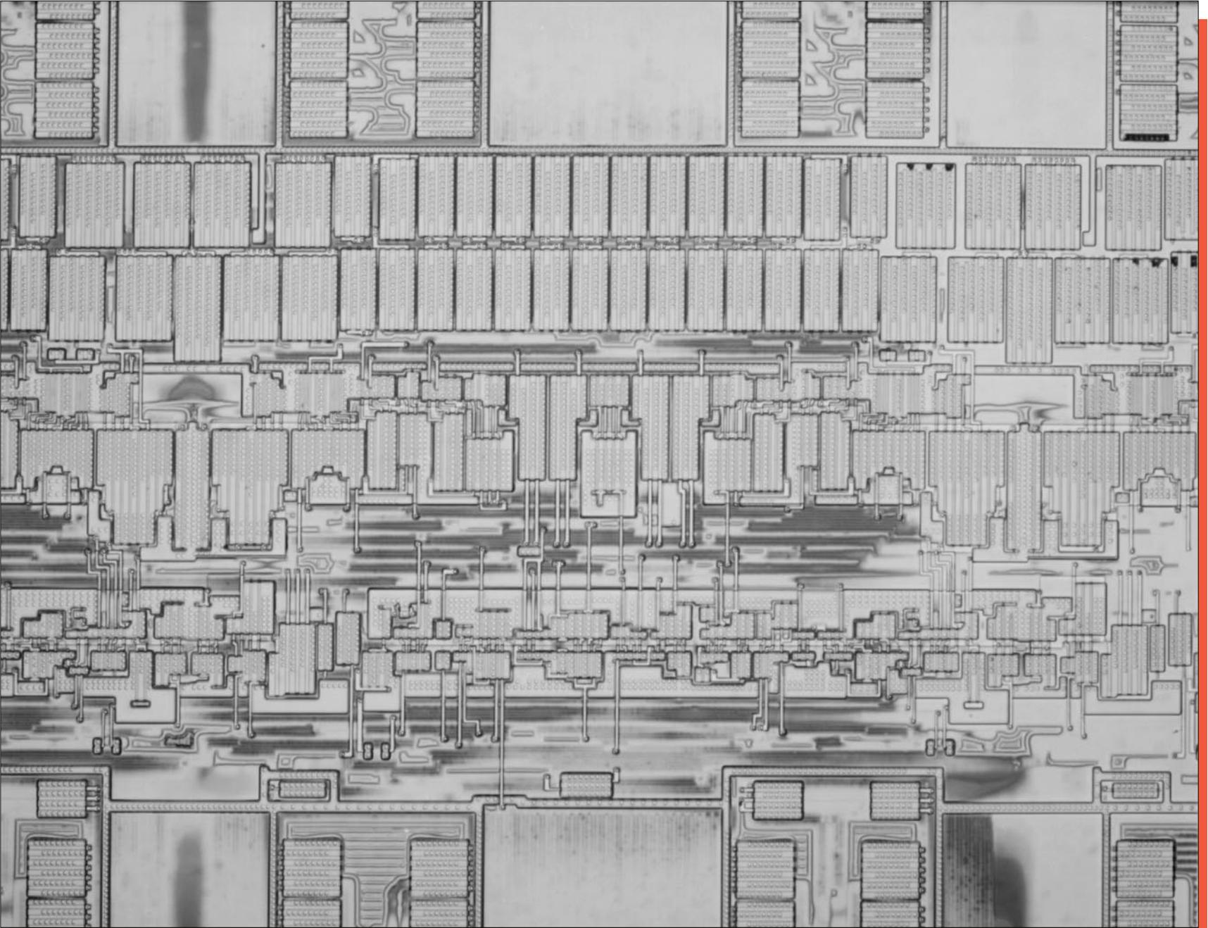
Figure 21b. Optical view of typical device circuitry. Poly, Mag. 520x.
