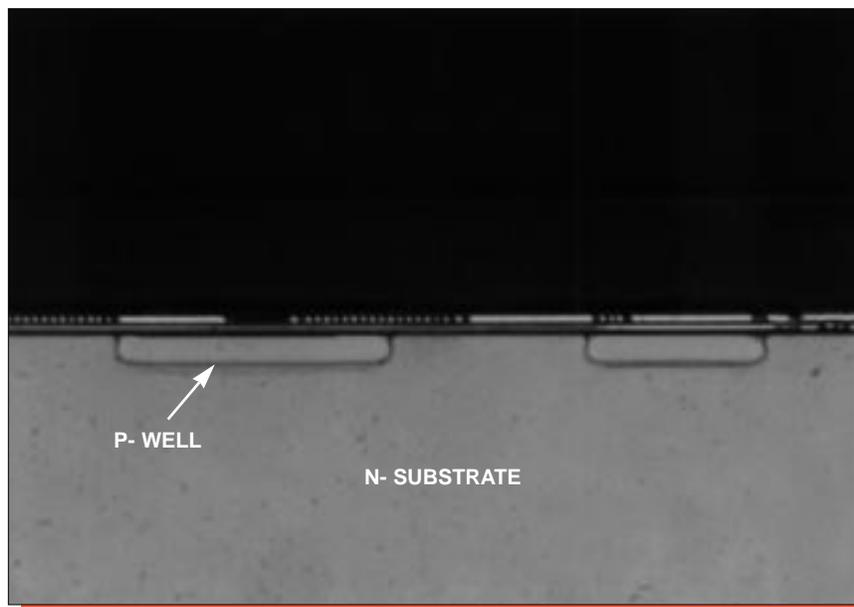
Figure 24. Optical section view of the well structure. Mag. 800x.
