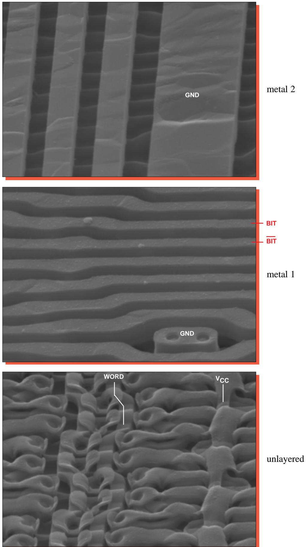
Figure 28. Perspective SEM views of a SRAM cell array. Mag. 13,000x, 60°.
