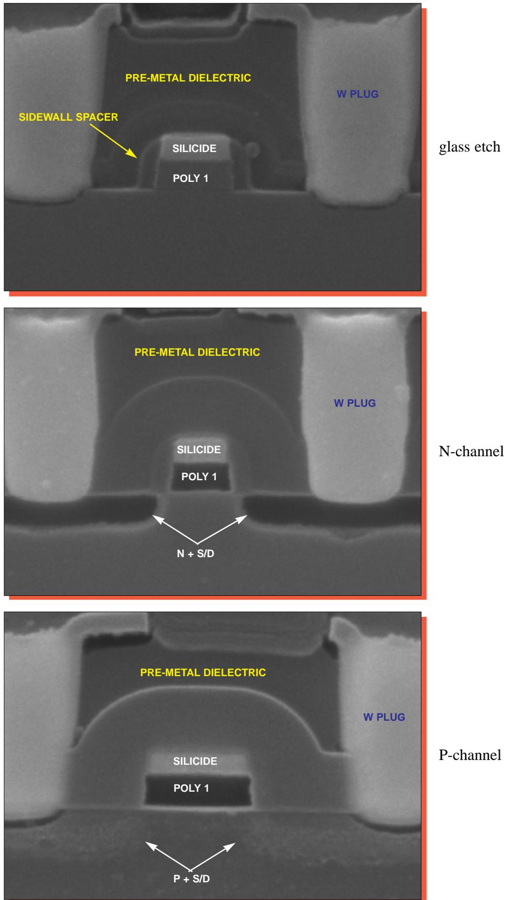
Figure 22. SEM section views of typical transistors. Mag. 52,000x.
