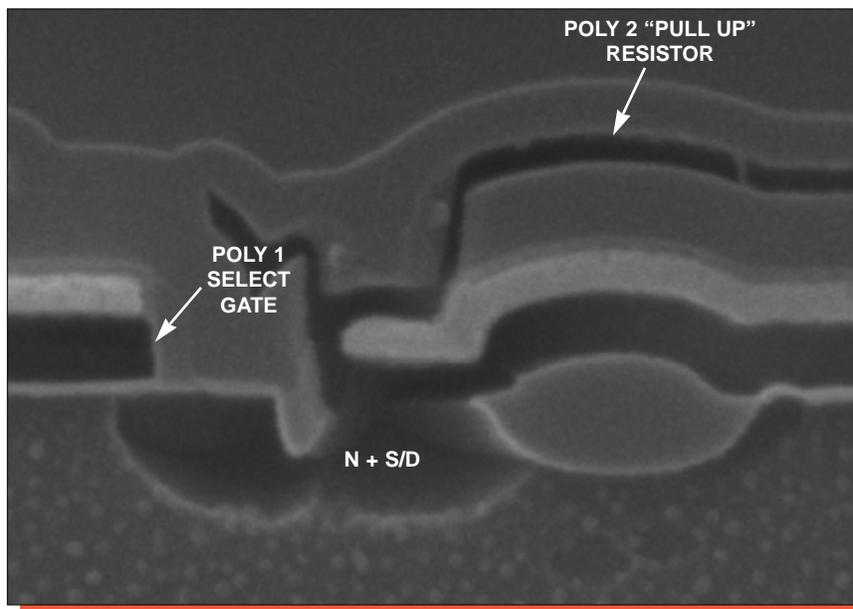
Figure 34. Detailed SEM views of SRAM cell array. Mag. 52,000x.
