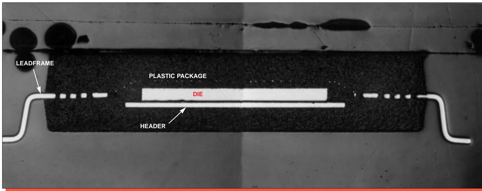
Figure 3. Package section view of general construction Mag. 13x.
