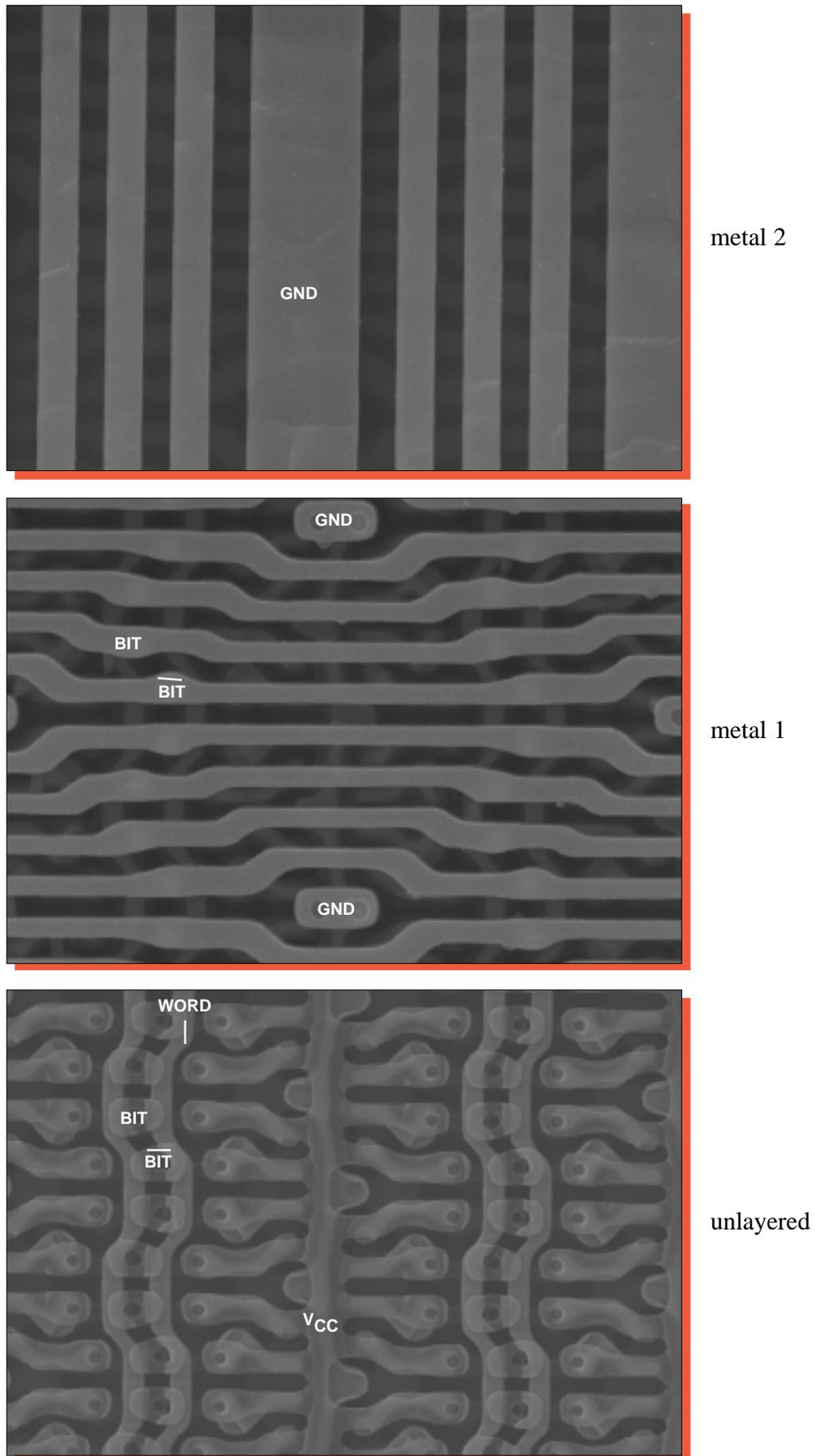
Figure 30. Topological SEM views of the SRAM cell array. Mag. 6500x.
