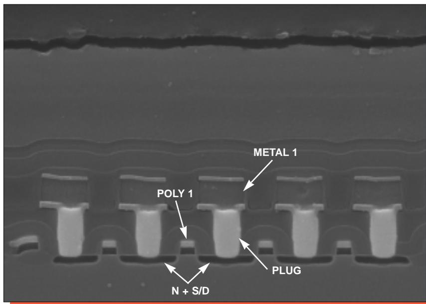
Figure 9. SEM section views illustrating general structure. Mag. 13,000x.
