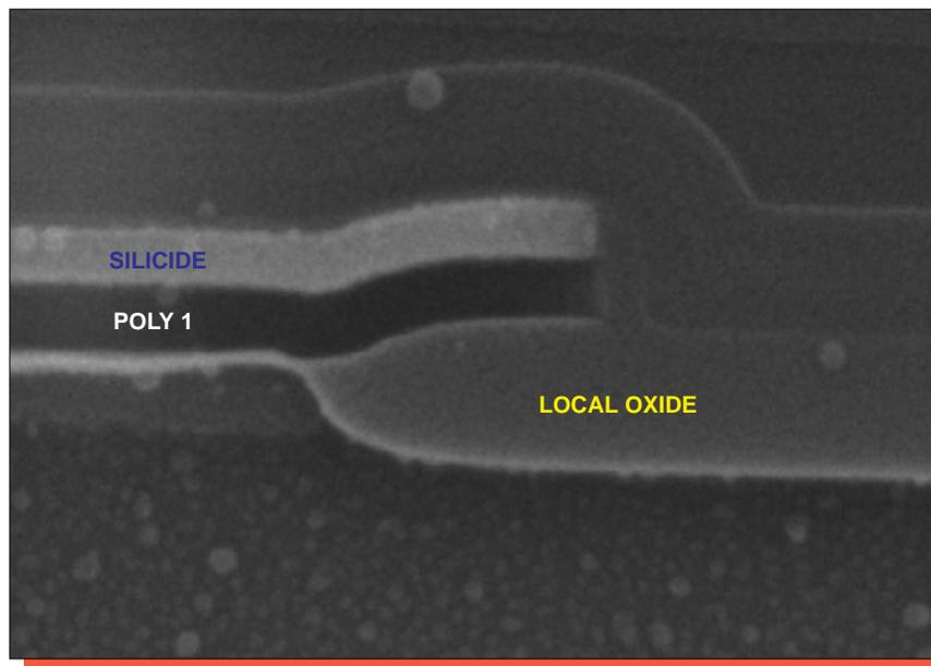
Figure 23. SEM section view of a typical local oxide birdsbeak. Mag. 52,000x.
