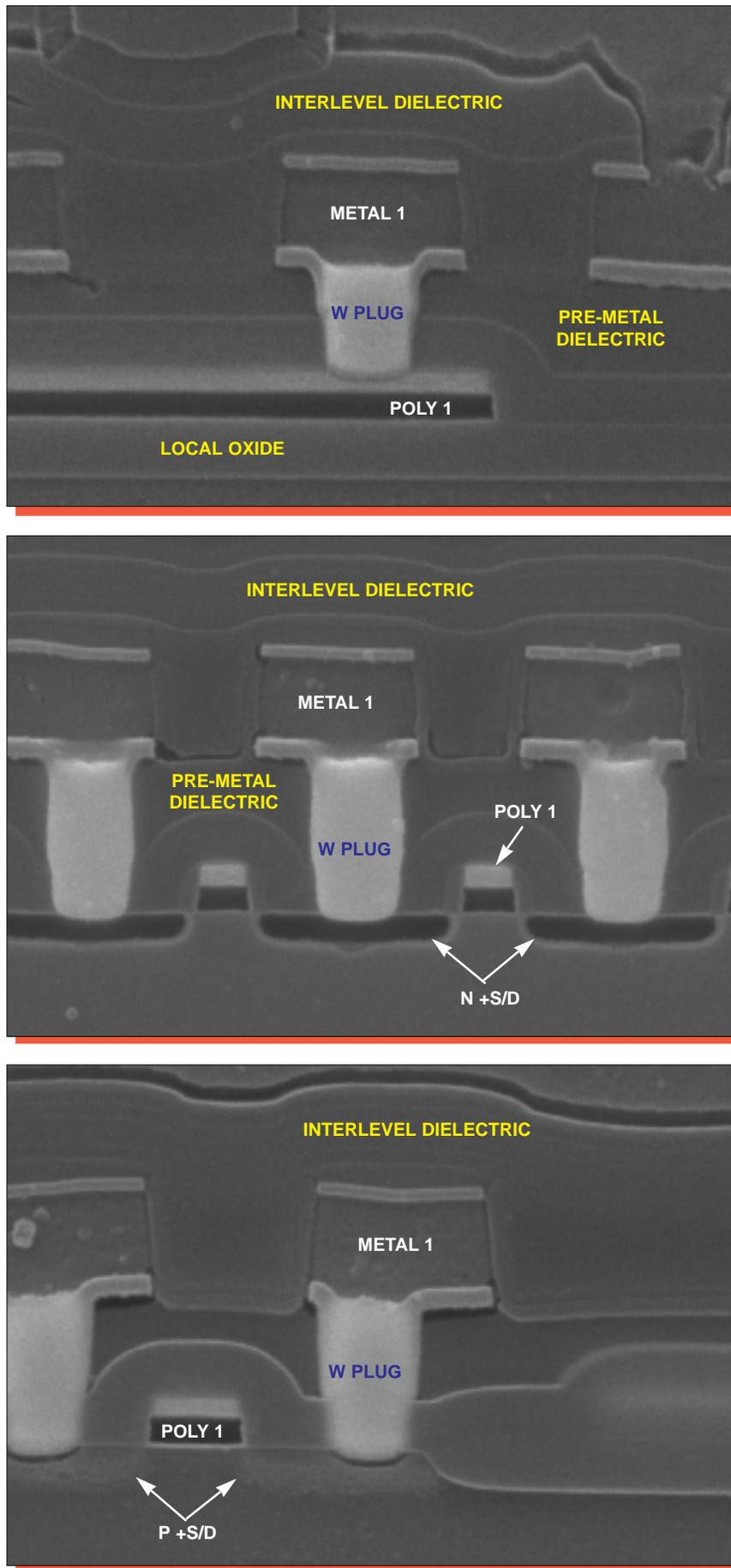
Figure 19. SEM section views of metal 1 contacts. Silicon etch, Mag. 26,000x.
