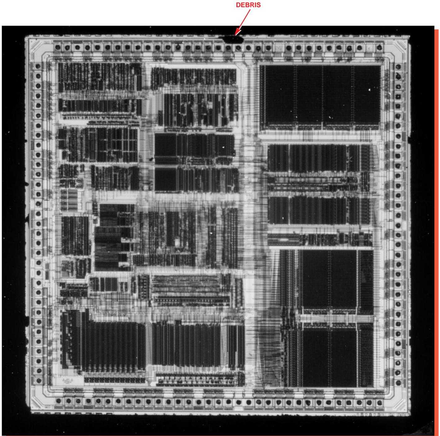
Figure 10. Whole die photograph of the Motorola XC56002PV80. Mag. 26x.
