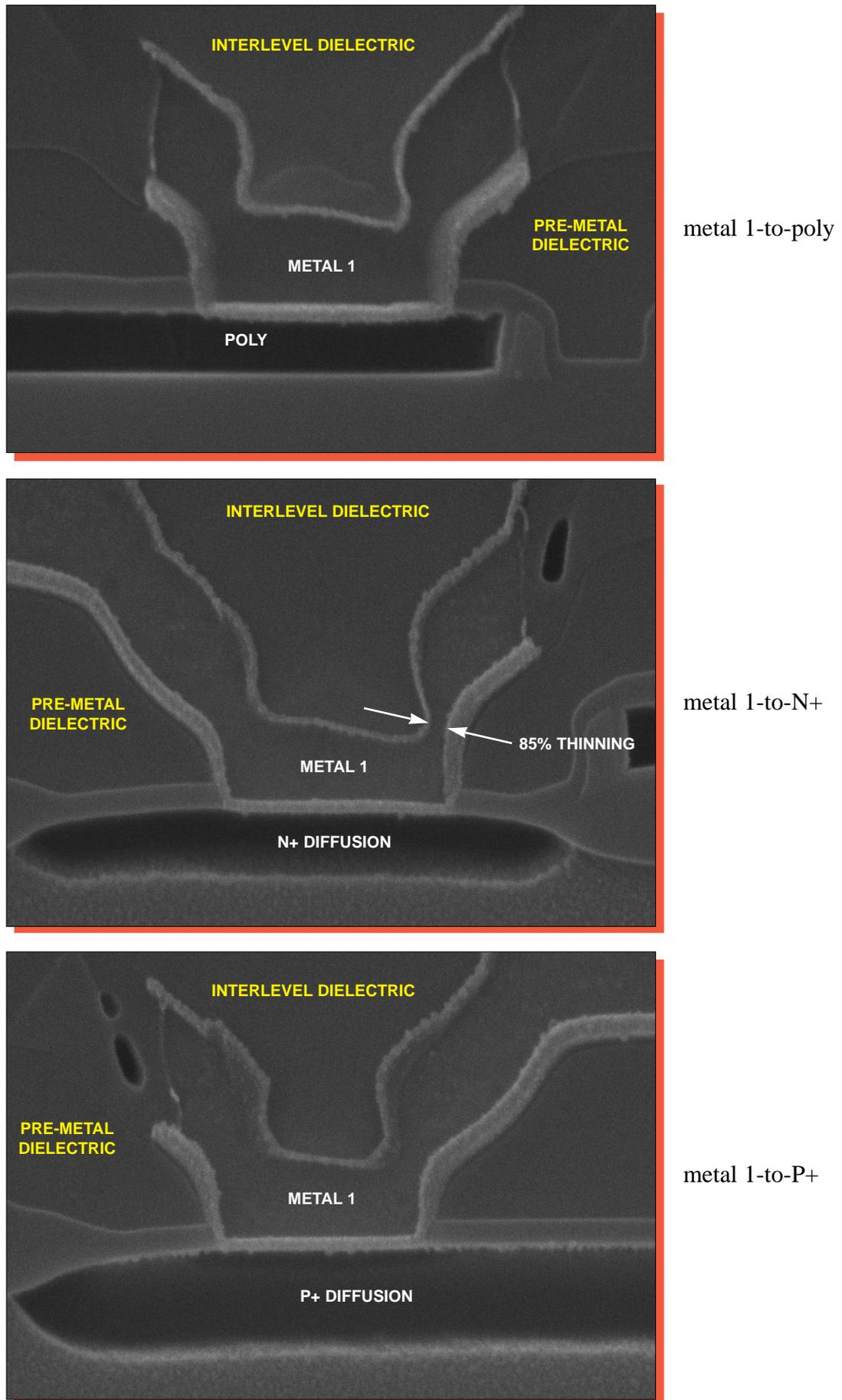
Figure 23. SEM section views of metal 1 contacts (silicon etch). Mag. 40,000x.
