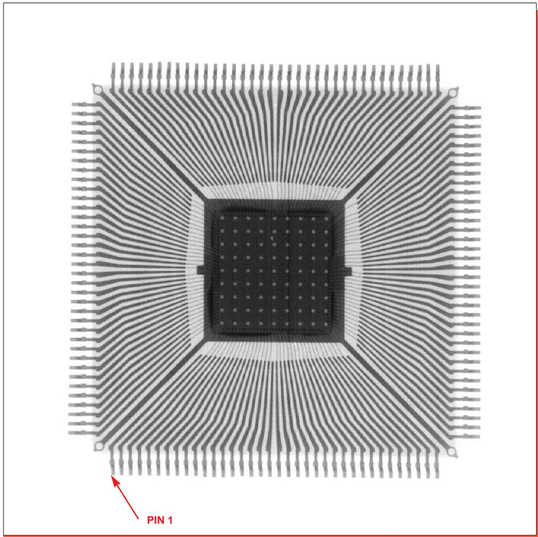
Figure 2. X-ray view of the package. Mag. 5x.
