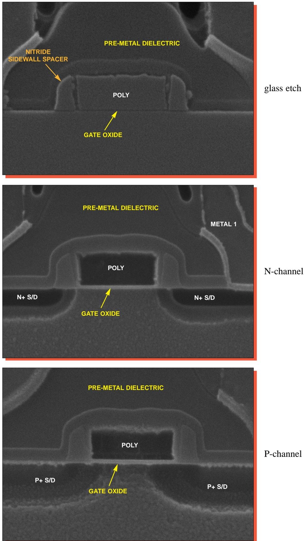
Figure 26. SEM section views of typical transistors. Mag. 52,000x.
