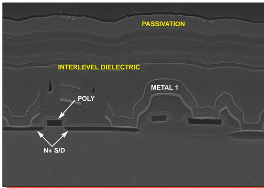
Figure 14. SEM section views illustrating general device structure. Mag. 10,000x.
