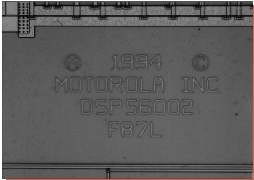
Figure 11. Optical view of marking on the die surface. Mag. 400x.
