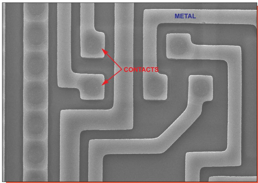
Figure 13. Topological SEM views of metal patterning. Mag. 1850x, 0°.
