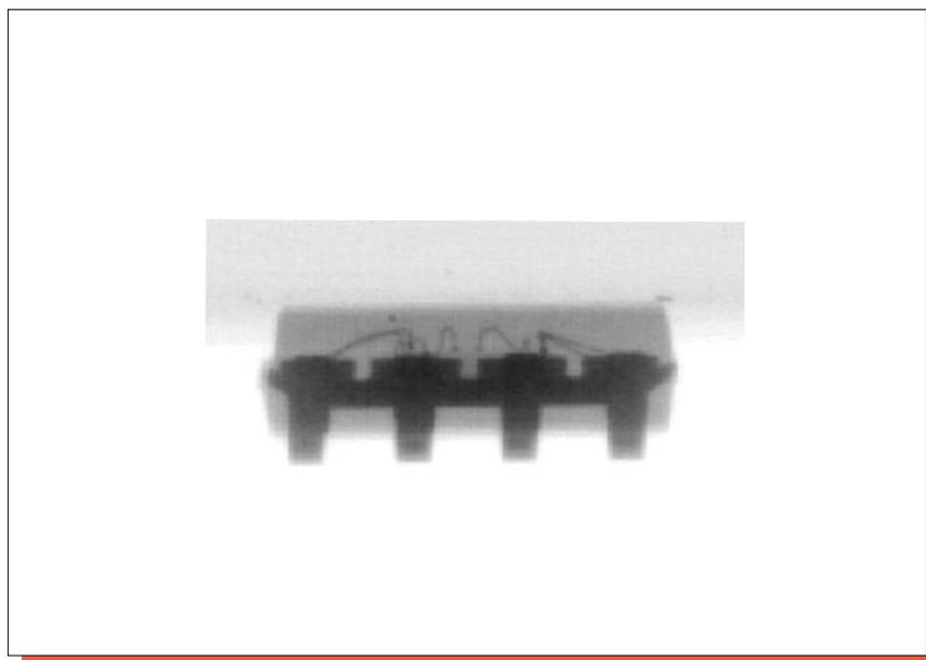
Figure 2. Topological and side x-ray views of the package. Mag. 10x.
