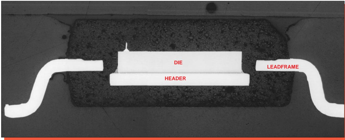
Figure 3. Section view of the package illustrating general package construction. Mag. 30x.
