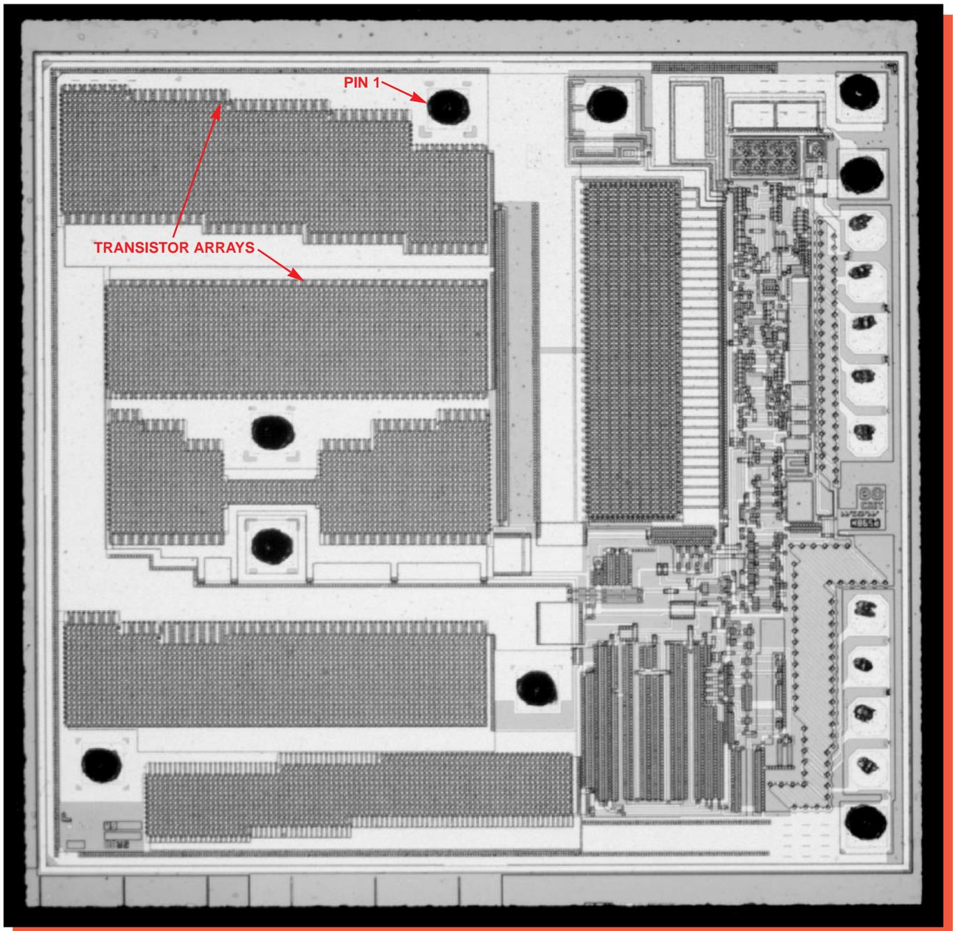
Figure 8. Whole die photograph of the Maxim MAX662 device. Mag. 76x.
