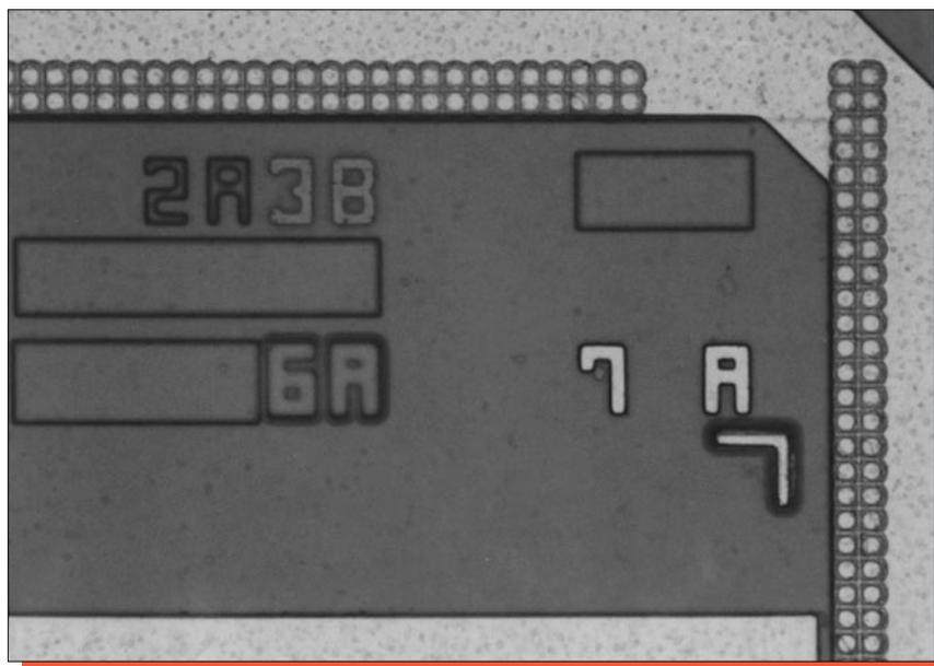
Figure 9. Die identification markings. Mag. 500x.
