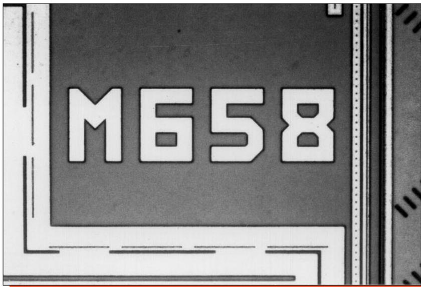
Figure 5. Identification markings from the die surface. Mag. 400x.
