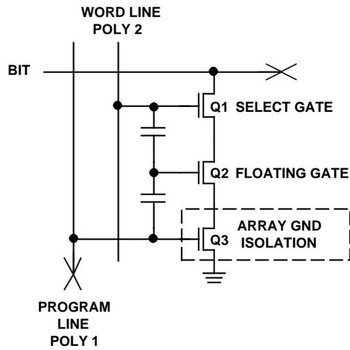
Figure 27b. Detailed topological view and schematic of an EEPROM cell.
