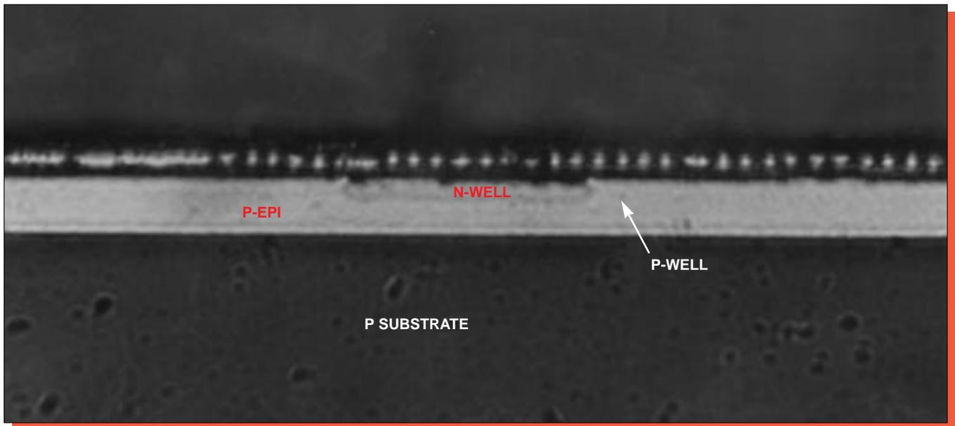
Figure 25a. Optical section view of well and epi layers. Mag. 1000x.
