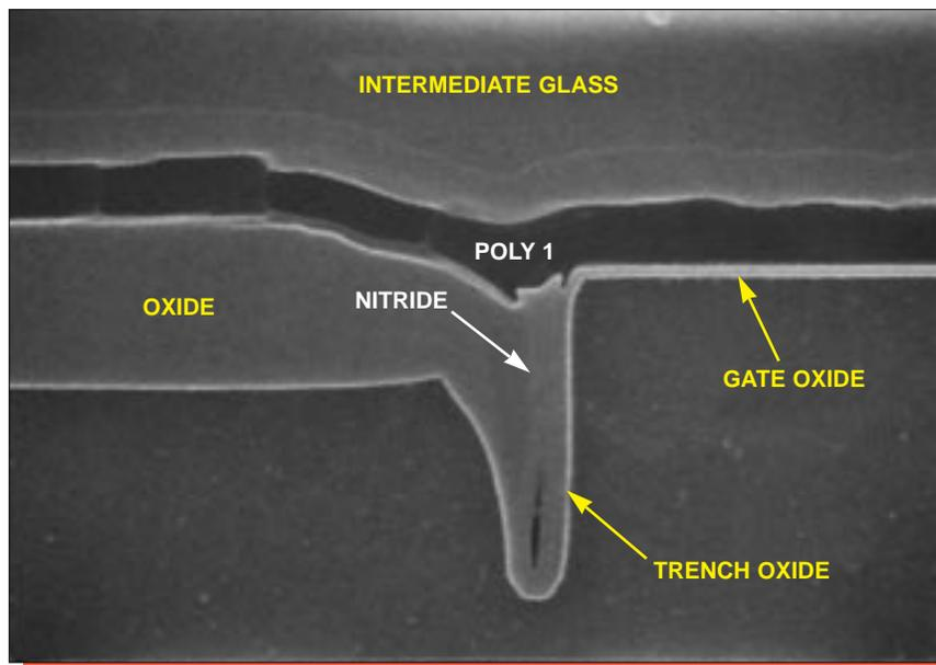
Figure 25b. SEM section view illustrating isolation. Mag. 30,000x.
