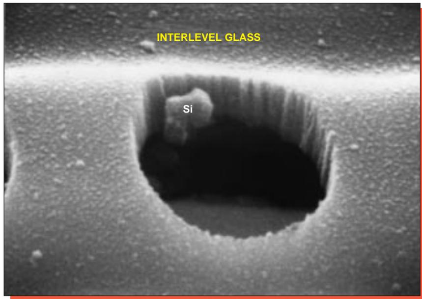
Figure 17. Perspective SEM view of via cut in oxide. Mag. 30,000x, 60°.
