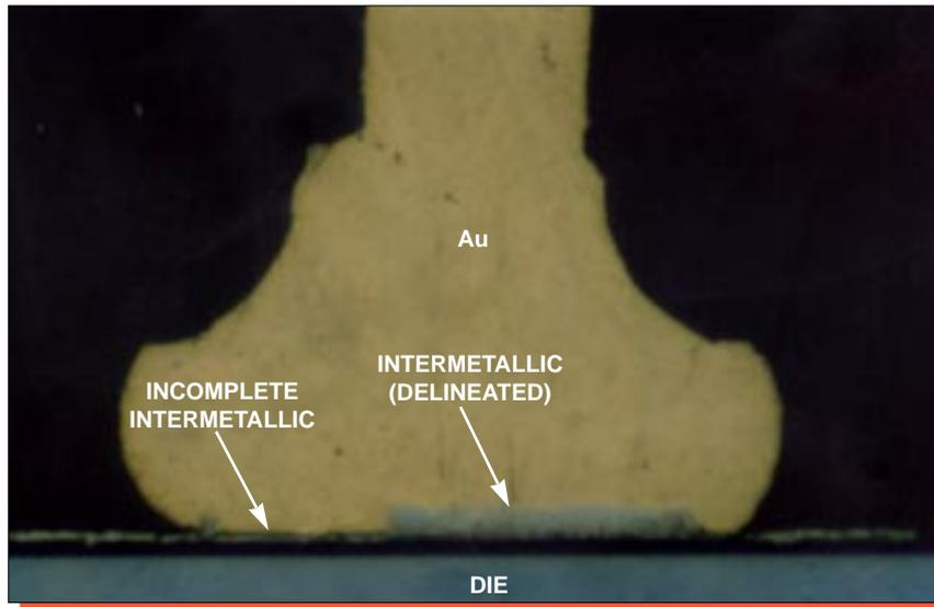
Figure 8. Optical view of a typical ball bond. Etched, Mag. 800x.
