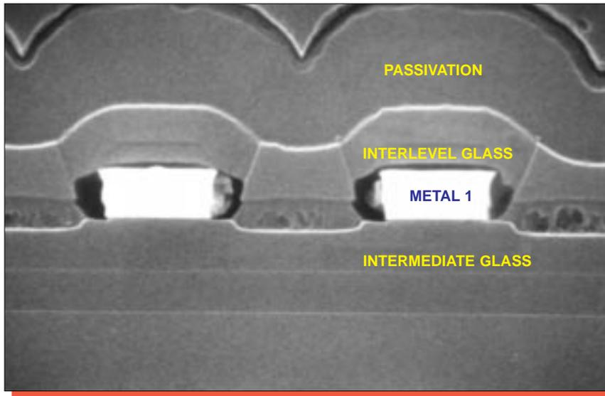
Figure 19. SEM section view of metal 1 line profiles. Mag. 14,000x.
