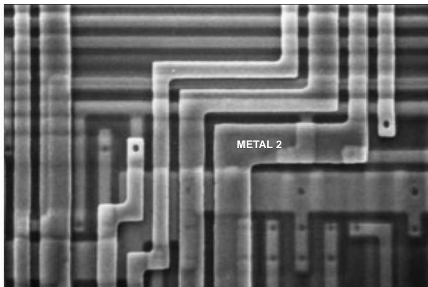
Figure 15. Topological SEM views of metal 2 patterning. Mag. 1500x.
