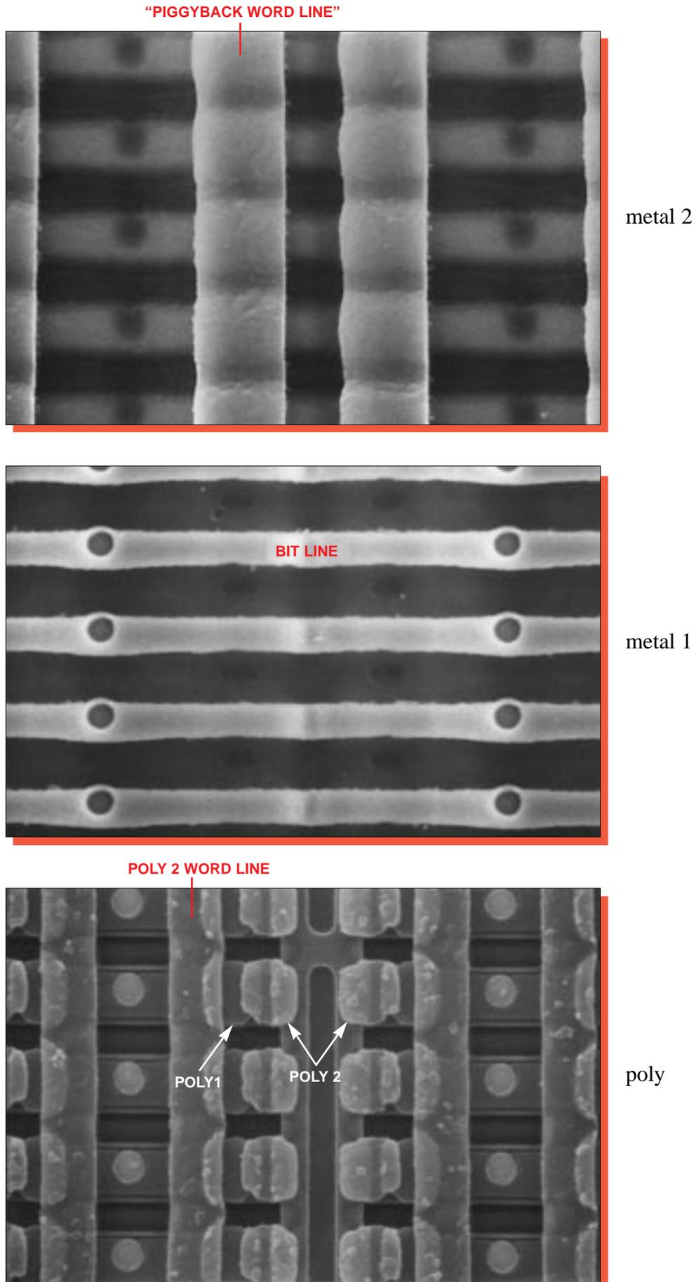
Figure 27. Topological SEM views of EEPROM cell array. Mag. 5000x, 0°.
