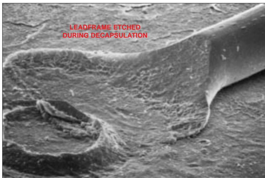
Figure 9. Perspective SEM views of typical wirebonds. Mag. 800x, 60°.
