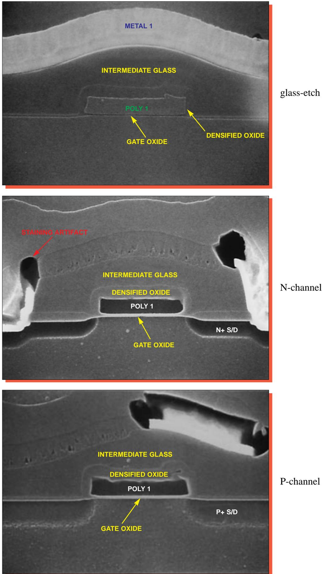
Figure 25. SEM section views of typical transistors. Mag. 25,000x.
