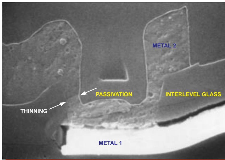
Figure 18. SEM section view of metal 2-to-metal 1 via. Mag. 25,000x.
