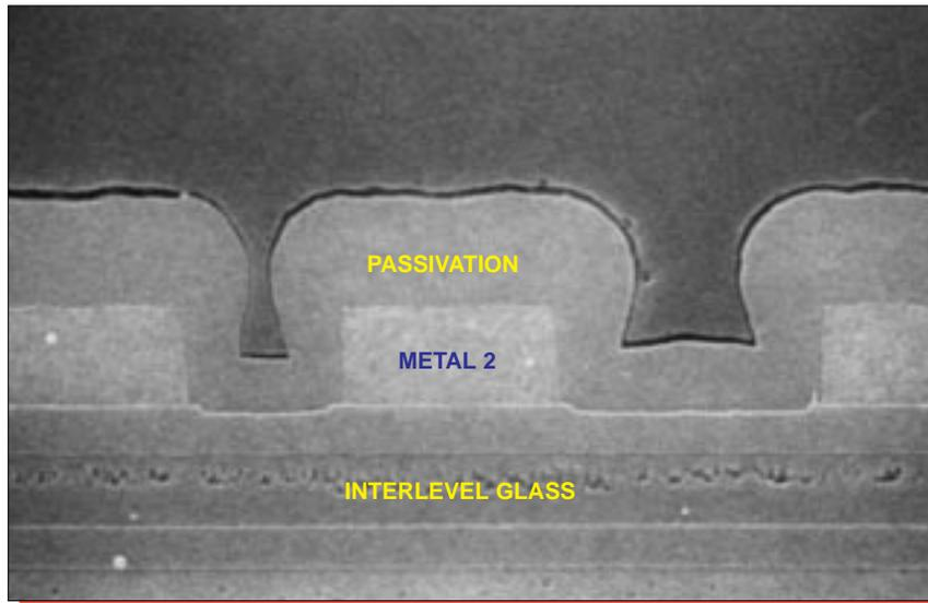
Figure 14. SEM section view of metal 2 line profile. Mag. 10,000x.
