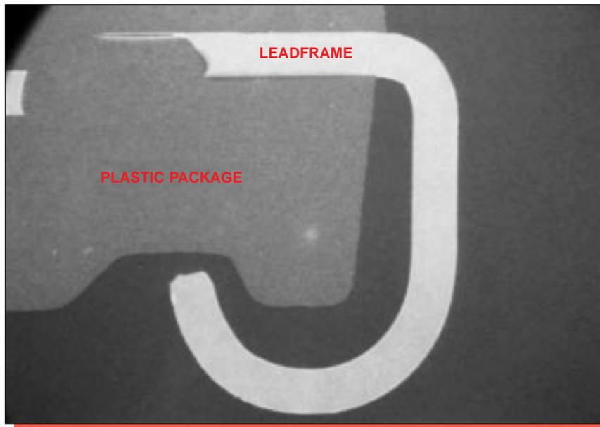
Figure 4. SEM section view of leadforming. Mag. 30x.
