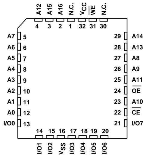
Figure 1. Package photograph and pinout of the Xicor X28C010J-20 128K x 8 EEPROM. Mag. 4x.
