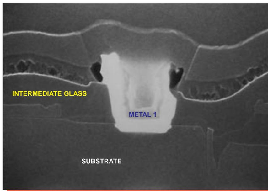
Figure 22. Glass etch SEM section views of typical metal 1 contacts. Mag. 20,000x.
