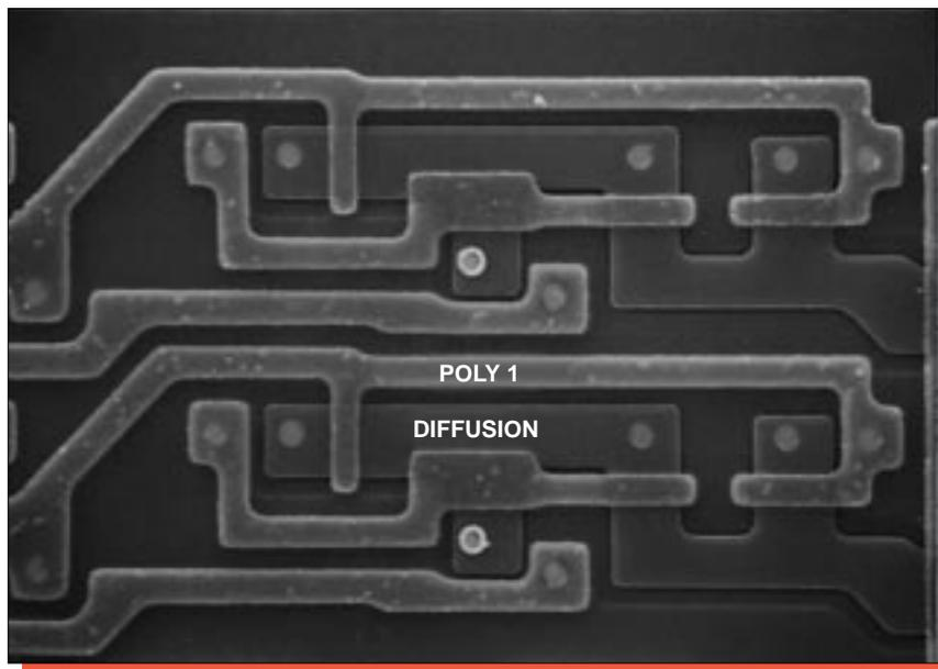
Figure 23. Topological SEM views of poly 1 patterning. Mag. 2500x.
