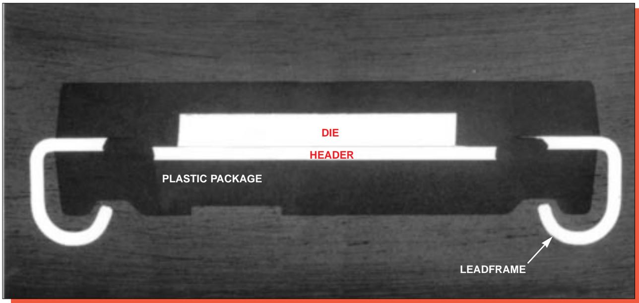
Figure 3. Optical section view of the package. Mag. 13x.
