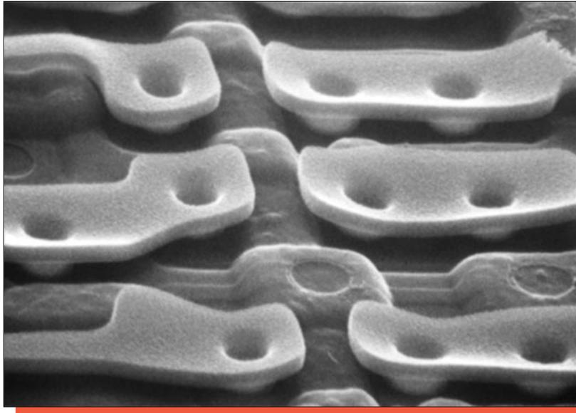
Figure 24. SEM view of general polycide coverage. Mag. 15,000x, 60°.
