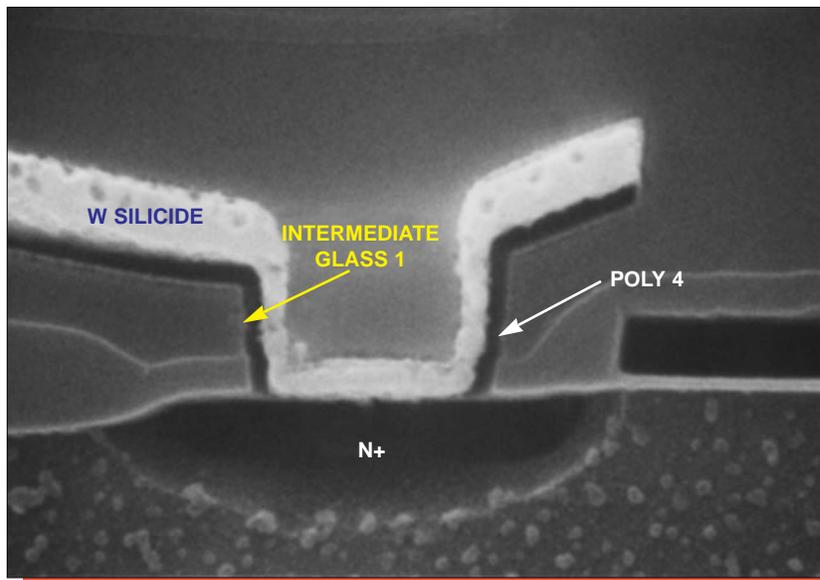
Figure 25. SEM section view of a polycide-to-N+ contact. Mag. 50,000x.
