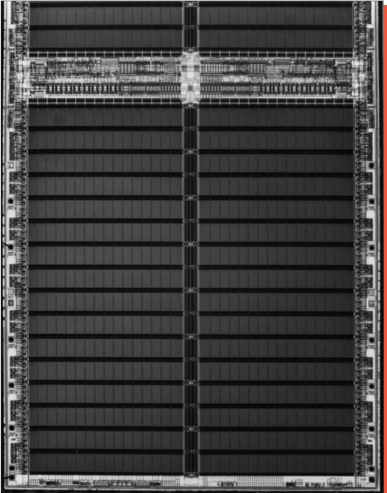
Figure 8a. Remaining portion of the Samsung KM44C4000 die photograph. Mag. 30x.
