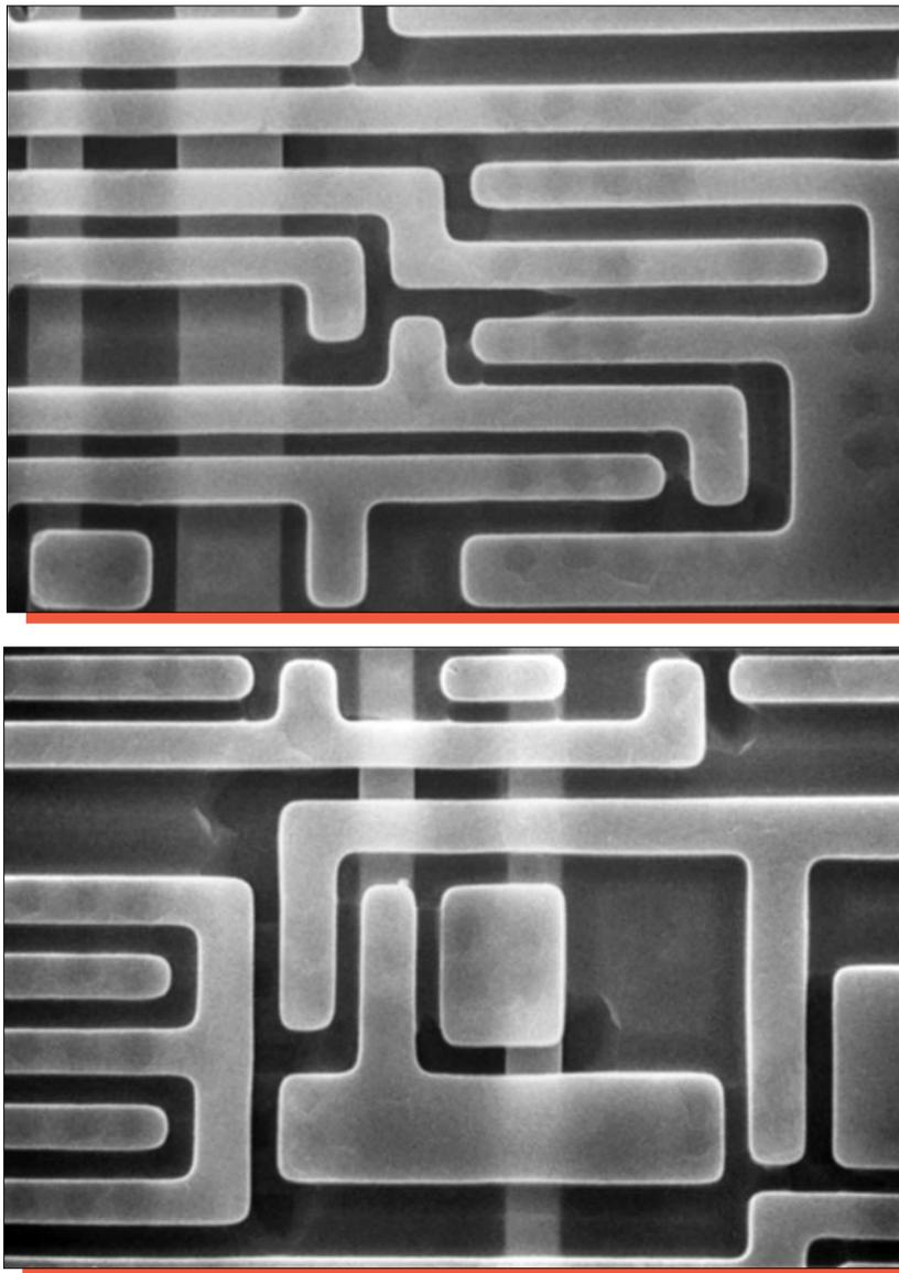
Figure 19. Topological SEM views of metal 1 patterning. Mag. 4000x, 0°.
