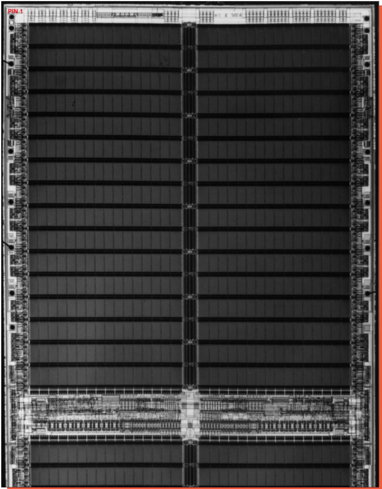
Figure 8. Portion of the Samsung KM44C4000 die photograph. Mag. 30x.
