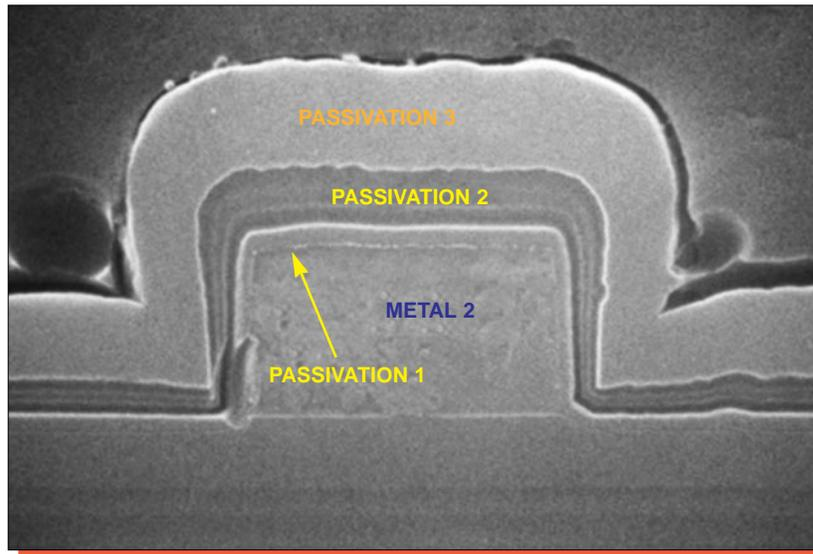
Figure 12. SEM section view of a metal 2 line profile. Mag. 25,000x.
