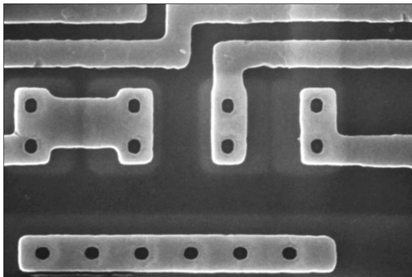
Figure 13. Topological SEM views of metal 2 patterning. Mag. 3500x, 0°.
