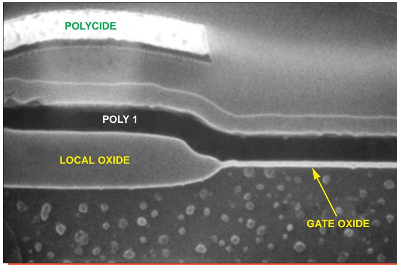
Figure 30. SEM section view of a local oxide birdsbeak. Mag. 50,000x.
