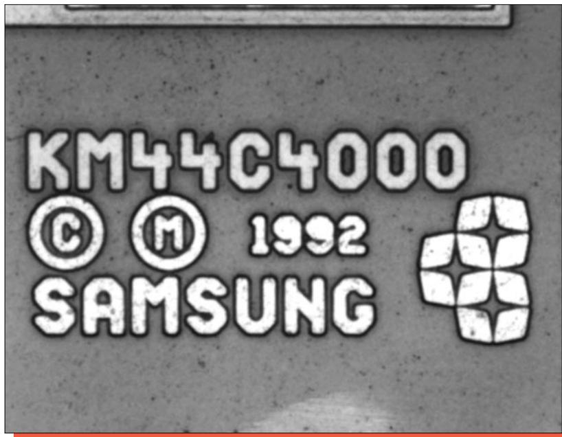
Figure 9. Die identification markings. Mag. 800x.
