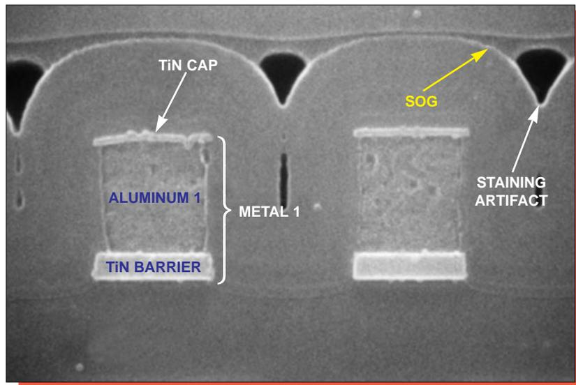
Figure 18. SEM section view of metal 1 line profiles. Mag. 40,000x.
