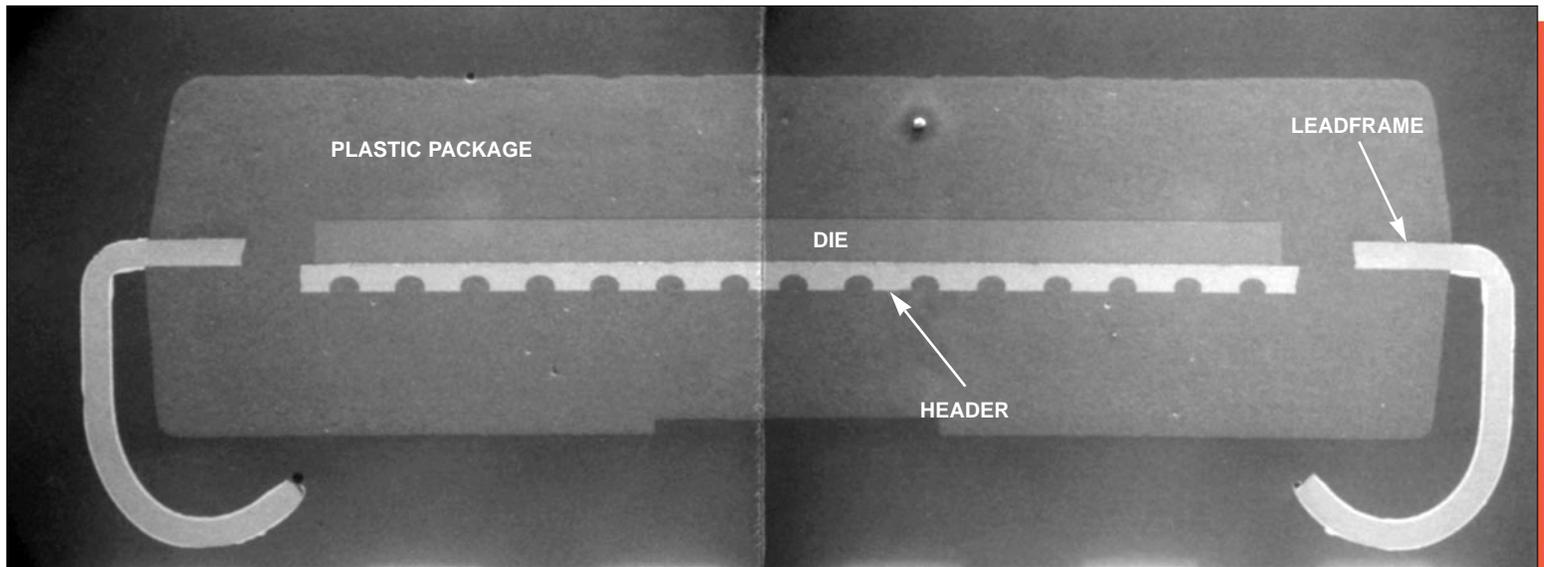
Figure 3. Section view of the package illustrating general construction. Mag. 17x.
