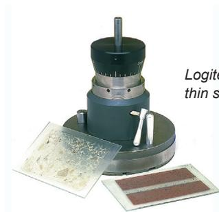
Logitech PLJ7 jig with thin section samples.
