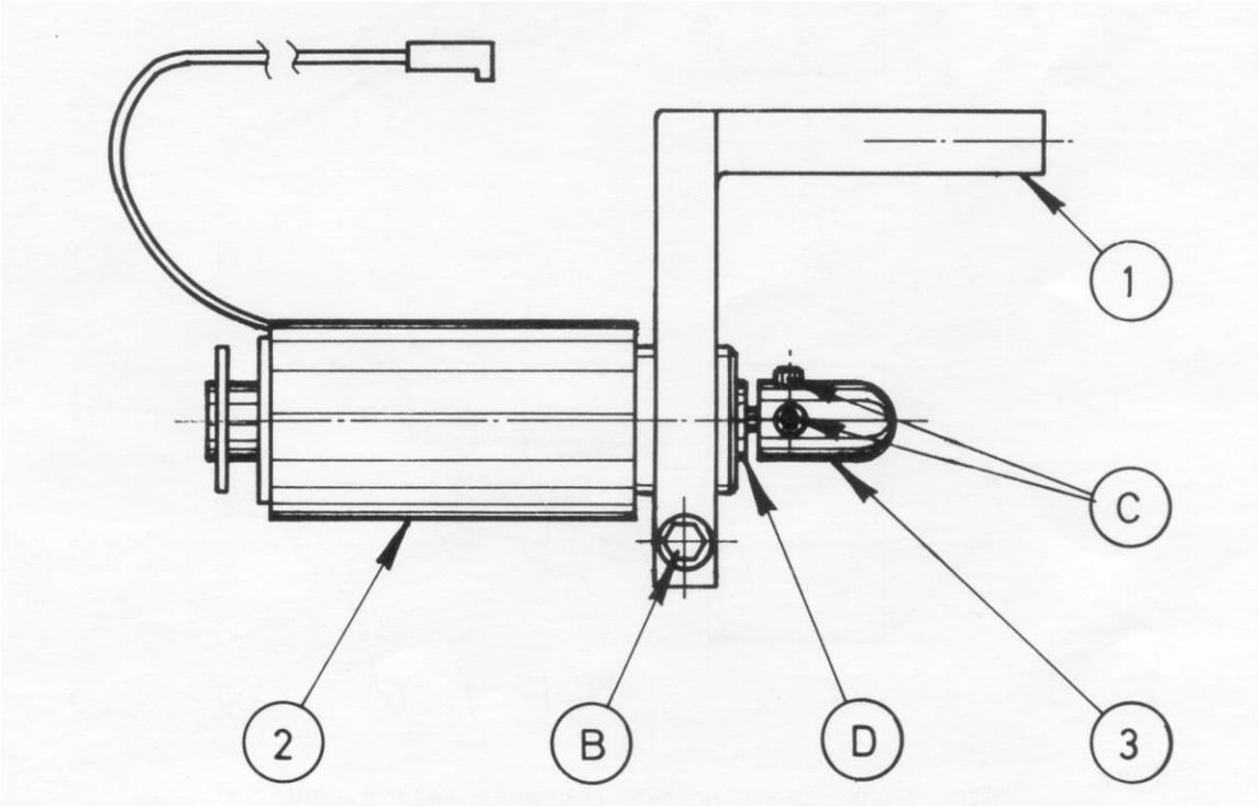
FIG. 10-8 EFO SOLENOID BRACKET ASSEMBLY (#4124-0451-0)
