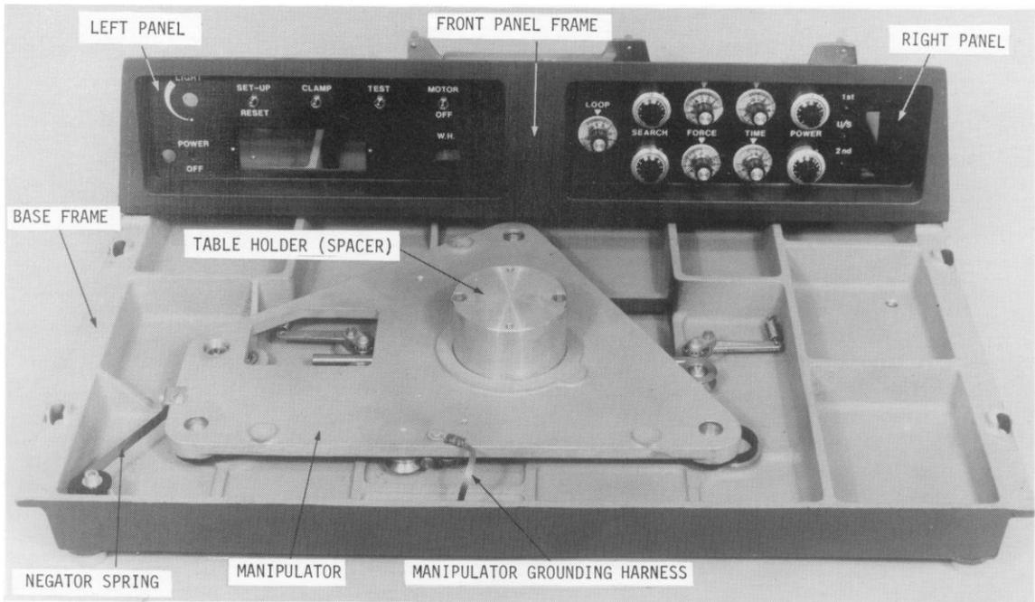
FIG. 3-3 MANIPULATOR ASSEMBLY AND WORKHOLDER TABLE SUSPENSION
