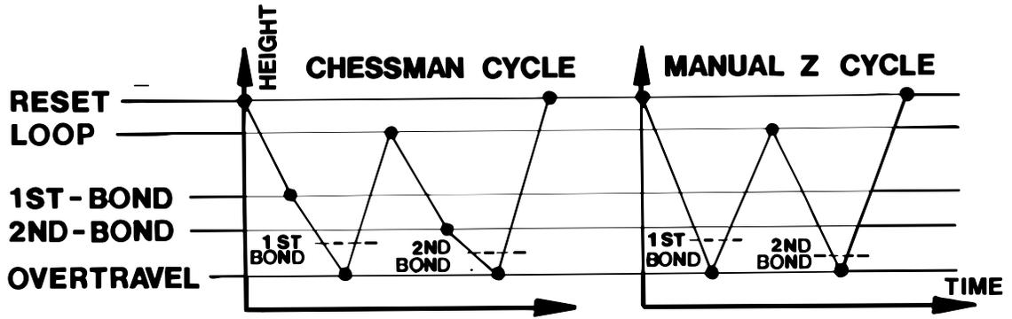
FIG. 3-7 BONDING HEAD PLACEMENTS
