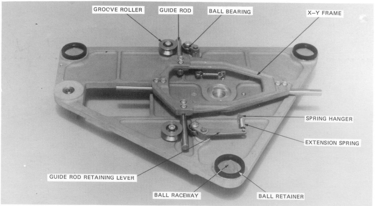
FIG. 3-5 MANIPULATOR UNDERSIDE AND X-Y FRAME
