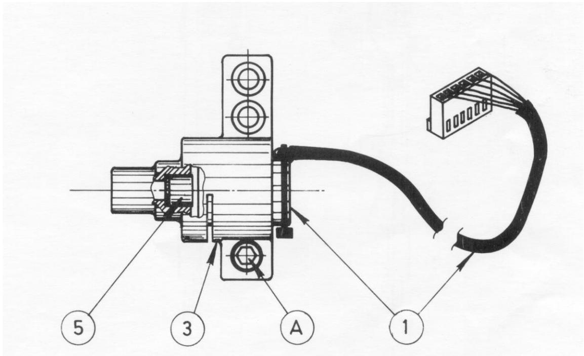
FIG. 10-8 MAIN/Z LVDT ASSEMBLY (#4123-0414-0)
