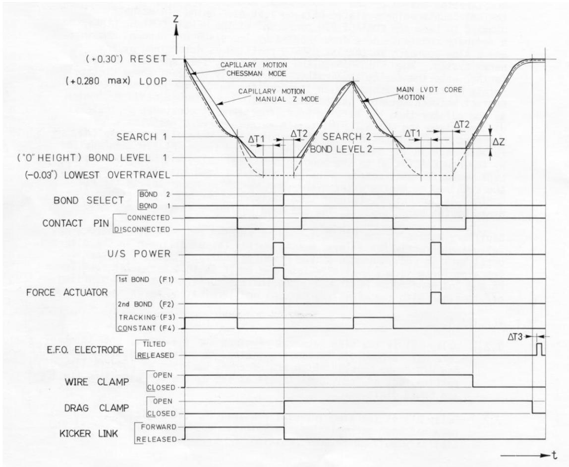
FIG. 7-1 BONDING CYCLE TIME STUDY
