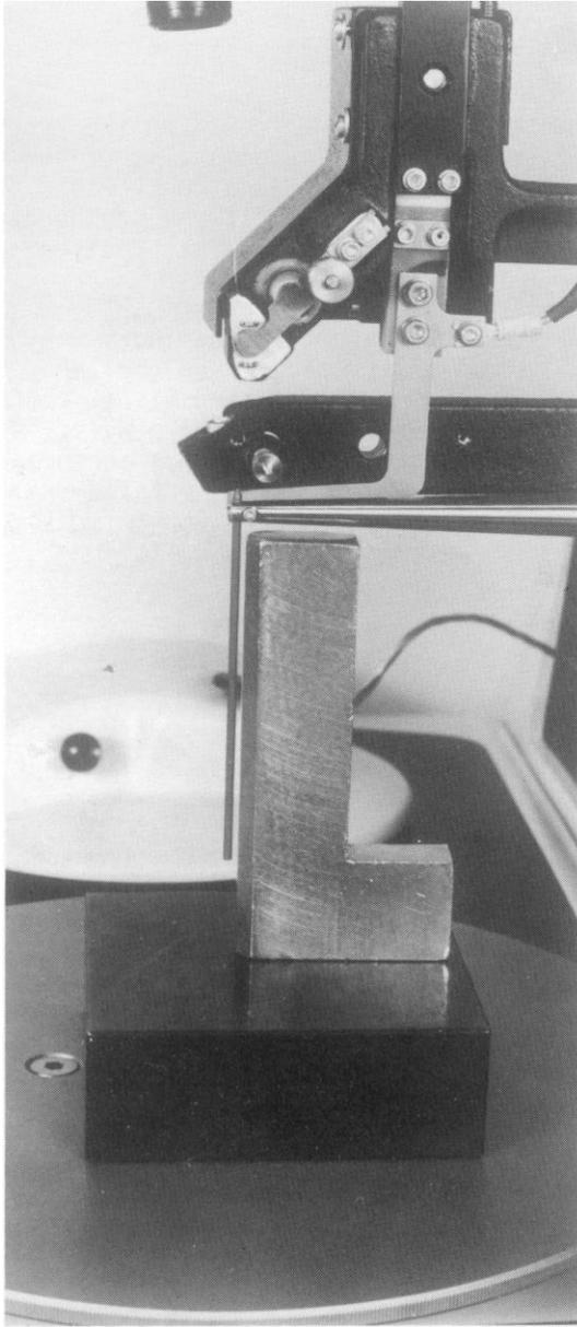
FIG. 6-1 TRANSDUCER INSERTION AND LEVELING ADJUSTMENTS
