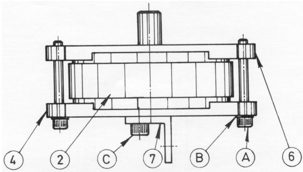
FIG. 10-4 FORCE ACTUATOR ASSEMBLY (#4123-0413-0)
