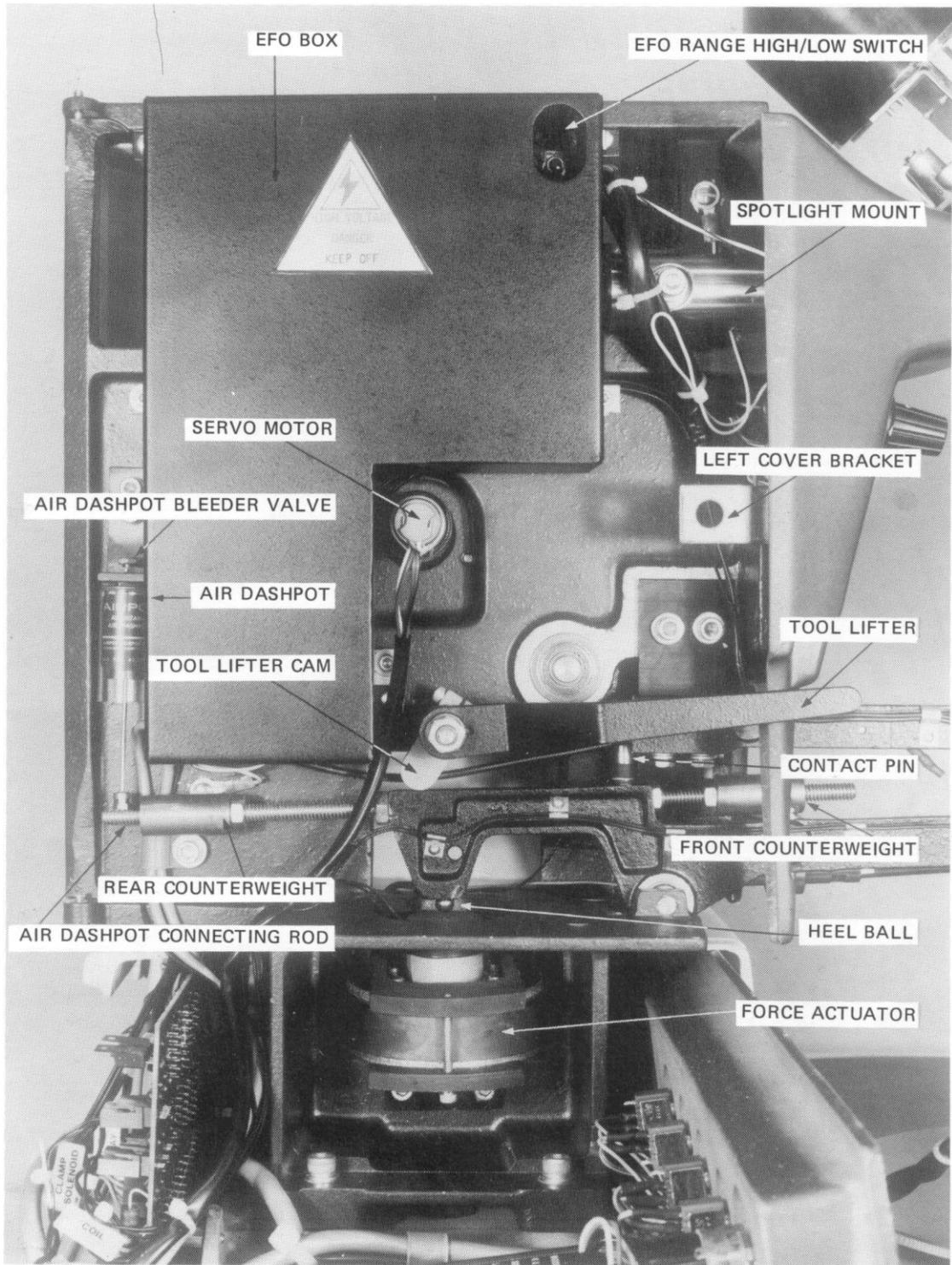
FIG. 3-9 MAIN HEAD - INNER LEFT SIDE
