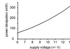
The power dissipation of the CR-113 is shown to the left as a function of supply voltage. The minimum supply voltage for good operation is +/- 6V. Any supply voltage applied in excess of this figure does not change or improve CR-113 performance, but instead results in unnecessary power dissipation.
