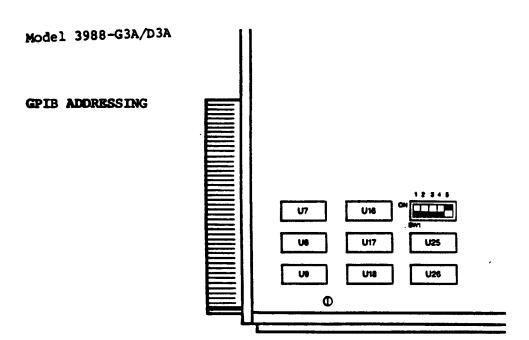
The GPIB address switch (SW1) is located on the component side of the module near the lower left corner
