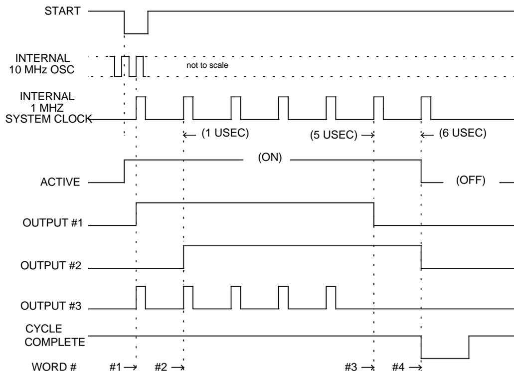
To repeat the sequence may require an enable output F(26)·A(1) and an appropriate start.
