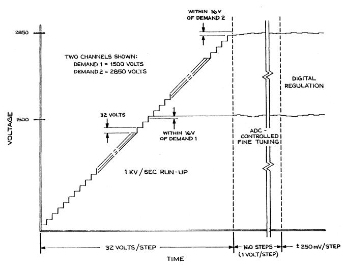
HV4032A: REPRESENTATION OF HIGH VOLTAGE RUN-UP FOR TWO 3.3KV CHANNELS
