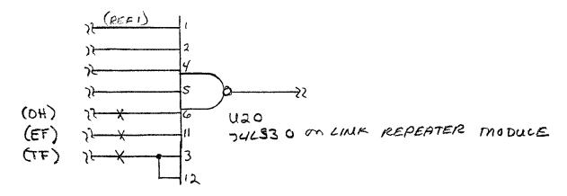
HOUSE AGGREGATE CODE DIETECTOR, U20, ON LINK REPEATER THODUCE IS DIAGRAMMED TO Show which inputs must be isocated to provide SUBAGGREGATE HOUSE ADDRESSING.
