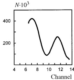
Fig. 5. Typical amplitude distribution obtained by irradiating a  $5 \times 5 \times 4$  mm  $\text{BaF}_2$  crystal, grown from a charge prepared in a platinum crucible from OSCH-7-5  $\text{BaCO}_3$ .
