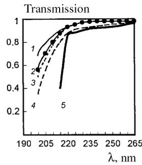
Fig. 4. Light transmission coefficient of  $\text{BaF}_2$  crystals versus wavelength for samples which are grown from a charge prepared in platinum (1, 3) and nickel (2, 4) crucibles, OSCH-7-5 and CH grade  $\text{BaCO}_3$ , respectively; 5) industrial sample.
