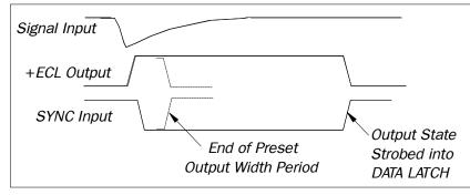
The state of the ECL outputs at the time the SYNC input occurs, are held for the duration of the SYNC input pulse. The output states are transferred into a DATA LATCH at the trailing edge of the SYNC input. The DATA LATCH can be read via CAMAC.
