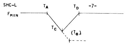
THIS CYCLE WILL BEGIN THE SAME, AT  $T_{\underline{A}}$ . However, before acceleration is complete, the unit will start to decelerate in order to end the cycle at the minimum frequency so  $T_{\underline{B}}$  is never achieved and at  $T_{\underline{C}}$  the down cycle is begun and the up cycle terminated.
