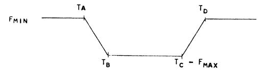
THIS TRAPAZOIDAL WAVESHAPE IS GENERATED BY USE OF AN OSCILLATOR, COUNTER AND DIGITAL TO ANALOG CONVERTER. THE ACCELERATION TIME,  $T_A-T_B$ , IS DETERMINED BY THE FREQUENCY OF THE ACCELERATION OSCILLATOR, IC 59, WHICH DETERMINES THE TIME IT WILL TAKE TO FILL THE EIGHT BIT COUNTER, (255 COUNTS).
